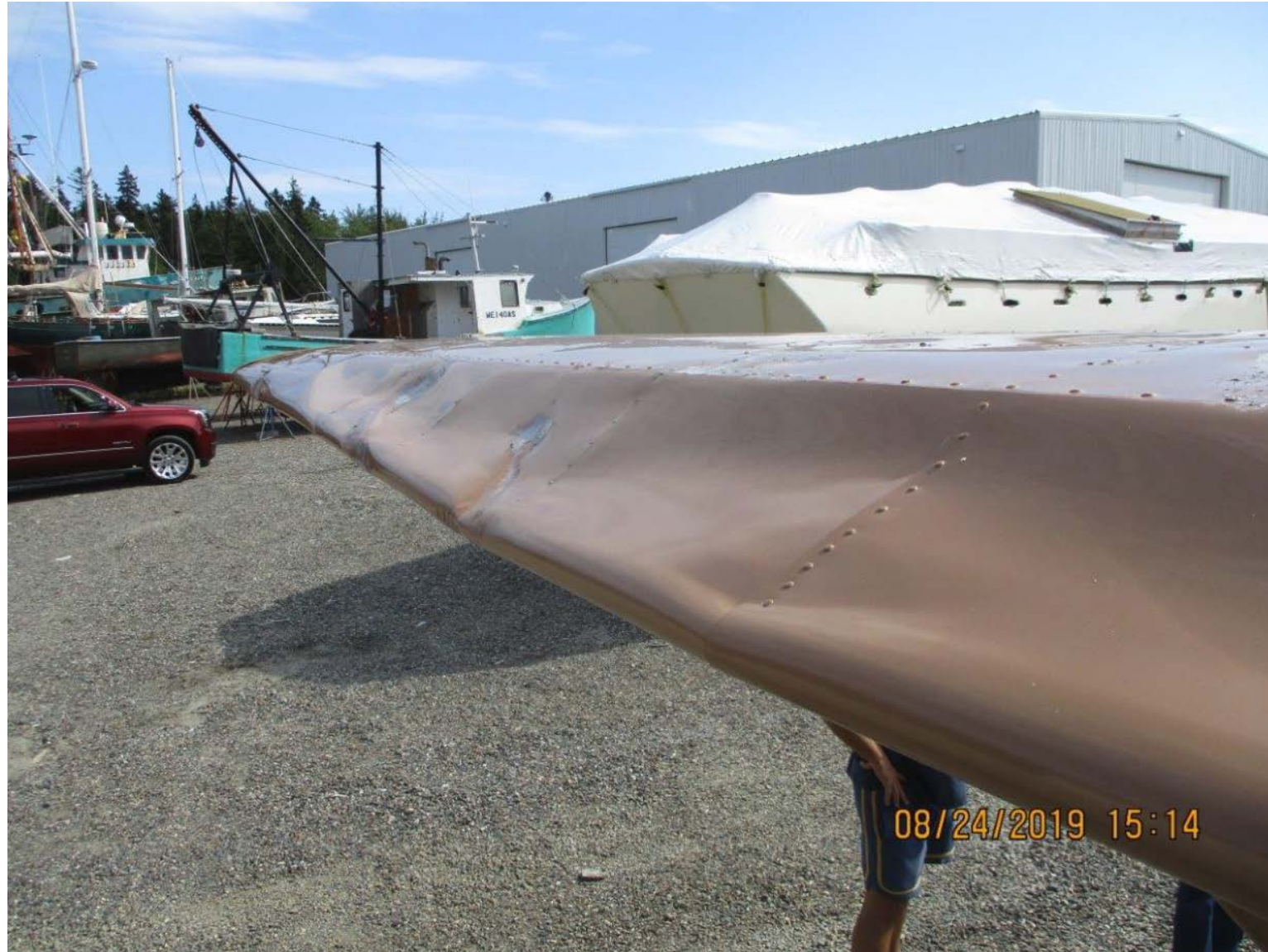
Photo 3 – View of right-wing substantial damage (Credit FAA)
