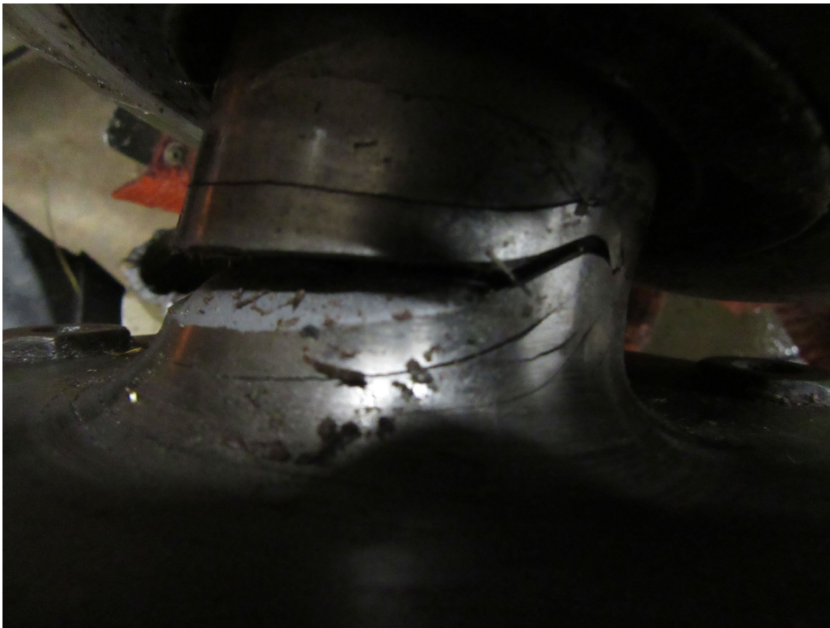
Photo 12 -Top View of Crankshaft Fracture – Courtesy of FAA
