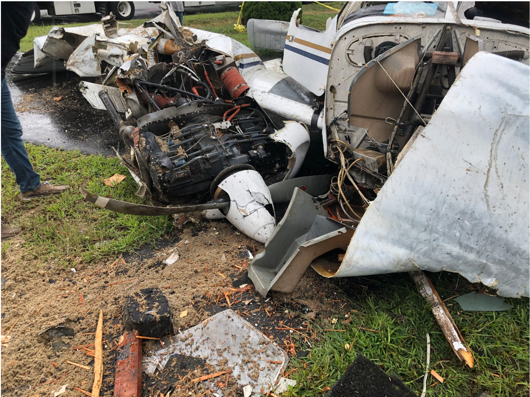
Photo 4 - Digital Photograph From Federal Aviation Administration. Frontal View of the Airplane, Right Wing, Right Engine Assembly and Right Propeller After Recovery From Roof.
