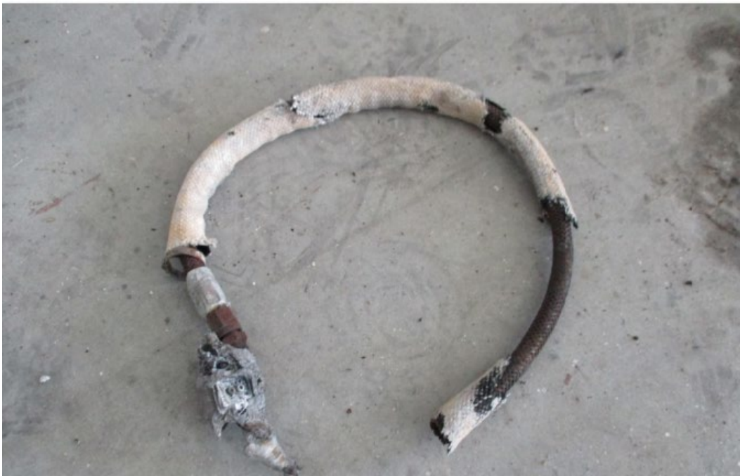
Photograph 3 – Accident airplane – Fuel line.
