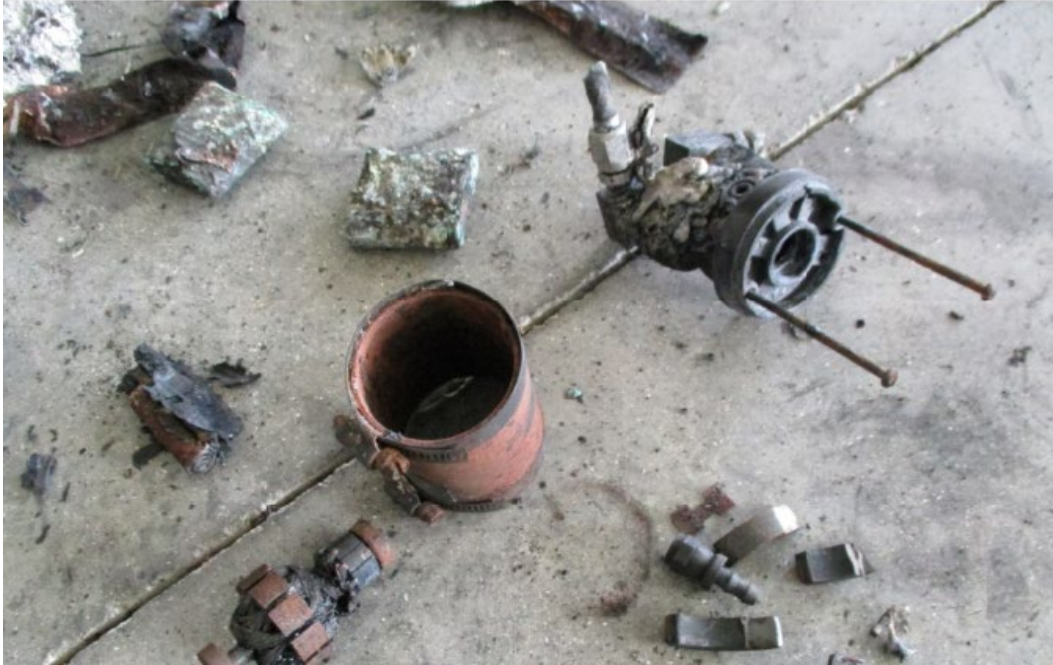
Photograph 2 – Accident airplane - Fuel Pump disassembled.
