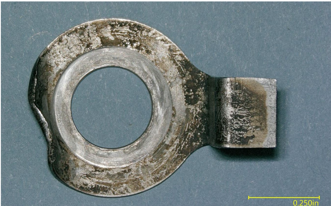
Figure 6 – The lock plate, viewed from the aft side, as received.
