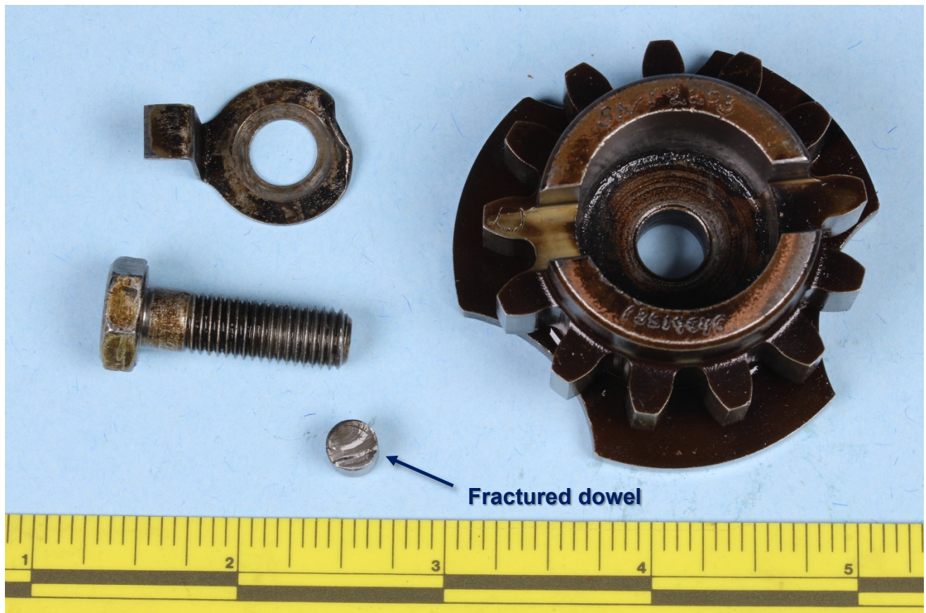
Figure 1 – View of the crankshaft drive gear, bolt, lockplate, and fractured pin, as received.
