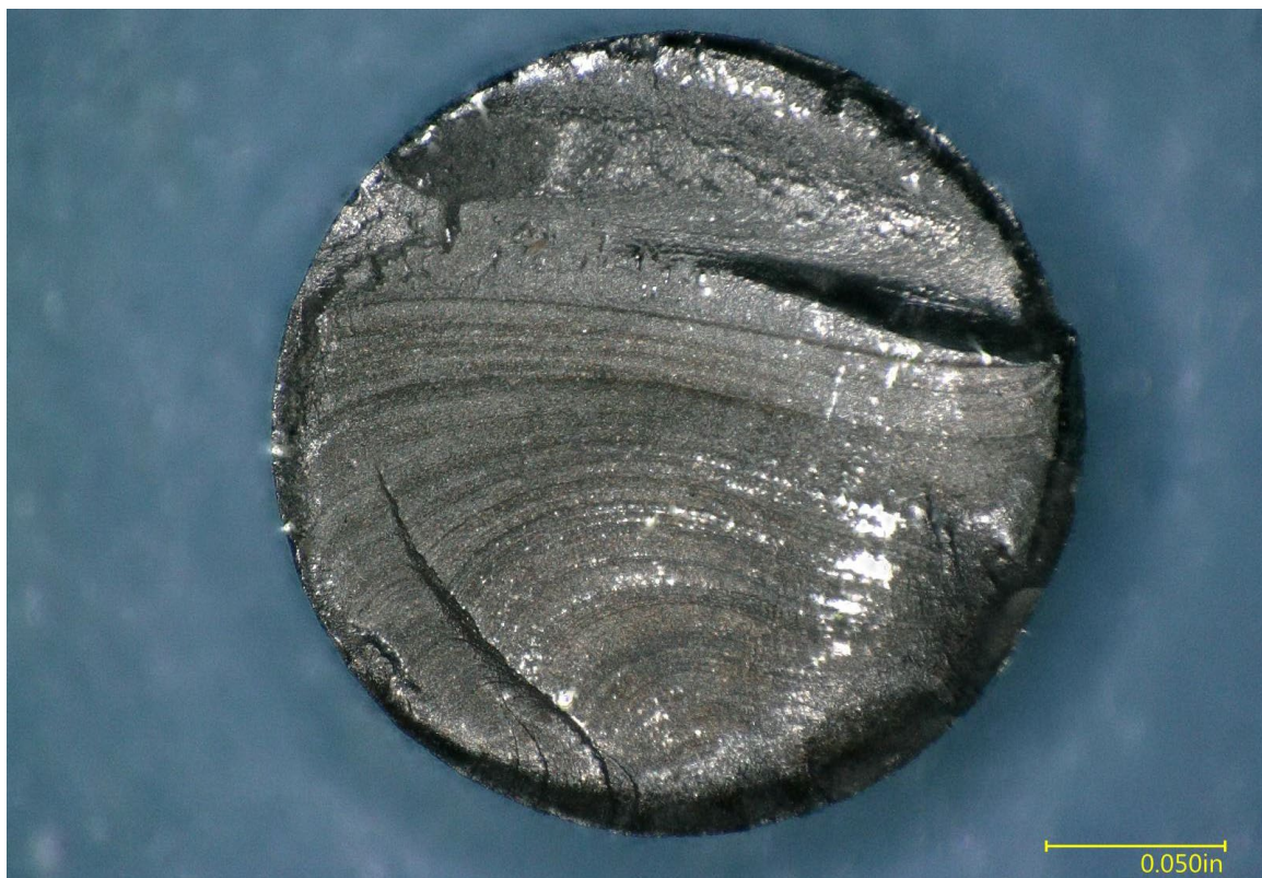
Figure 8 – View of the fracture surface of the dowel remnant.
