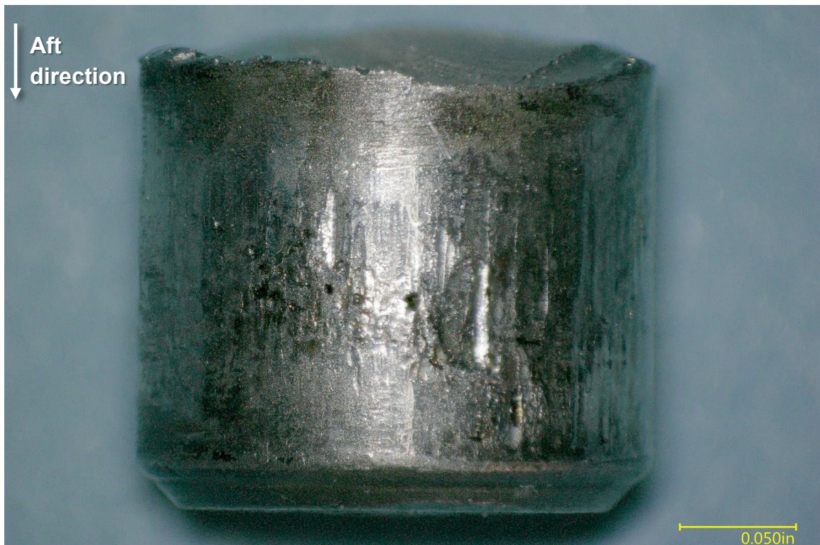
Figure 7 – View of the fractured crankshaft dowel from the side.
