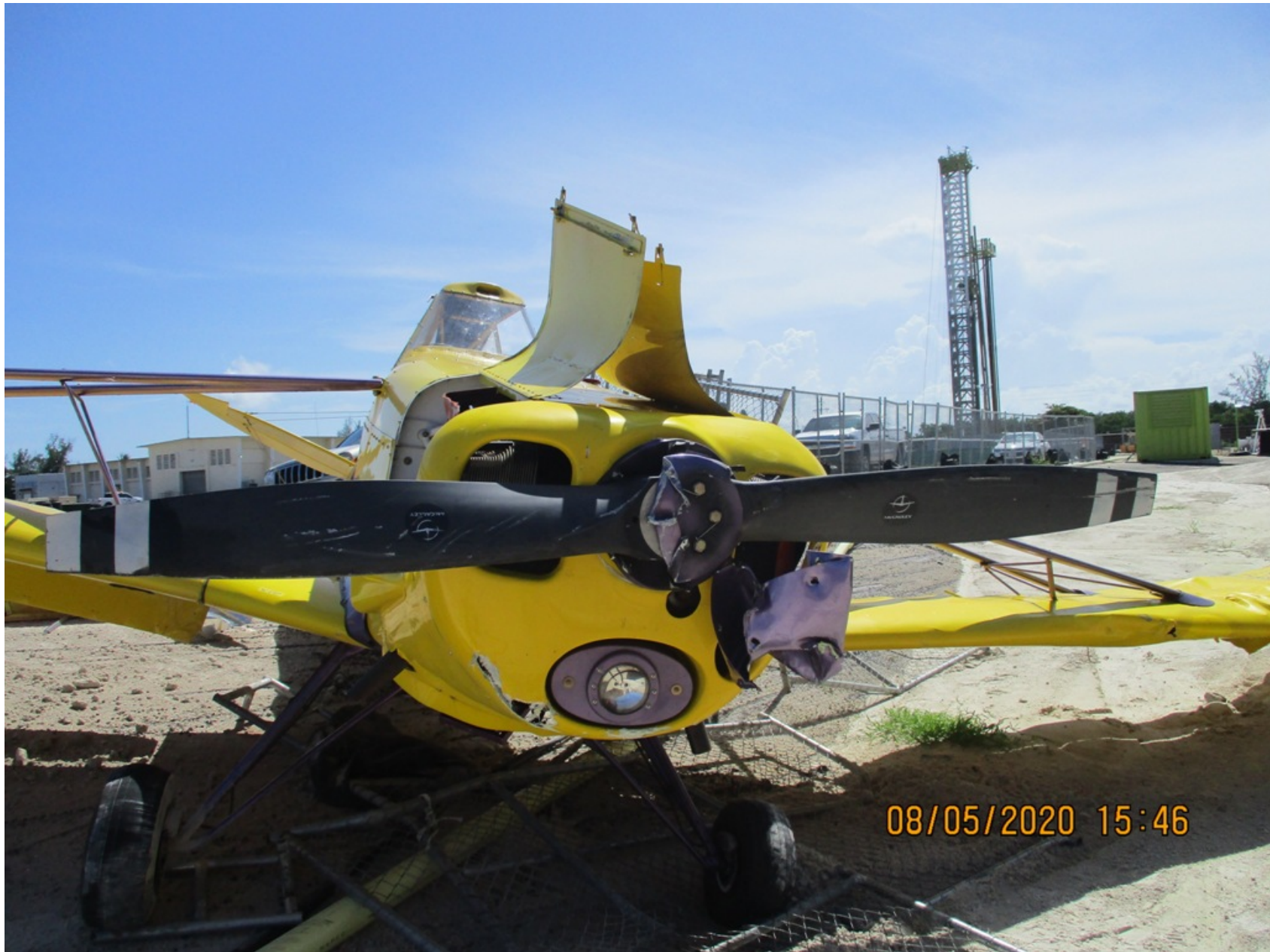
Photo 3 - Digital Photograph from FAA. Close-Up Frontal View of the Propeller and Portions of the Fuselage and Both Wings At the Accident Site. Note the Damage to The Propeller Spinner and Scratches to the Propeller.
