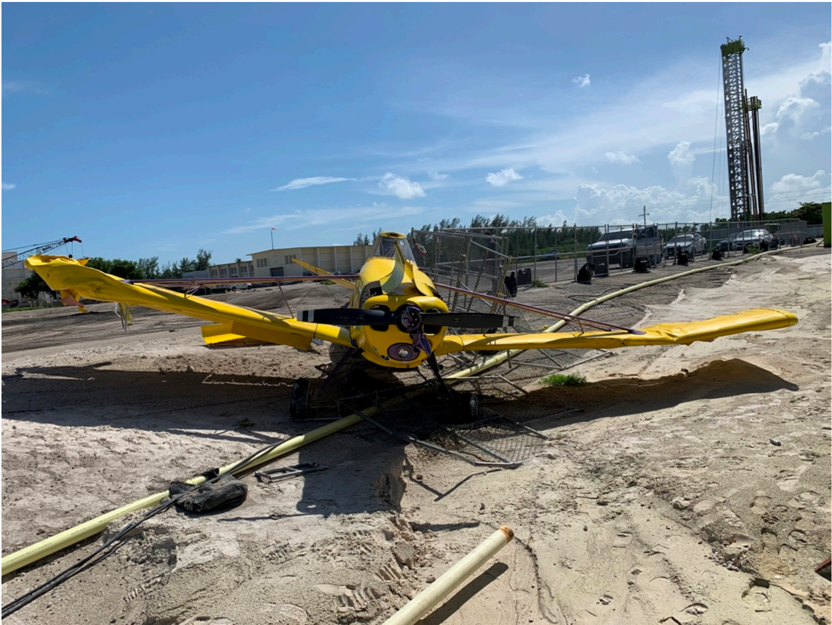
Photo 1 – Digital Photograph from FAA. Front View of the Airplane At the Accident Site. Note the substantial Damage to Both Wings.
