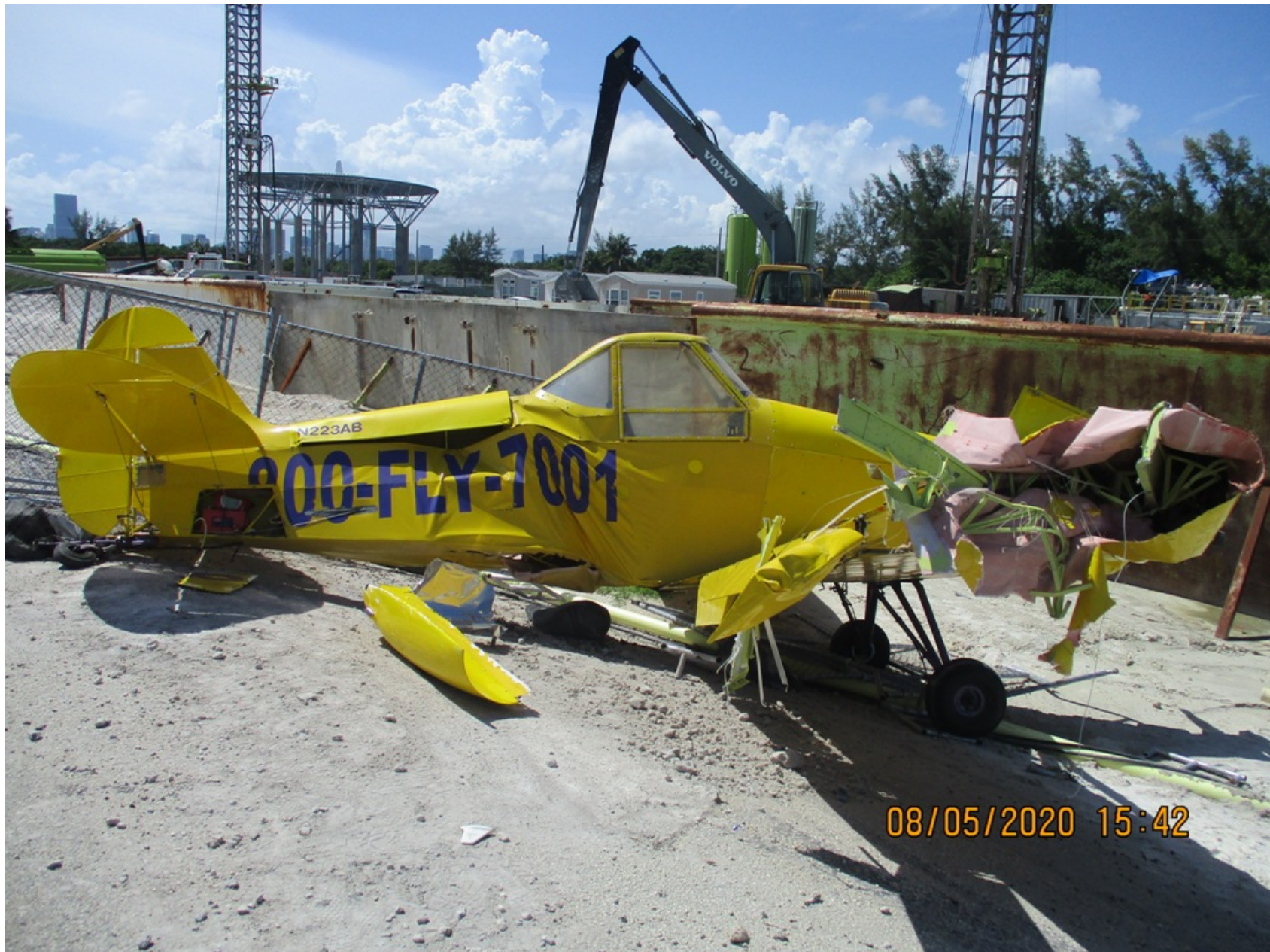
Photo 2 - Digital Photograph from FAA. Right Side View of the Airplane At the Accident Site. Note the substantial Damage to The Right Wing and Empennage.
