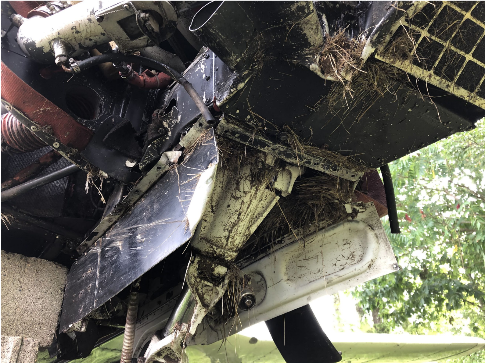
Photo 7 – Displaced and Twisted Tunnel and Wheel Well Area – Courtesy of McLarens Adjusters
