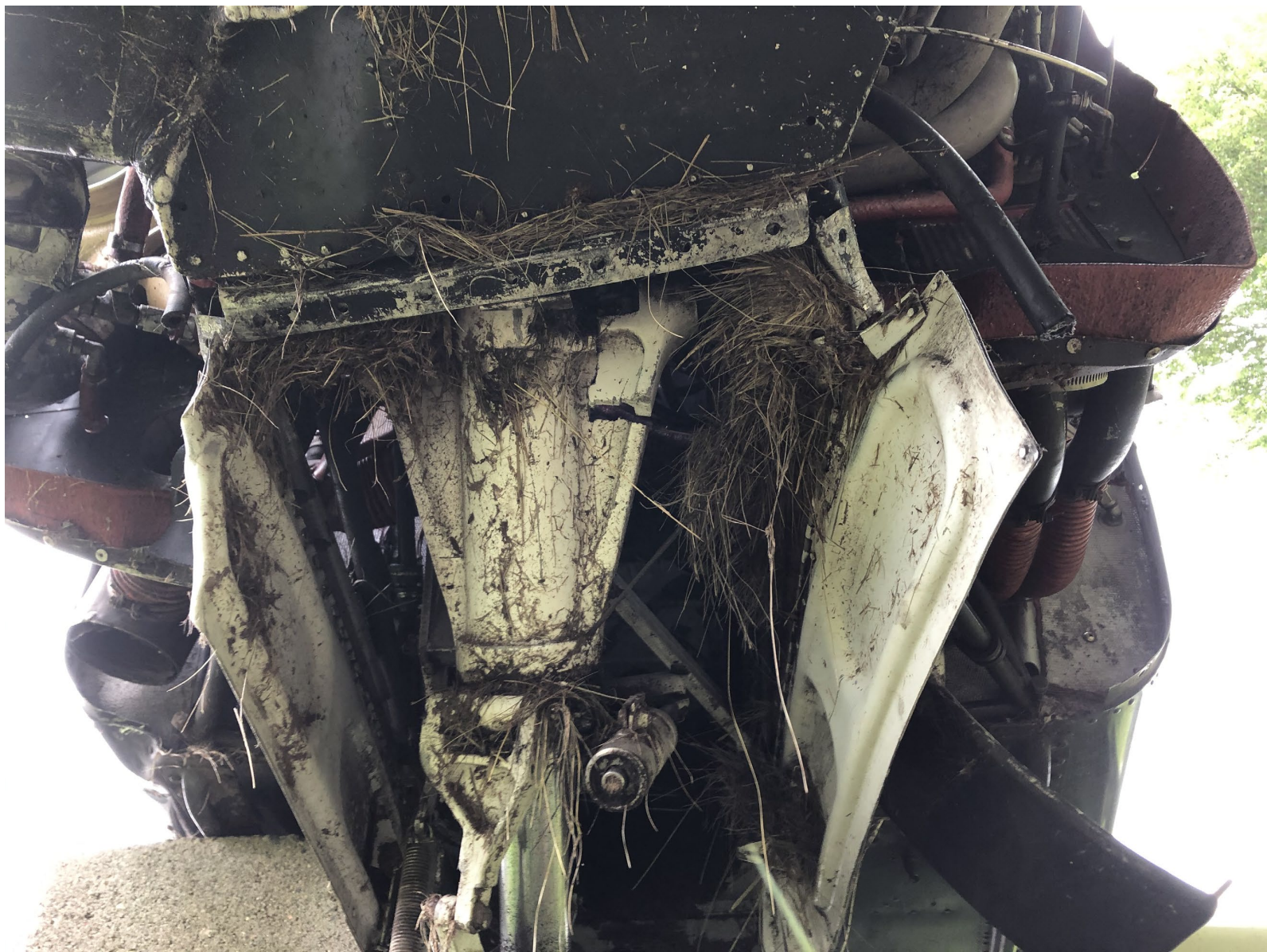
Photo 13 – Bottom View of Engine Showing Displacement to Right of Mounting Location – Courtesy of McLarens Adjusters
