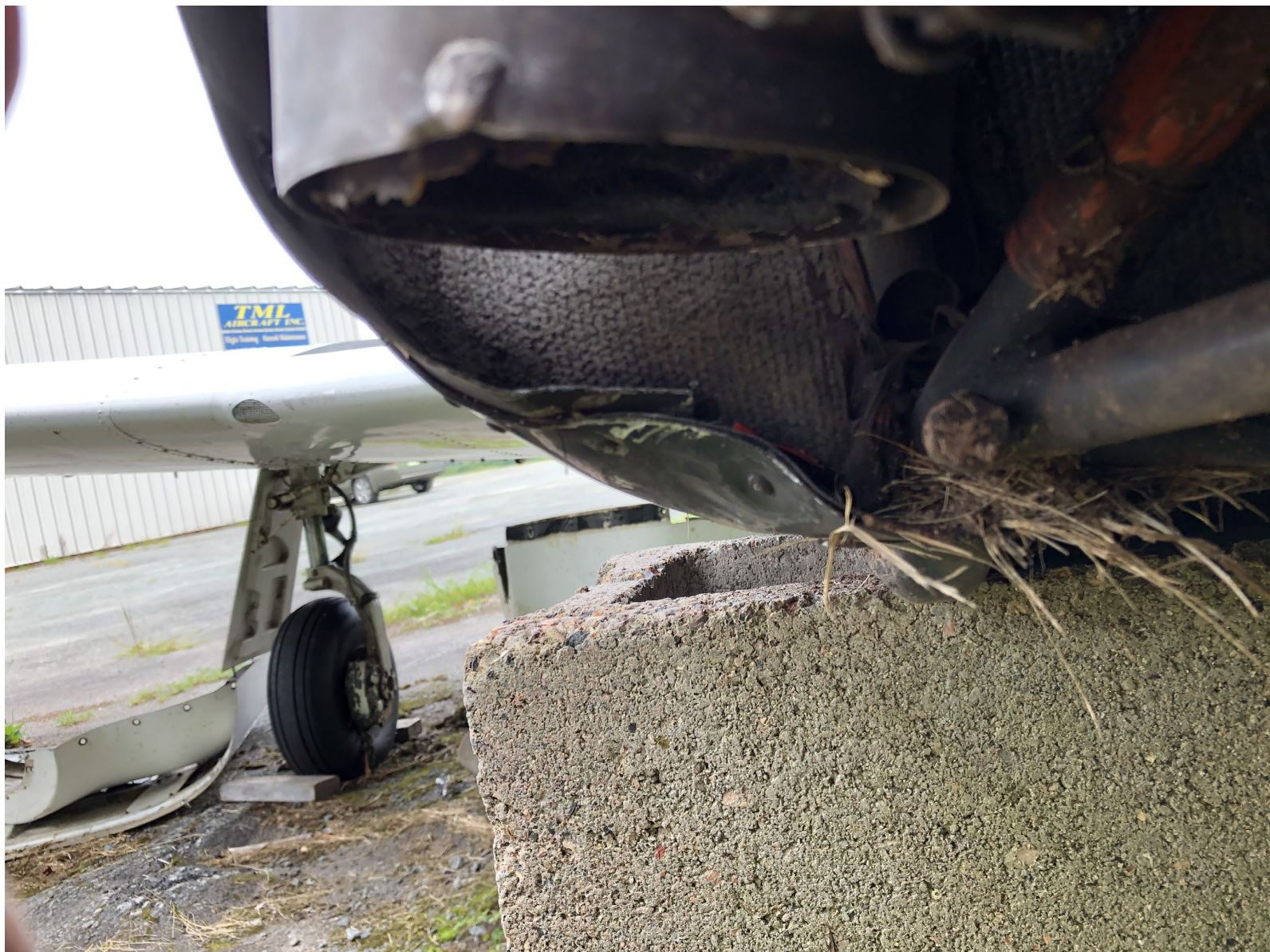
Photo 9 – Right Side of Front Lower Fuselage Displaying Damage at Fuselage Firewall Structure – Courtesy of McLarens Adjusting
