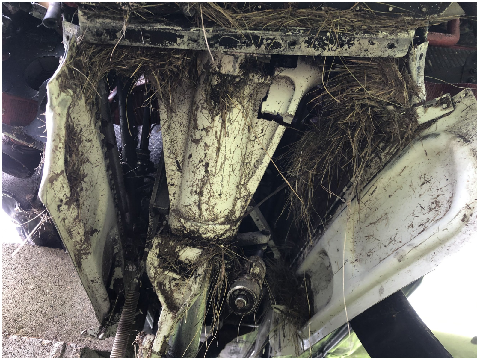
Photo 8 – Front of Nose Landing Gear Displaying Crack and Separation from Left Trunnion – Courtesy of McLarens Adjusters
