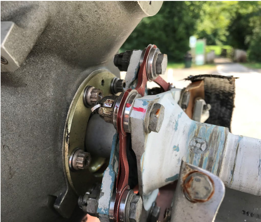
Photo 12: Tail Rotor Drive Coupling
