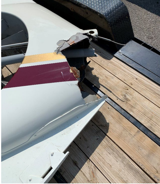
Photo 4: Fenestron Fracture Area
