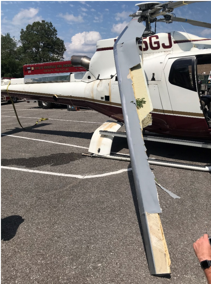
Photo 3: Main rotor blade damage
