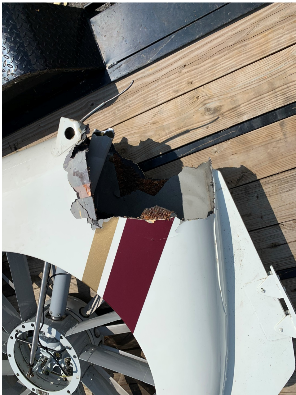
Photo 6 – View of Fenestron Fracture (Photo Courtesy of Airbus Helicopter)
