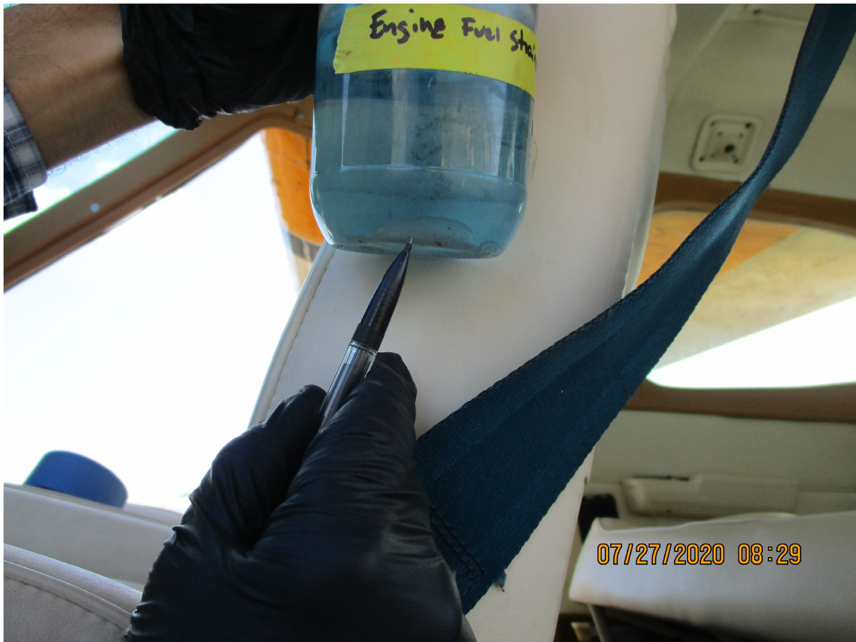
Photo 5 - FAA Digital Photograph. View of the Fuel Sample Drained From Fuel Strainer. Note the Pen Pointing to Water in Sample.
