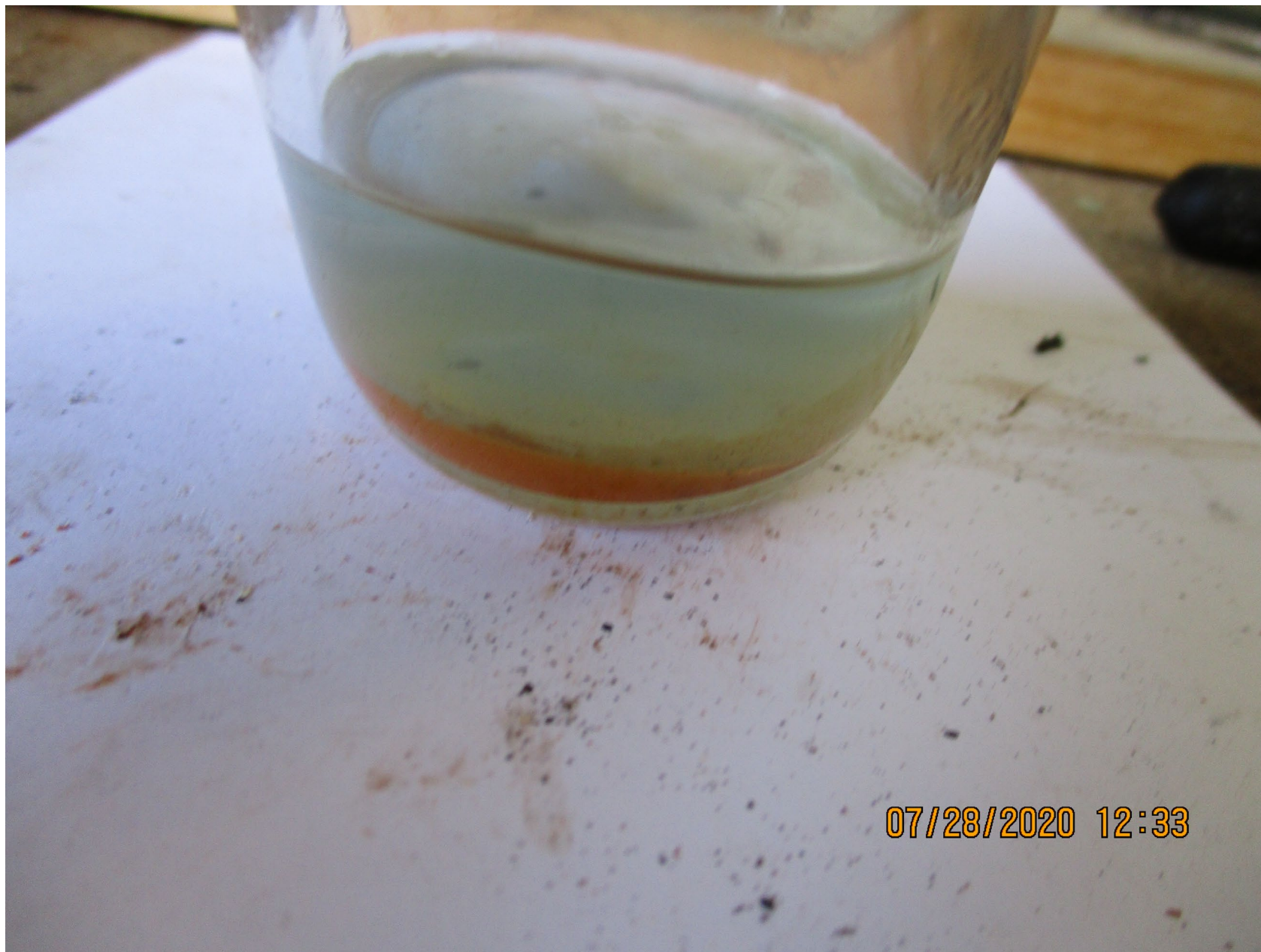
Photo 6 - FAA Digital Photograph. View of the Fuel Sample Drained From Servo Fuel Injector Inlet. Note the rust Colored Water Contamination in the Bottom of the Sample.
