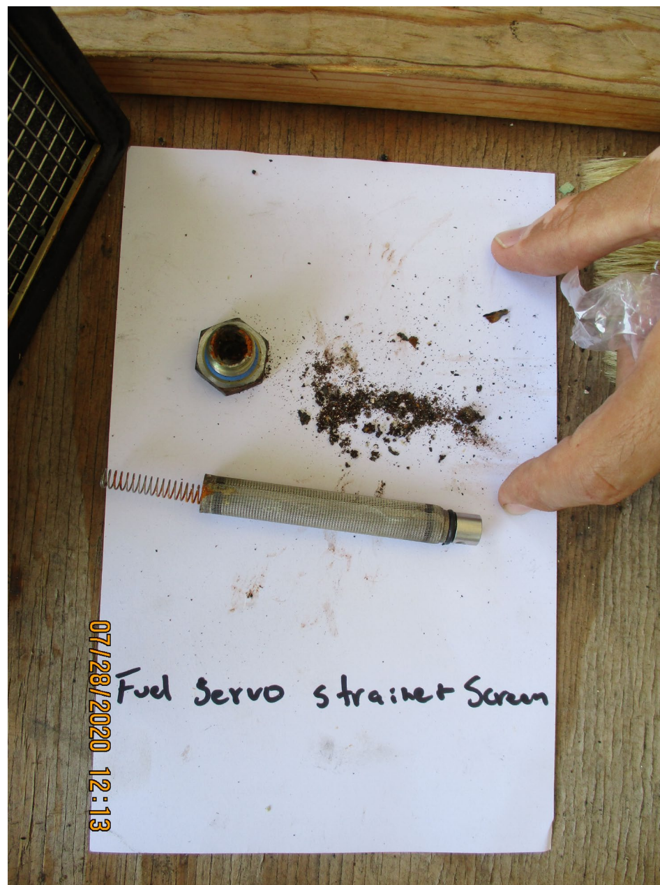
Photo 7 - FAA Digital Photograph. View of the Ferrous Contaminant Collected From Inside The Servo Fuel Injector Inlet Screen.
