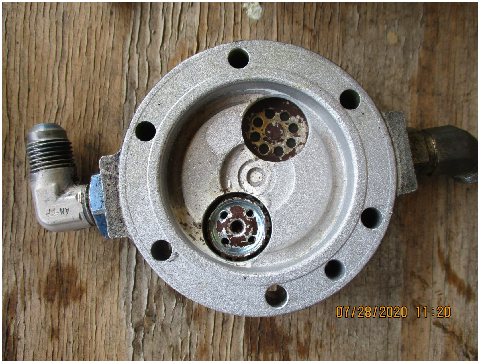
Photo 10 - FAA Digital Photograph. View of the Disassembled Engine-Driven Fuel Pump. Note the Corrosion of the Internal Valves.
