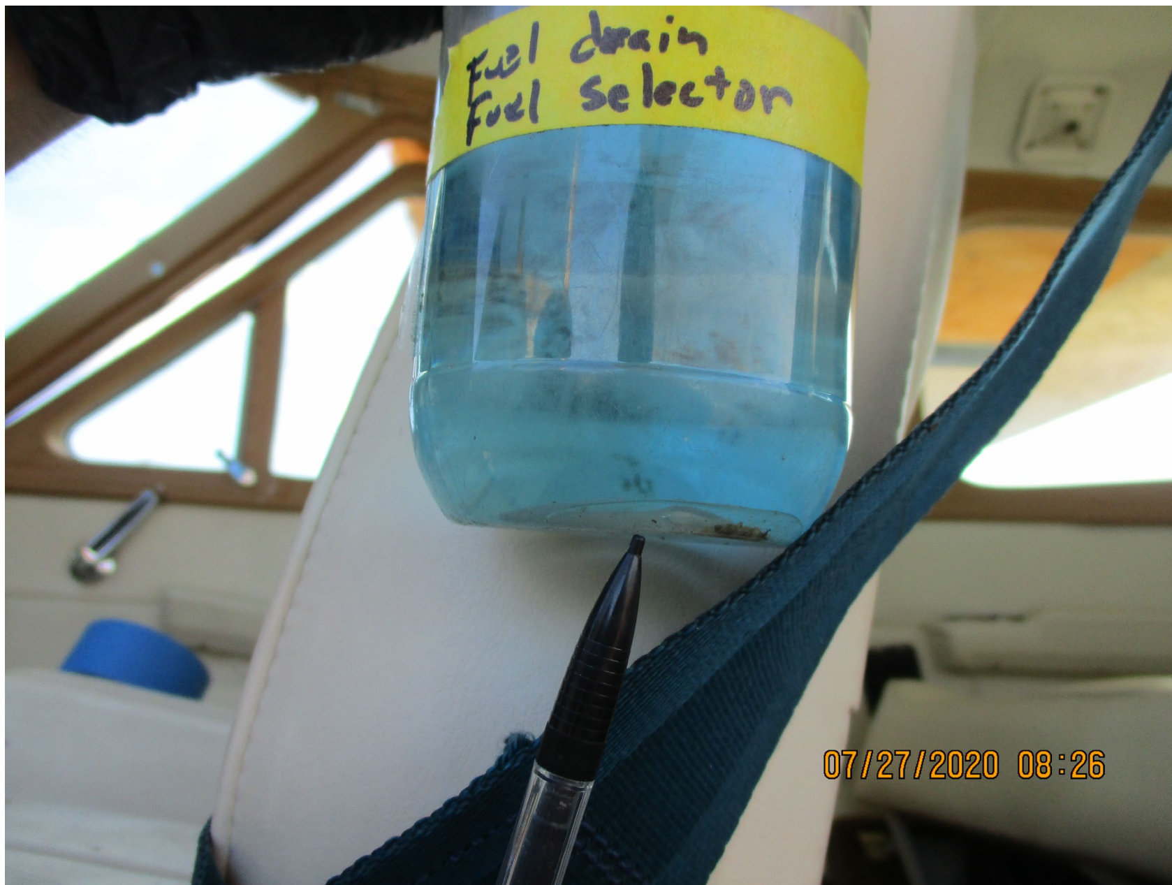
Photo 4 - FAA Digital Photograph. View of the Fuel Sample Drained From Fuel Reservoir Tank Assembly. Note the Pen Pointing to Water in Sample.
