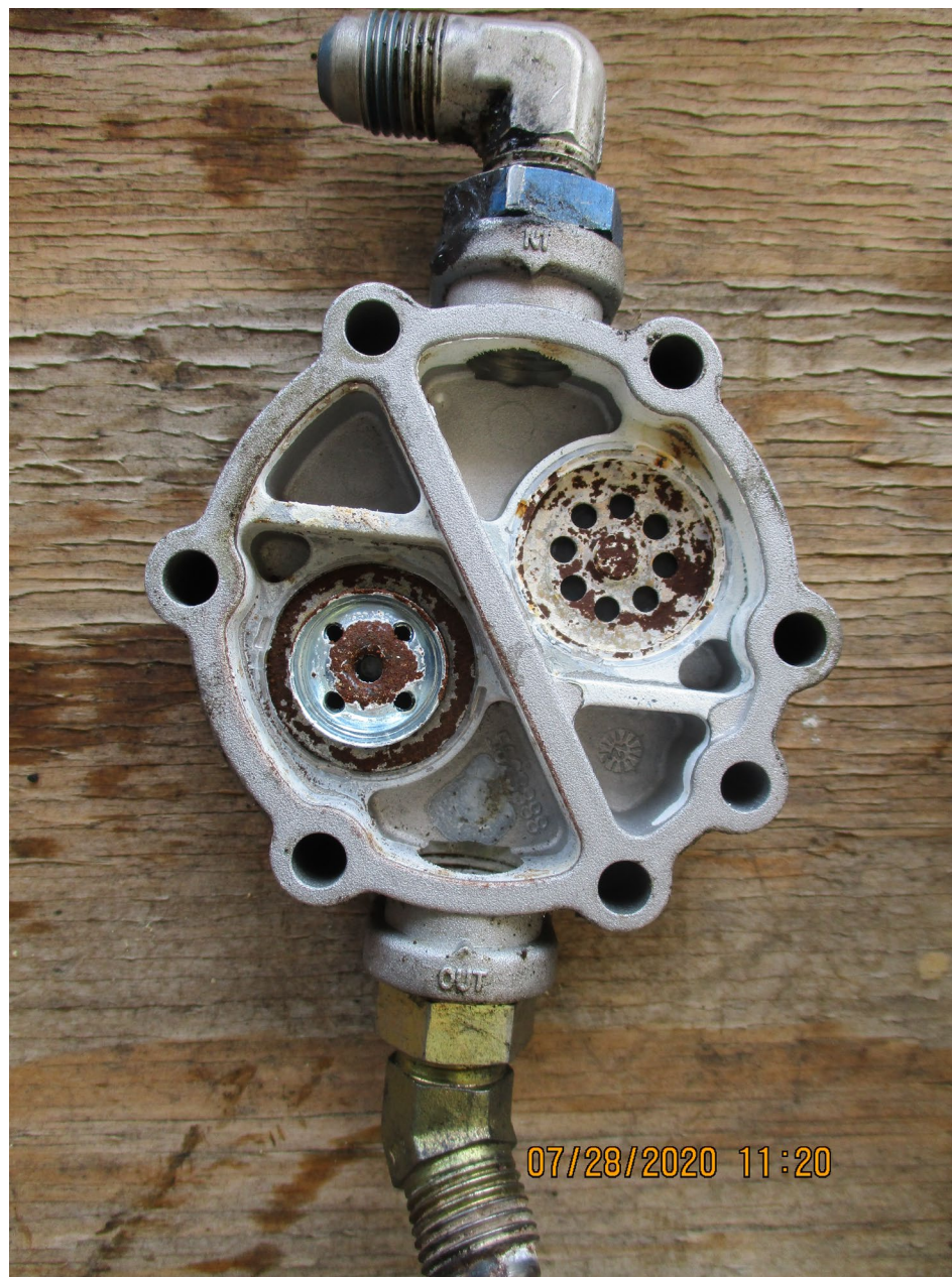
Photo 9 - FAA Digital Photograph. View of the Disassembled Engine-Driven Fuel Pump. Note the Corrosion of the Internal Valves.
