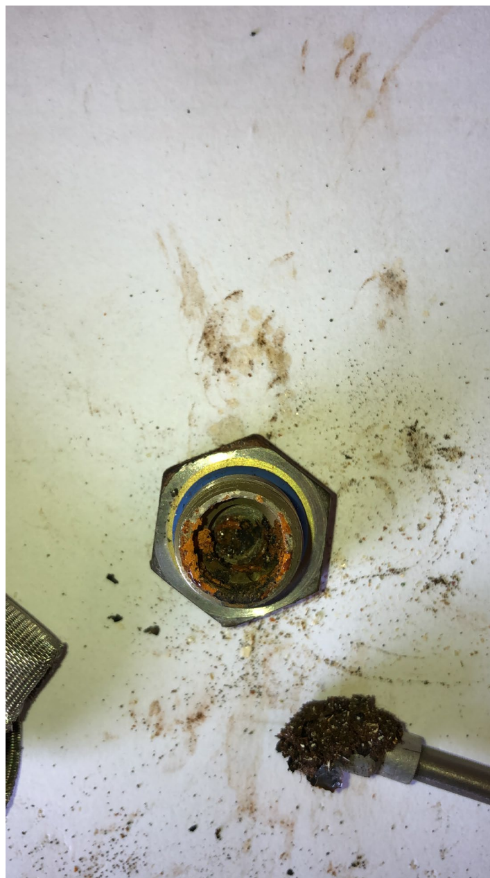
Photo 8 - FAA Digital Photograph. View of the Ferrous Contaminant Recovered From the Inlet Screen of the Servo Fuel Injector. Note the Corrosion of the Plug.
