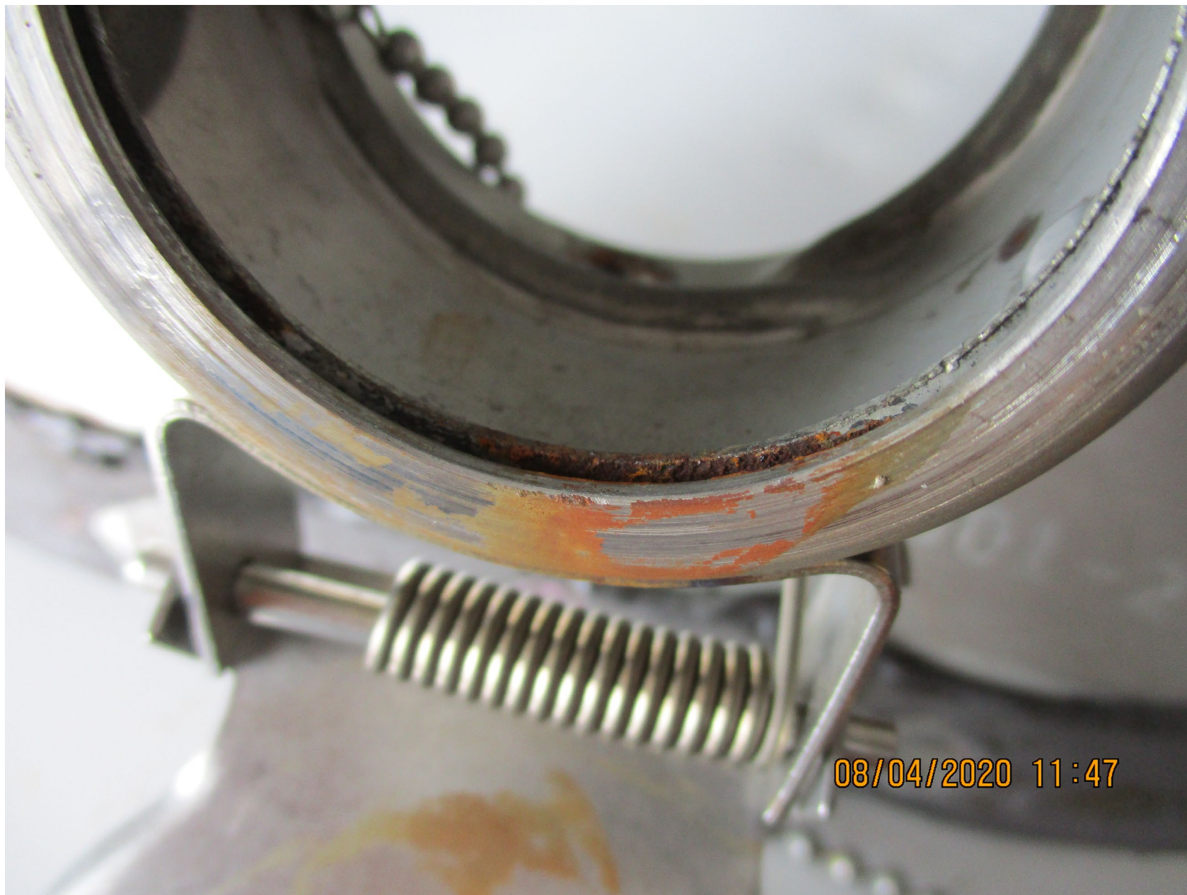
Photo 12 - FAA Digital Photograph. View of the Right Fuel Cap Assembly. Note the Corrosion.
