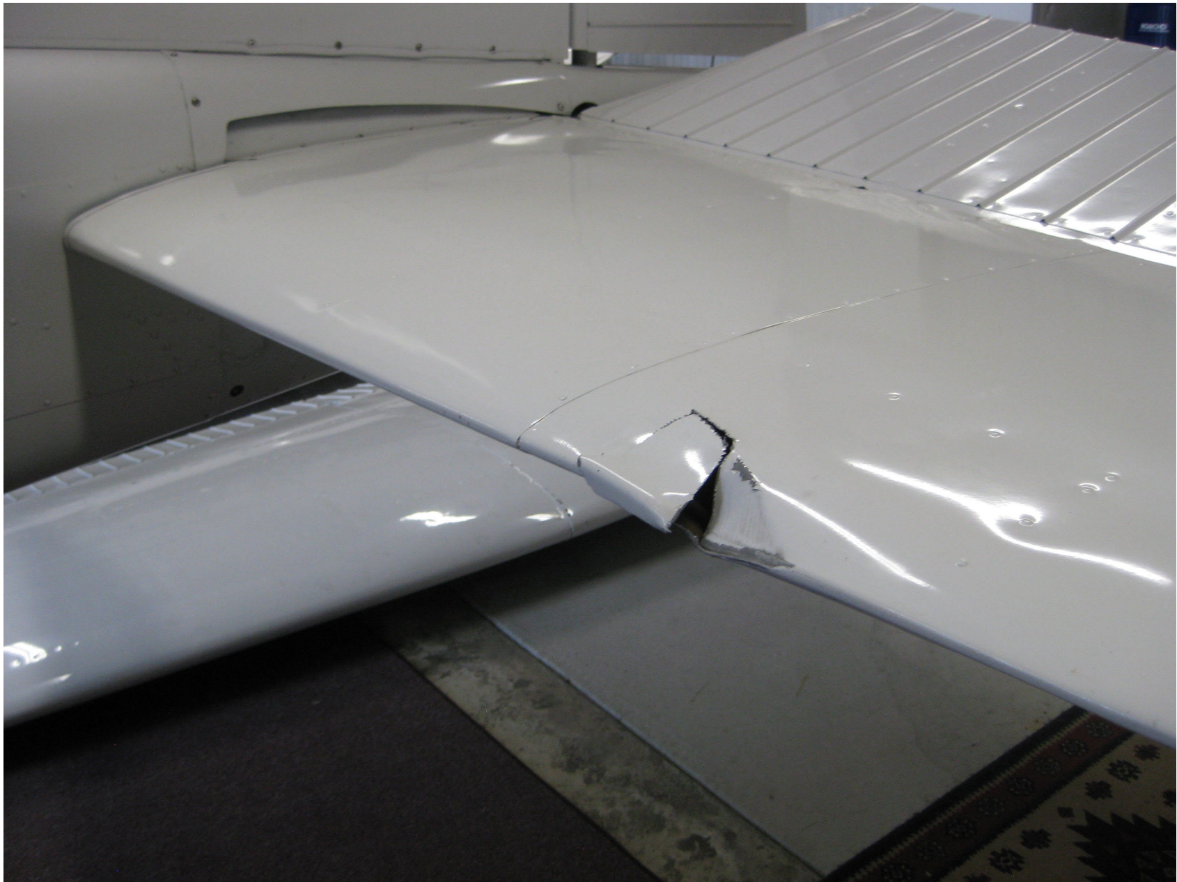
Photo 8 – Damage to Left Horizontal Stabilizer – Courtesy of FAA
