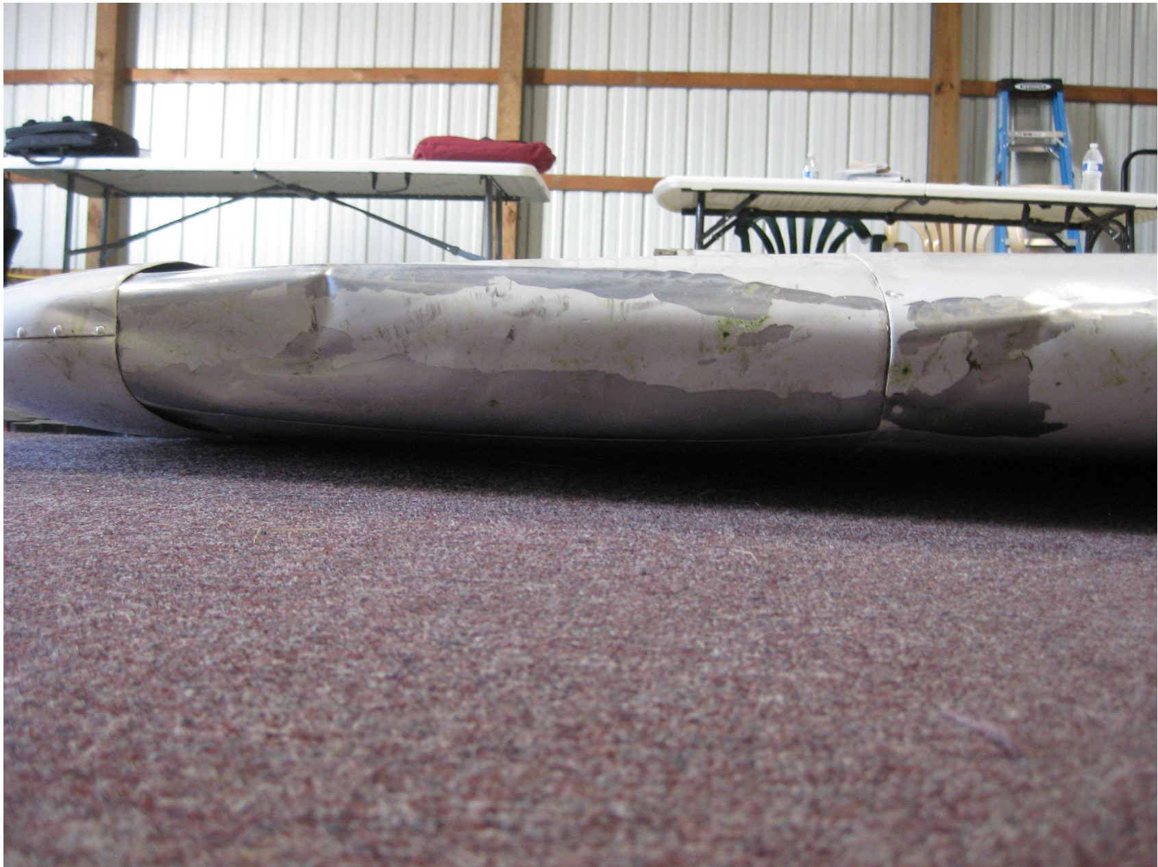
Photo 7 – Damage to Right Wingtip – Courtesy of FAA
