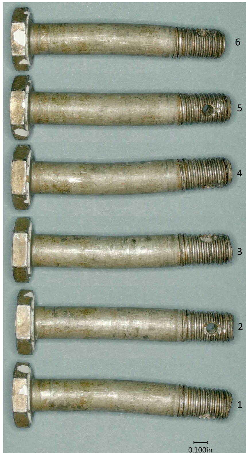
Figure 25 Digital microscope images of the pivot bolt between the left main landing gear upper and lower torque arm pieces.
