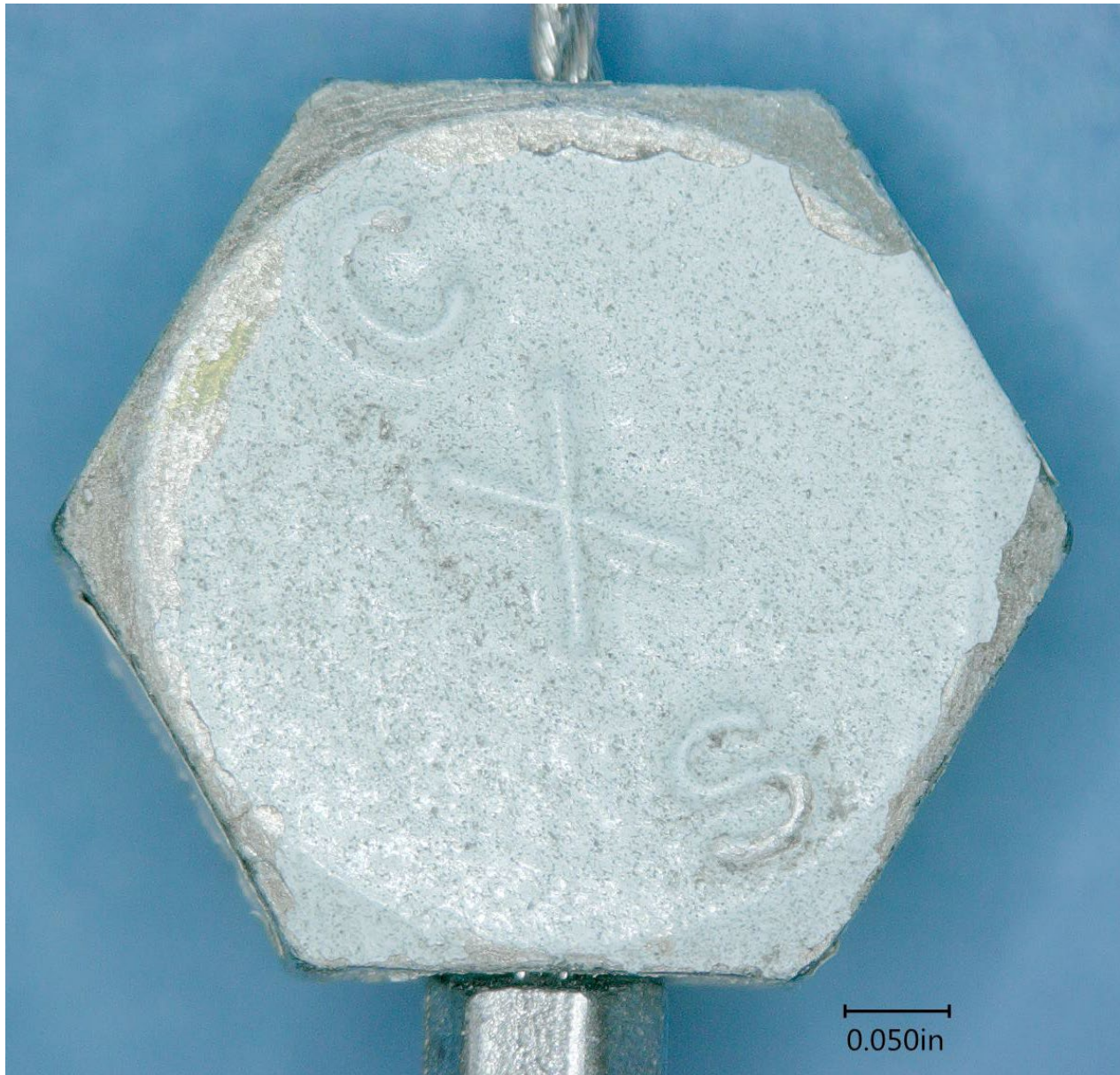
Figure 17 The top side of the Bolt 1 head revealing manufacturing markings.
