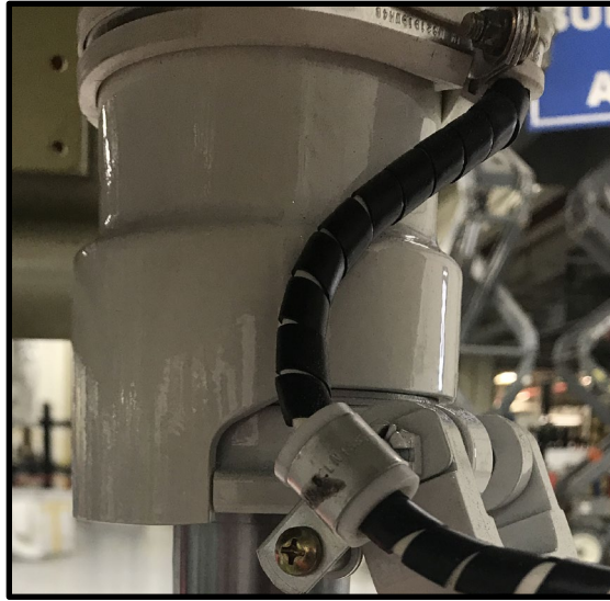
Figure 5-M600 Right turn mechanical stop between trunnion and strut just prior to engagement.
