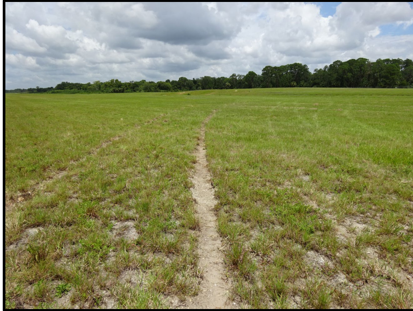
Figure 10-Ground scars in grass on the right side of Runway 27 from landing gear.
