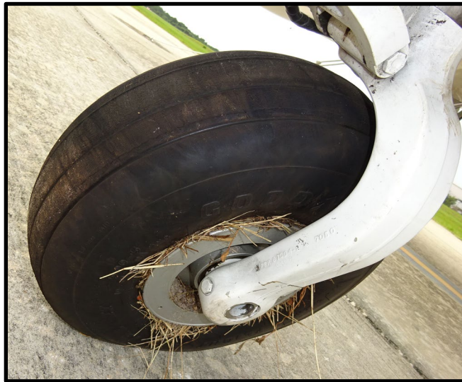
Figure 8-NLG tire with embedded dirt and grass and crosswise scuffing.
