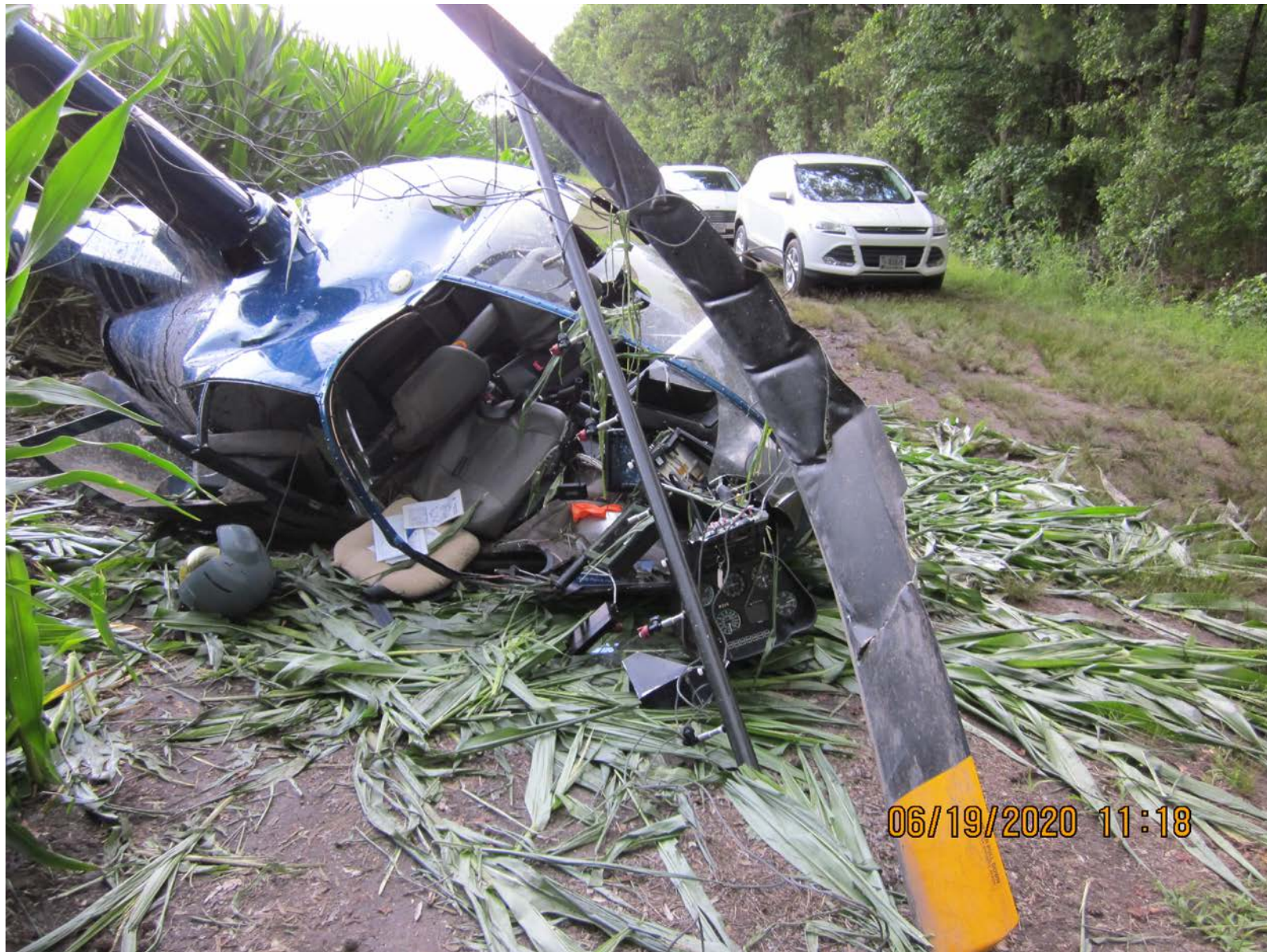
Photo 3 – View of front right side of helicopter showing damage to the fuselage and cockpit. (Courtesy of FAA)
