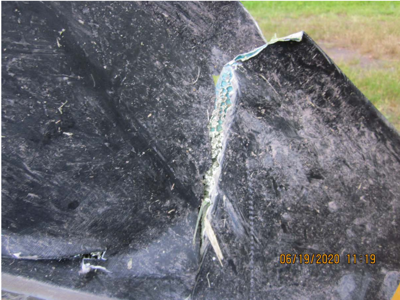
Photo 5 – Close up view of damaged rotor blade. (Courtesy of FAA)
