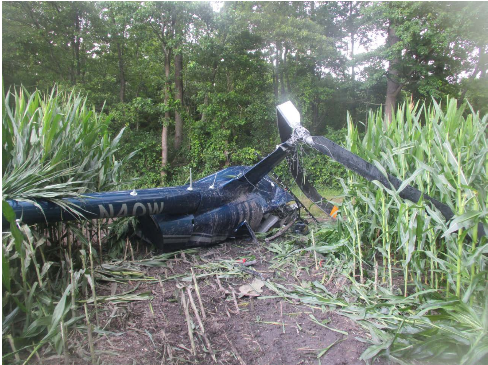
Photo 8 – View of right aft side of helicopter from the direction of travel through the corn. Note the wire wrapped around the rotor blades. (Courtesy of FAA)
