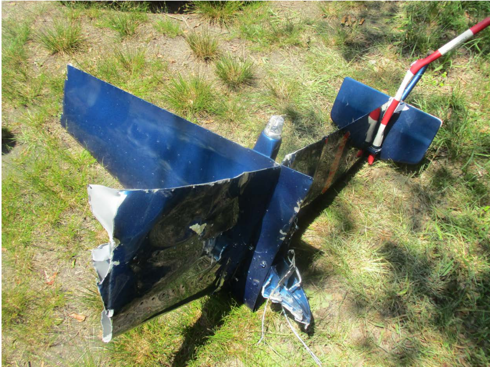
Photo 9 – View of separated empennage. Note: tail rotor separated during impact. (Courtesy of FAA)
