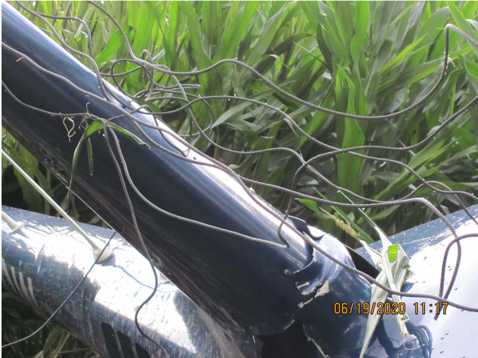
Photo 4 – Close up view of wire wrapped around the mast. (Courtesy of FAA)
