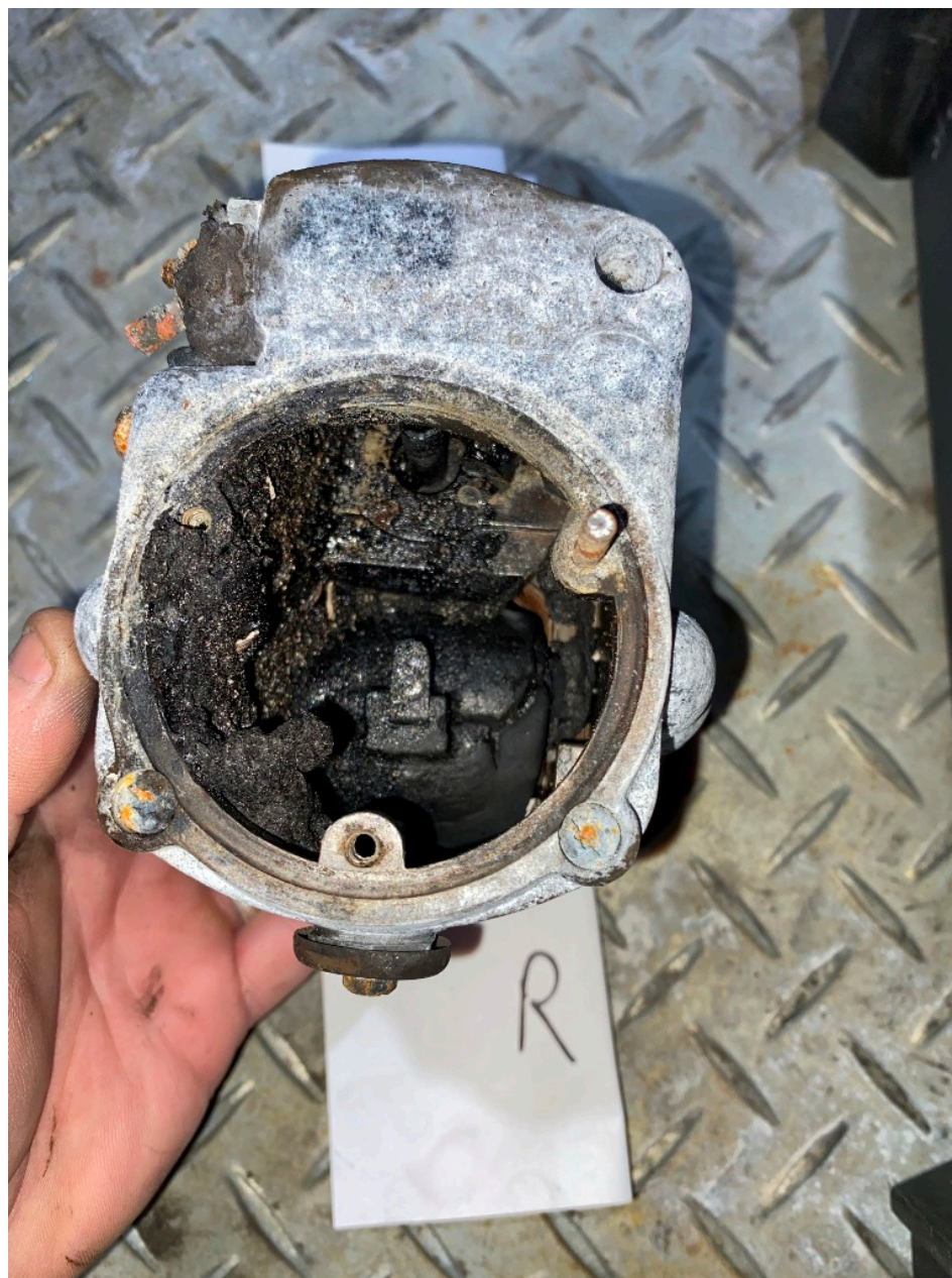
Photo 9 - Digital Photograph From Florida Air Recovery. View Showing the Internal Condition of the Right Magneto. Note the Extensive Postimpact Heat Damage.
