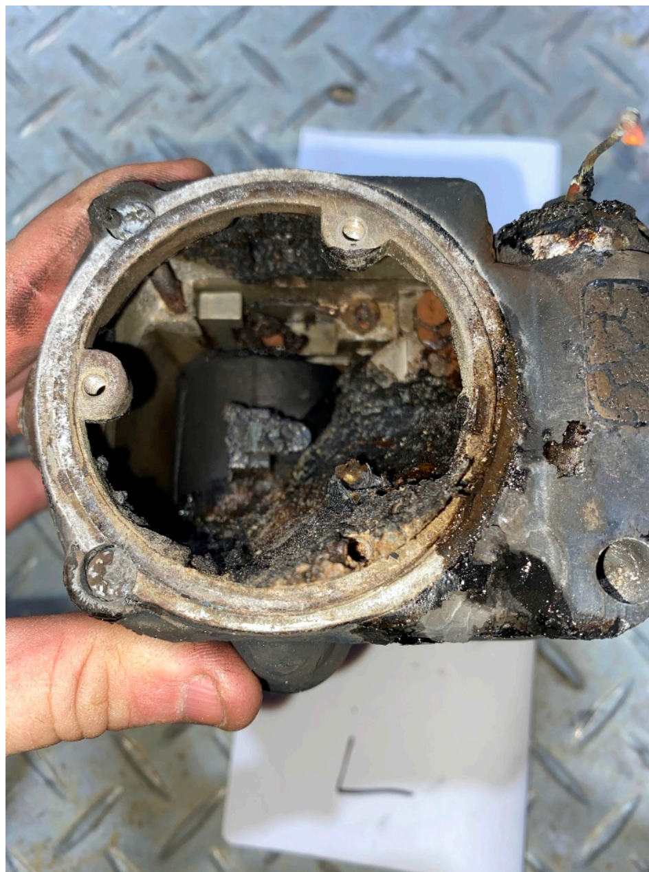
Photo 8 - Digital Photograph From Florida Air Recovery. View Showing the Internal Condition of the Left Magneto. Note the Extensive Postimpact Heat Damage.
