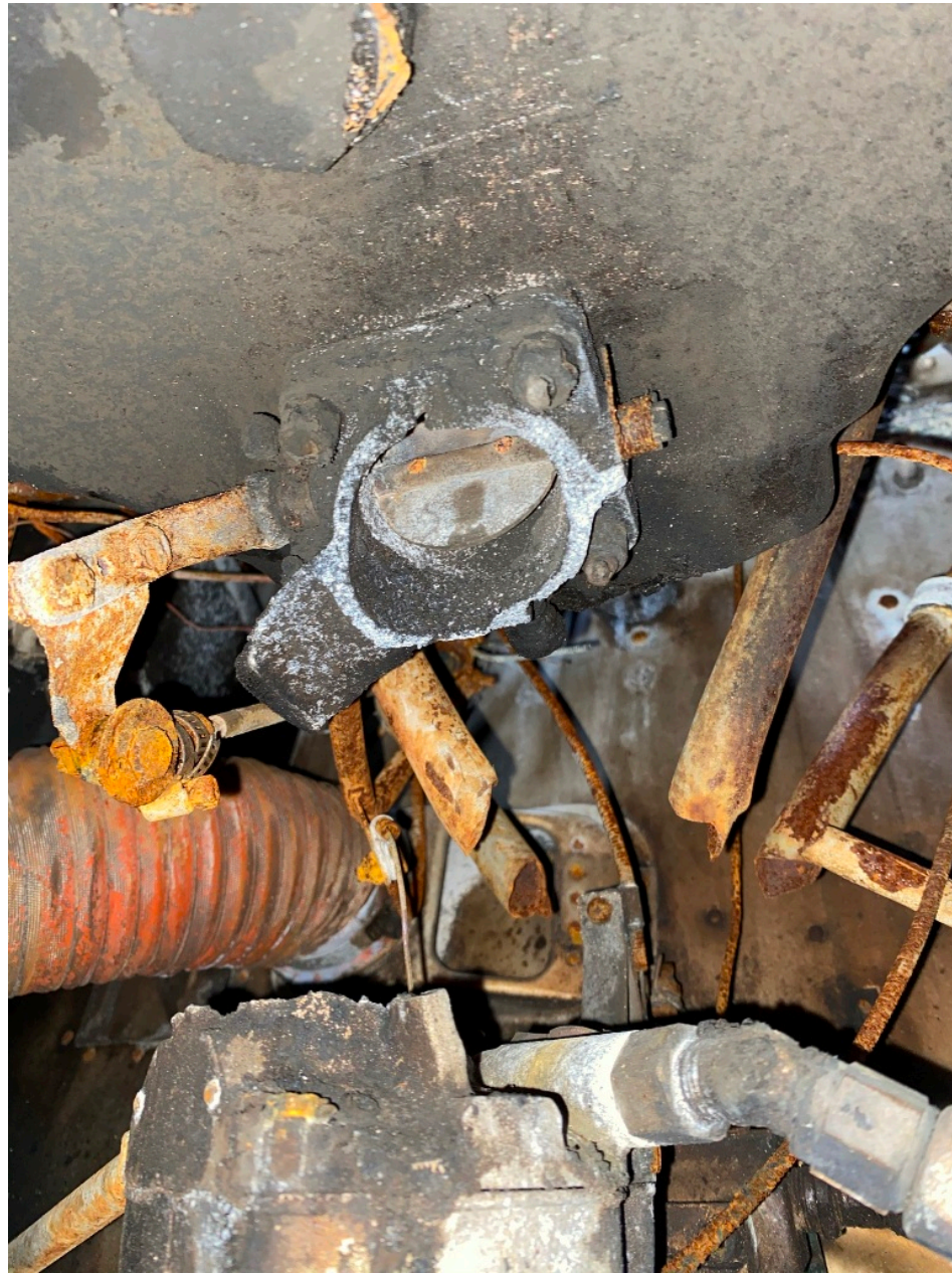
Photo 5 - Digital Photograph From Florida Air Recovery. View Showing the Fractured Throttle Body of the Carburetor. Note the Heat Damage in the Surrounding Area.
