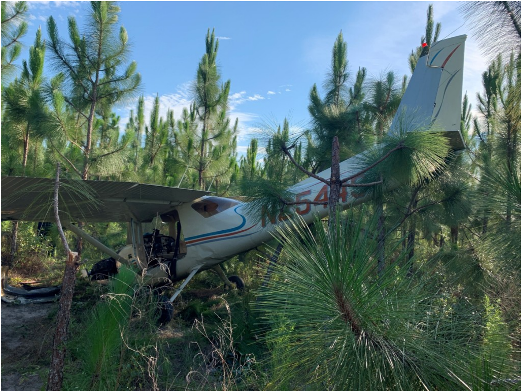
Photo 2 - Digital Photograph From Adam McCook. Left Side View of the Airplane at The Accident Site. Note the Compression Wrinkle in the Fuselage Near the Left Main Landing Gear Attach Point.
