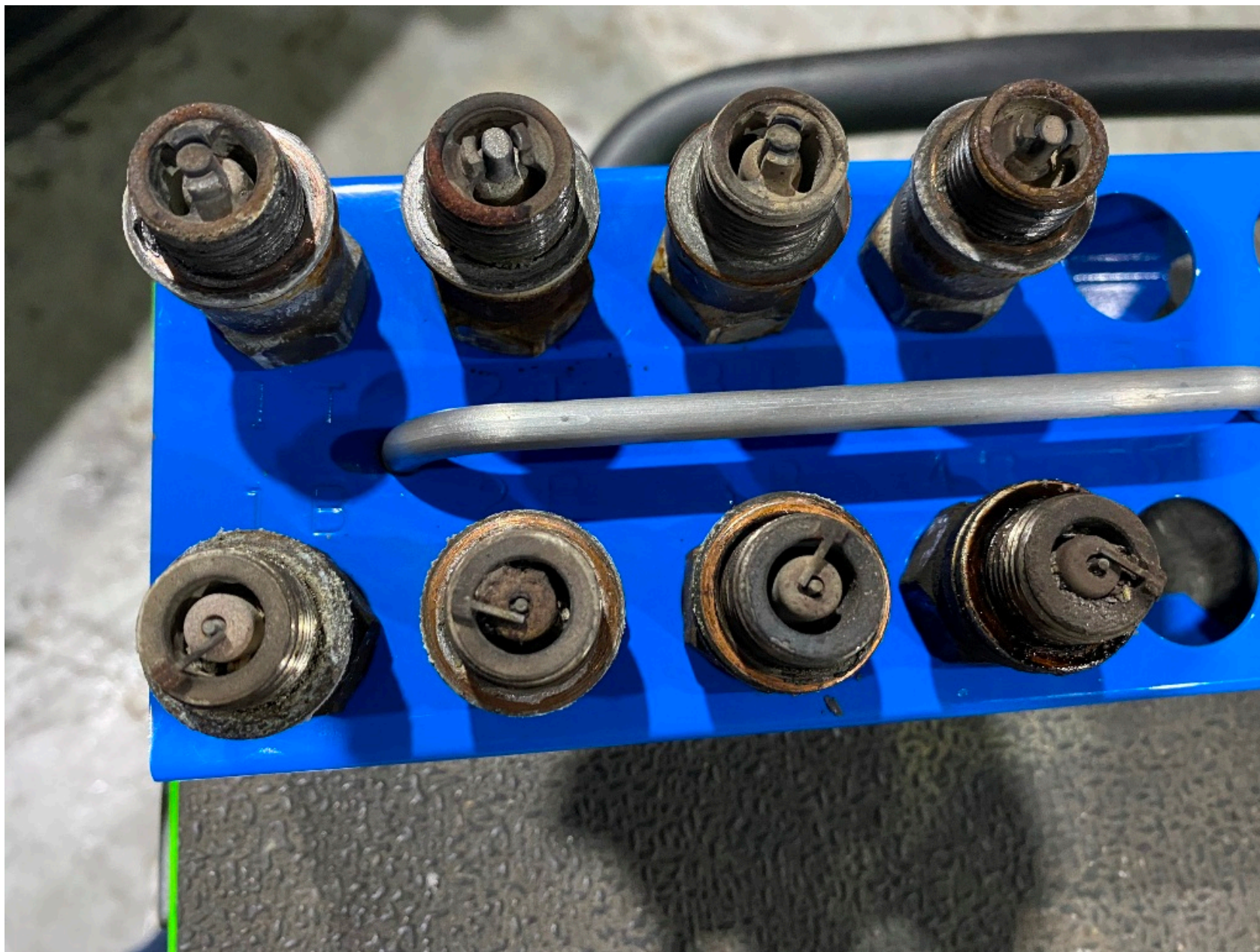
Photo 7 - Digital Photograph From Florida Air Recovery. View Showing the Condition of the Spark Plugs.
