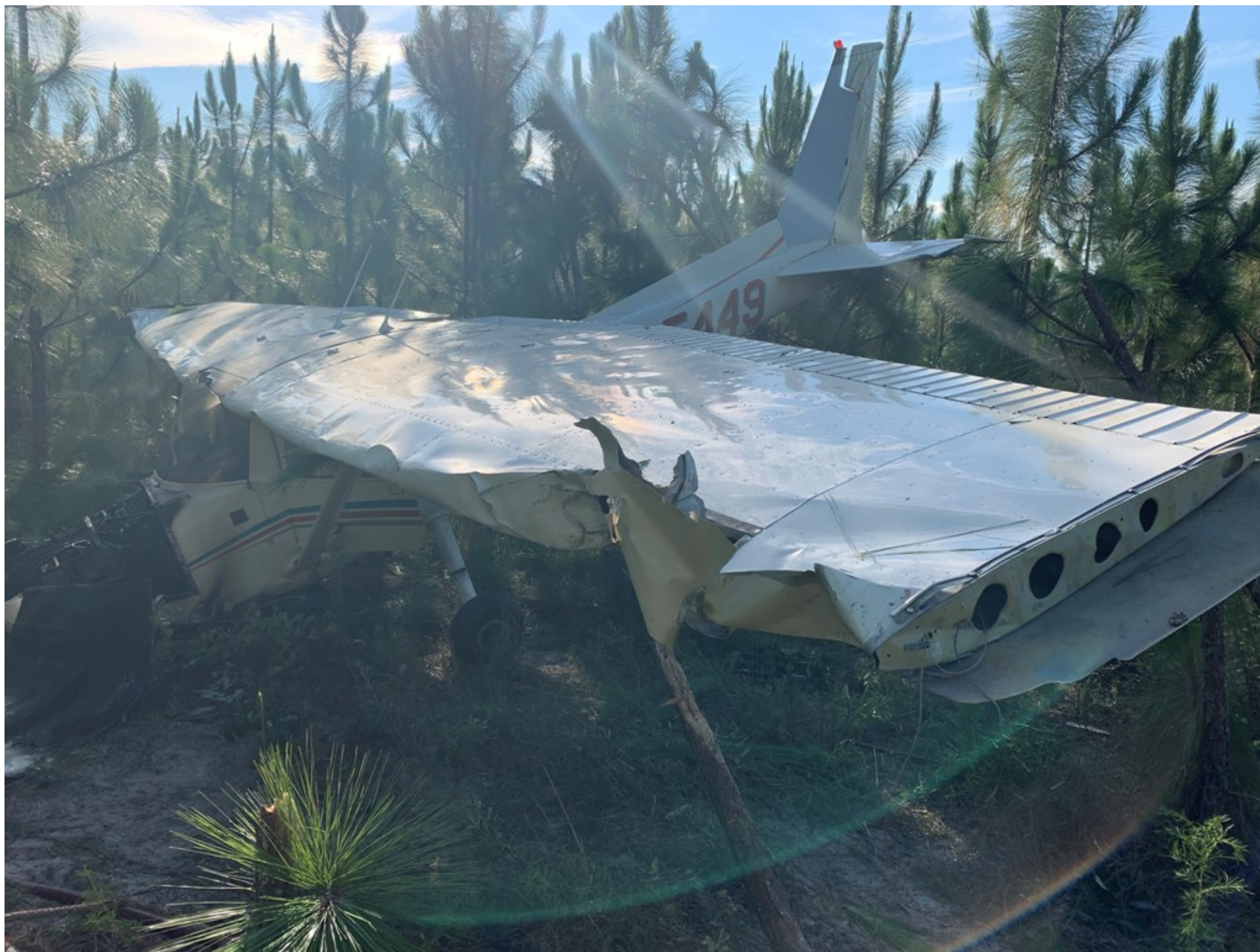
Photo 1 – Digital Photograph From Adam McCook. Left Side View of the Airplane at the Accident Site. Note the Extensive Damage to the Leading Edge of the Left Wing.
