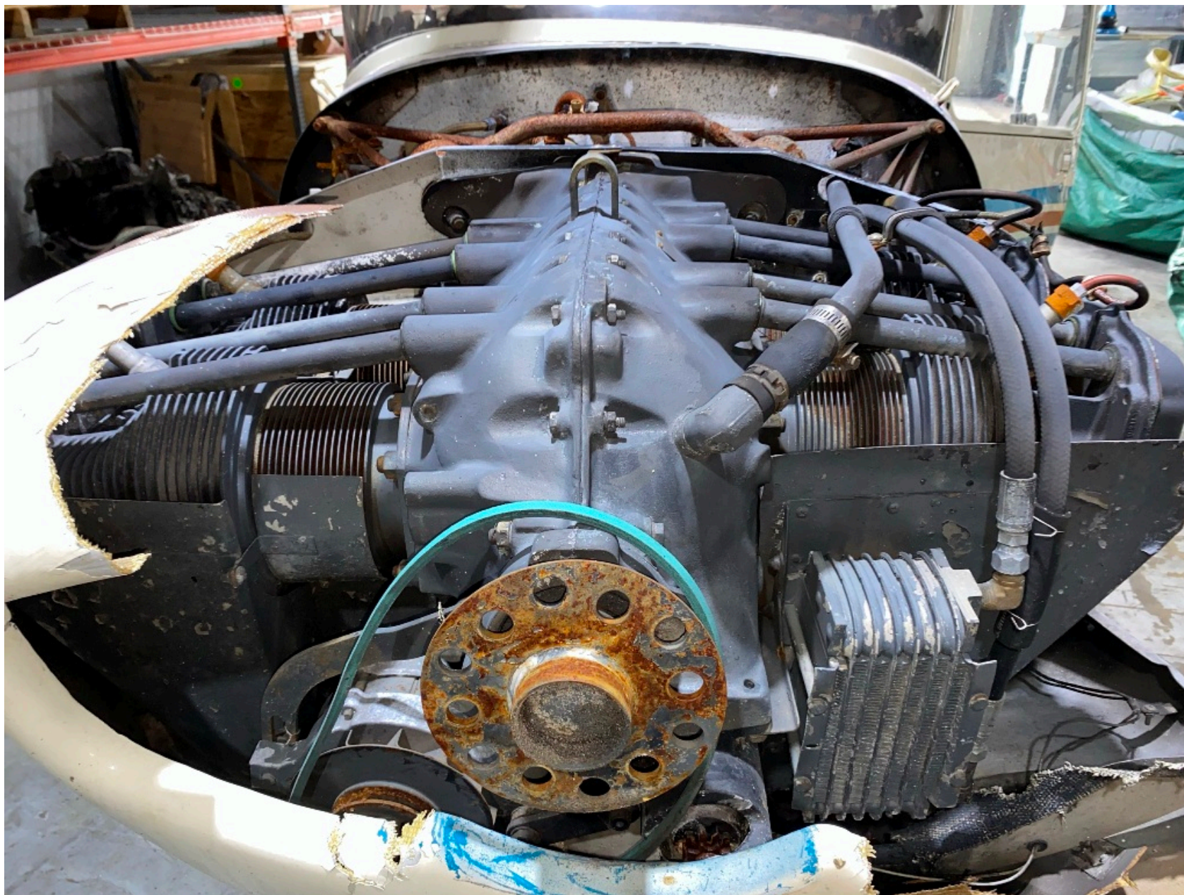
Photo 4 – Digital Photograph From Florida Air Recovery. Frontal View of the Engine Assembly Without Propeller Before Engine Postaccident Examination.
