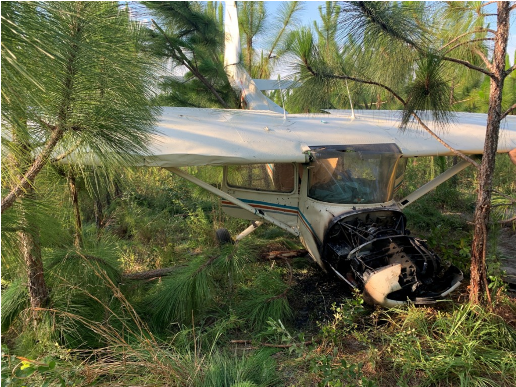
Photo 3 - Digital Photograph From Adam McCook. Forward View of the Airplane at The Accident Site. Note the Fire Damage in the Engine Compartment.
