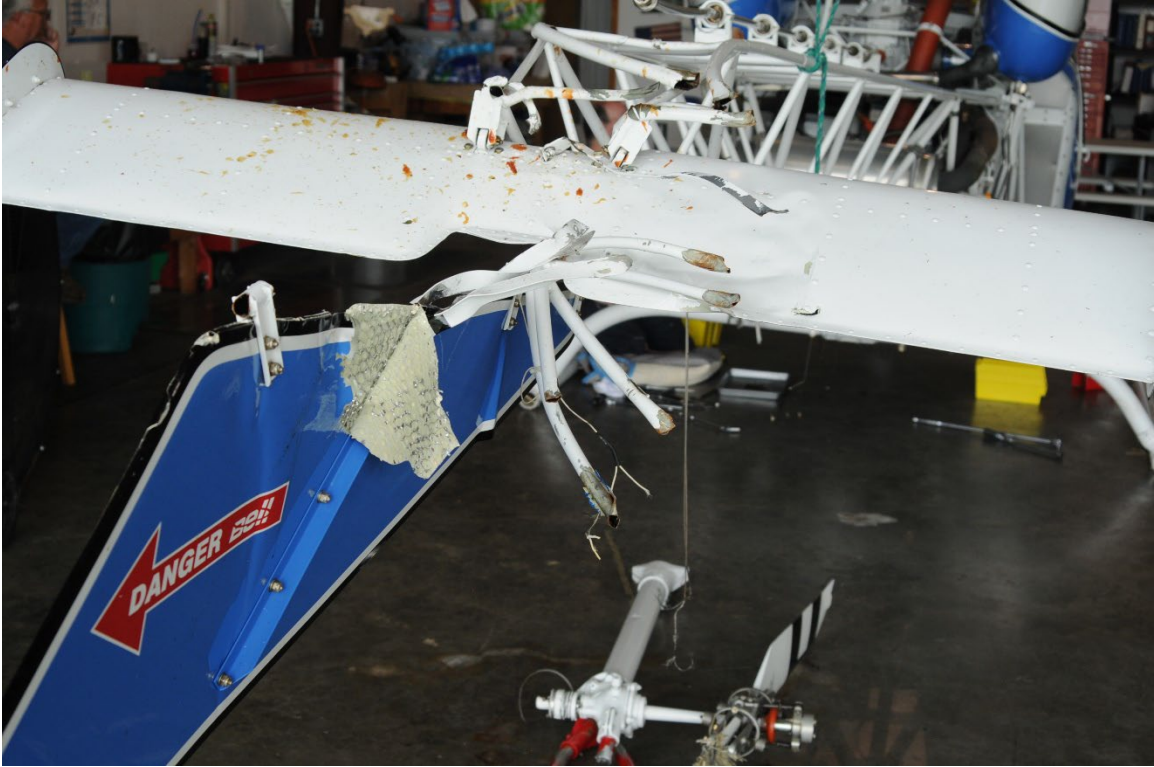
Photograph 4 – Accident helicopter – Post accident examination of tail rotor.
