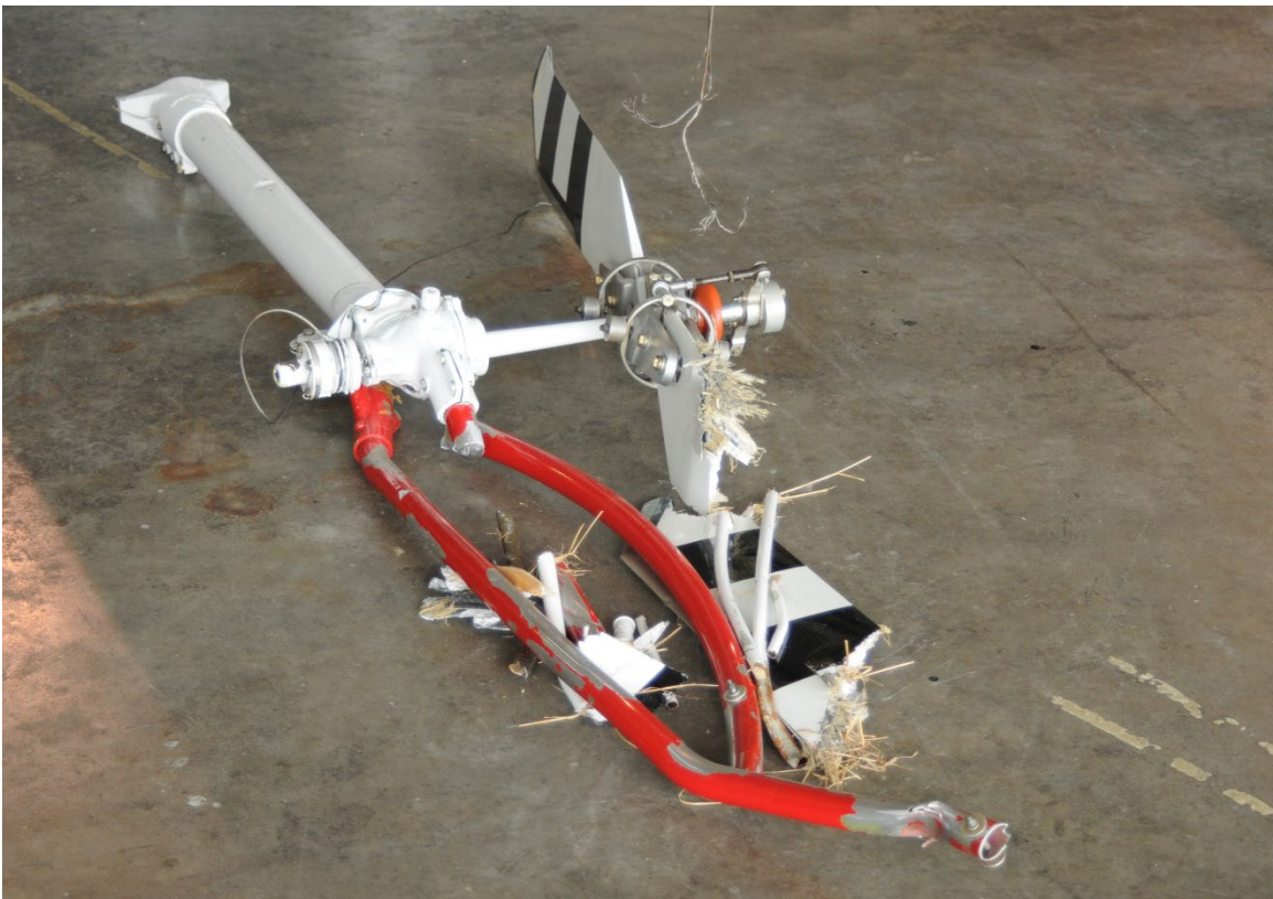
Photograph 5 – Accident helicopter – Post accident examination of tail rotor.
