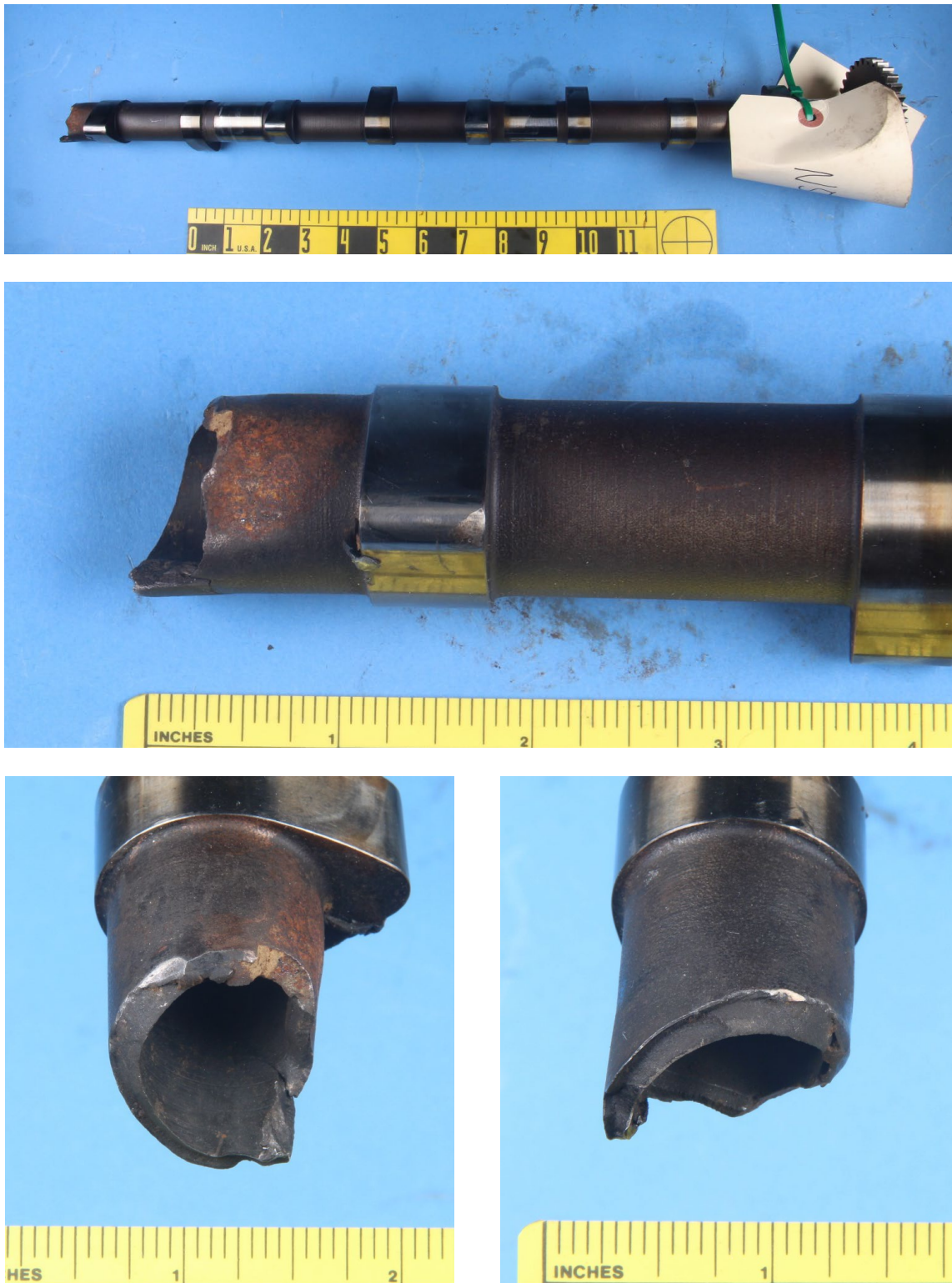
Figure 5: Overall and close-up photos showing the separated camshaft. The bottom two photos show the fracture surface adjacent to one cheek.
