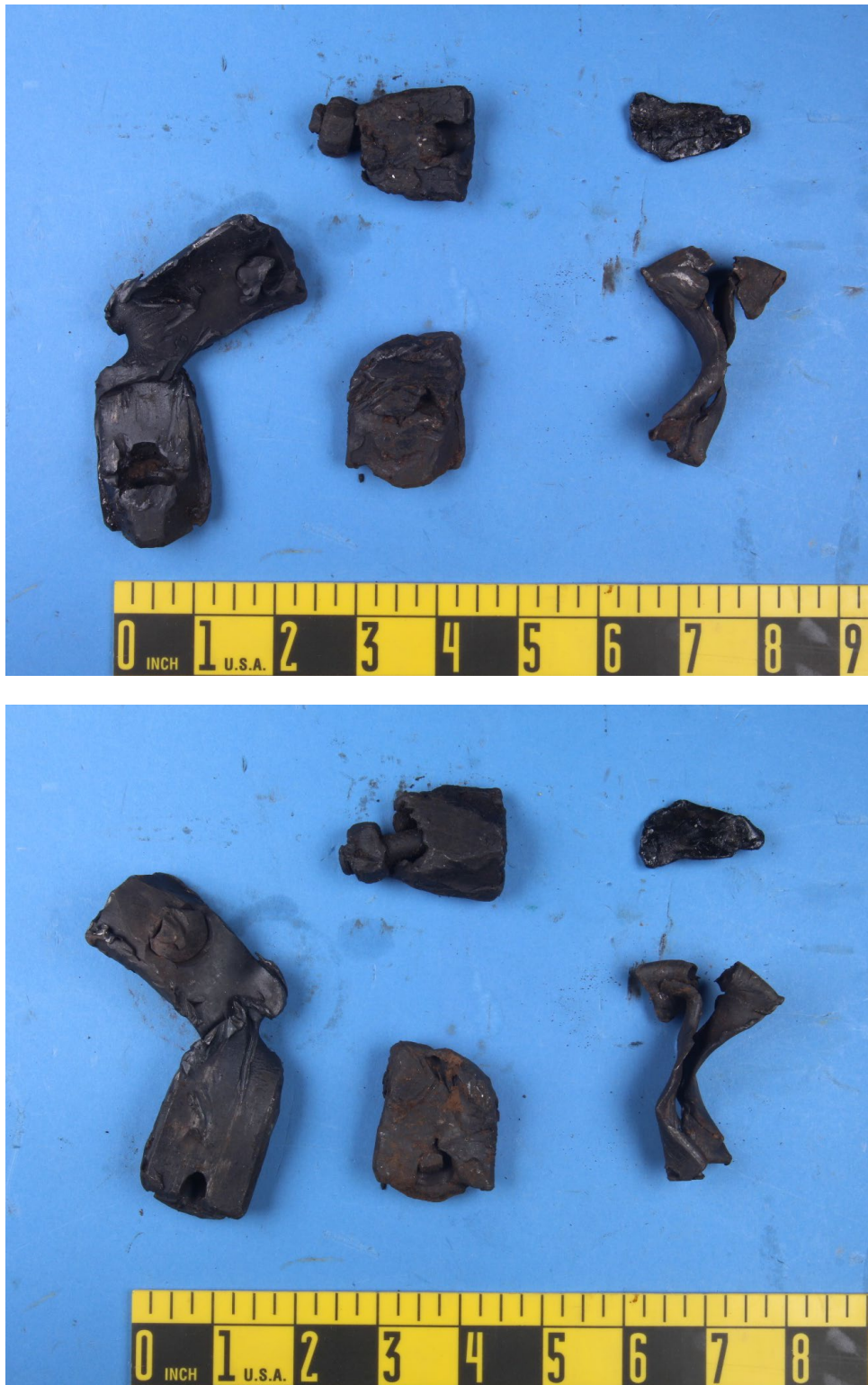
Figure 4: Overall photos showing the two sides of the connecting rod pieces.
