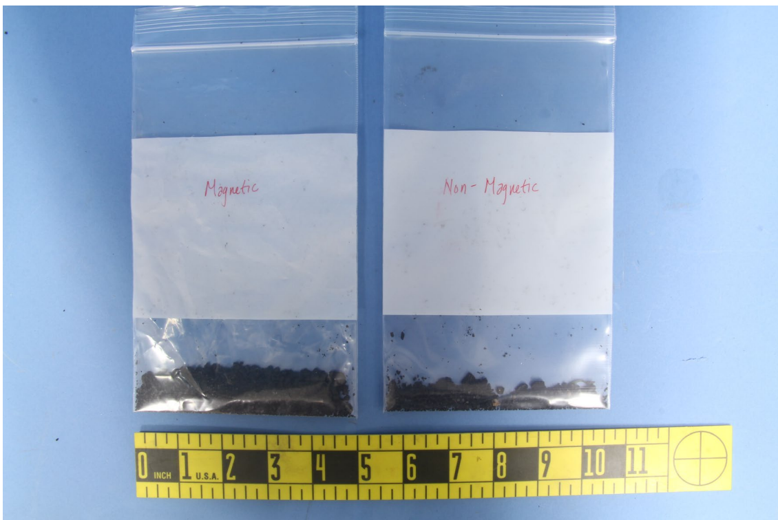
Figure 6: Overall photos of the oil suction screen debris (top) as-received and (bottom) after sorting using a magnet.
