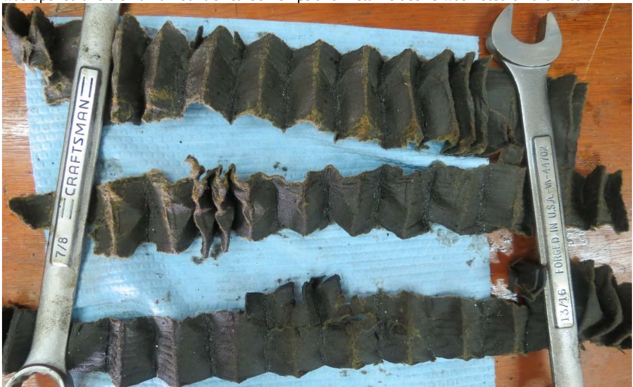
Figure 9. View of disassembled oil filter.
