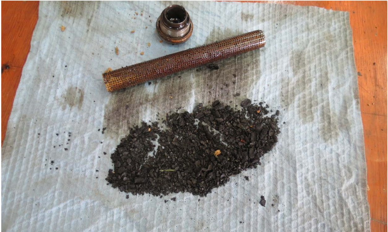
Figure 8. View of oil suction screen.
