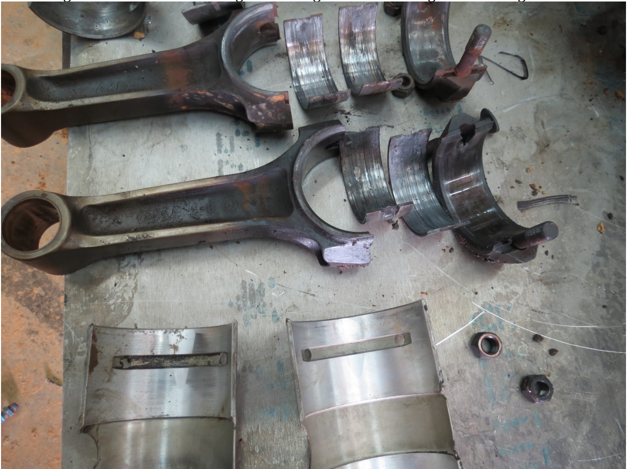
Figure 17. View of Nos. 1 and 2 connecting rods and bearings.
