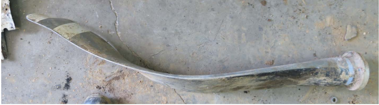
Figure 26. View of side of Blade A. Note bending.
