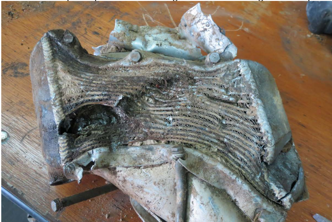
Figure 11. View of oil cooler as found.
