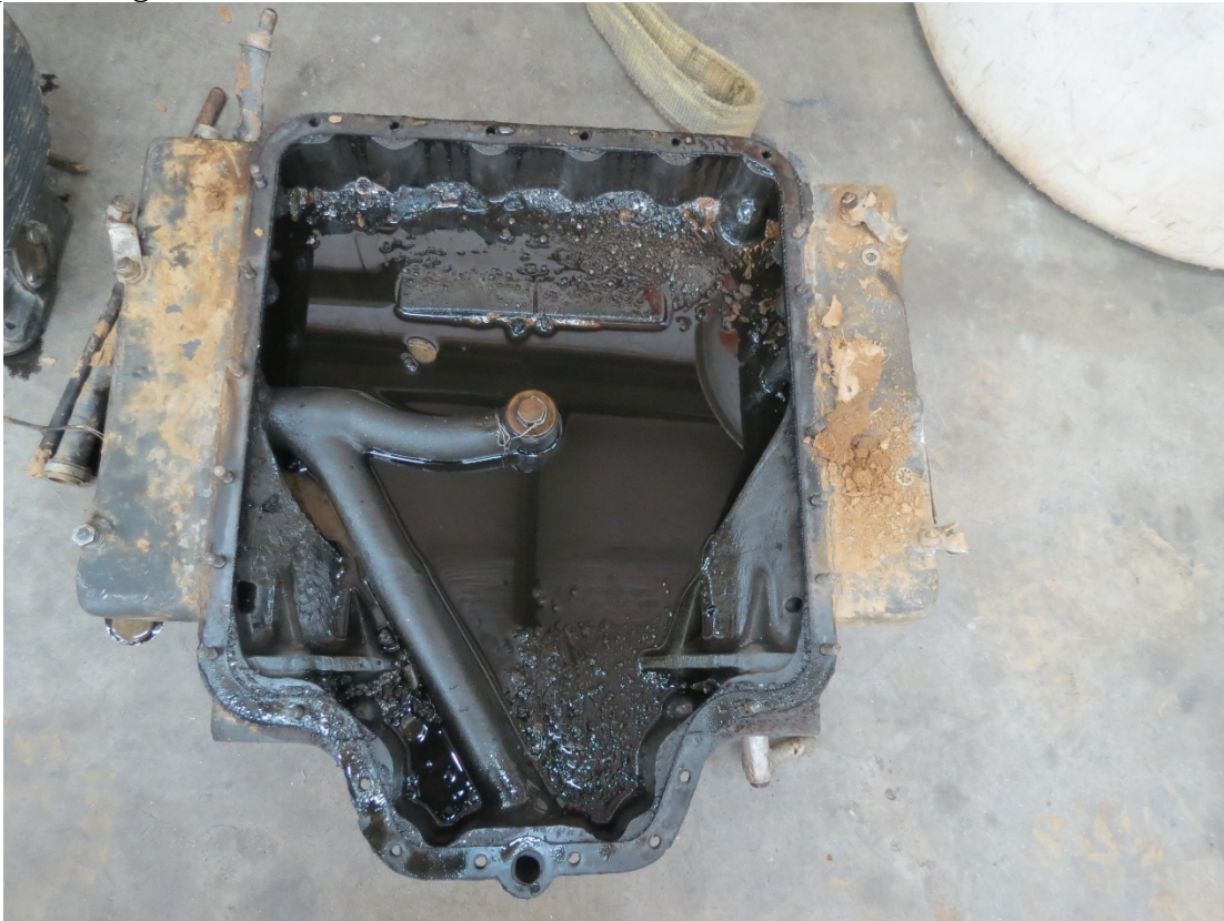
Figure 7. View of oil sump.
