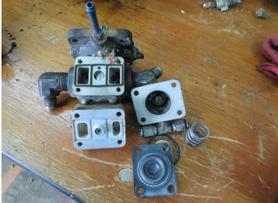
Figure 4. Disassembled fuel pump.
