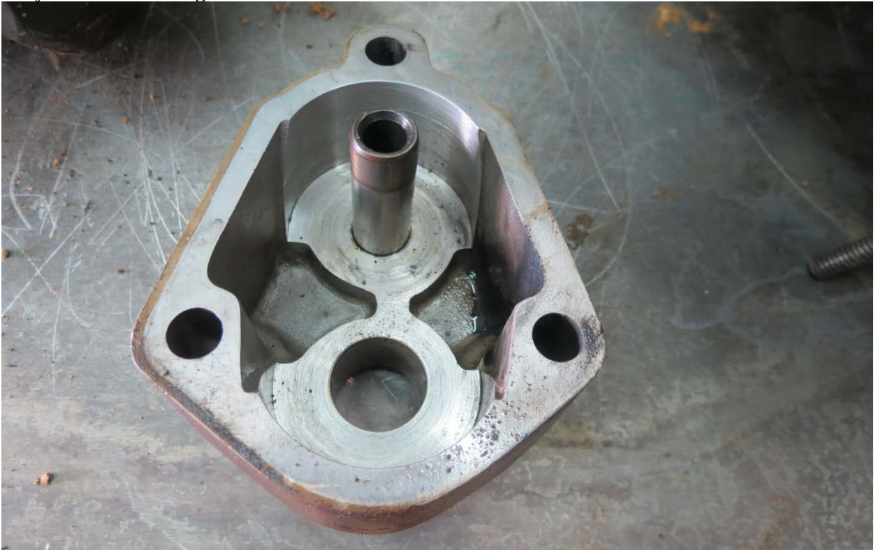
Figure 10. View of disassembled oil pump.
