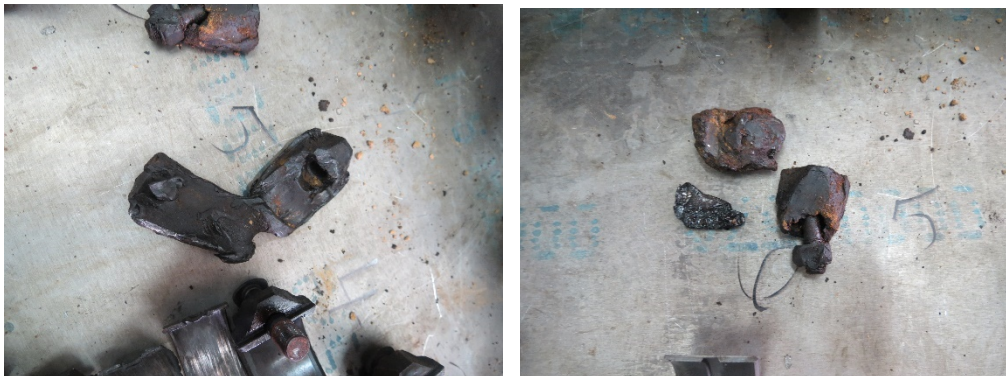
Figure 19. Nos 5 and 6 section of connecting rod.
