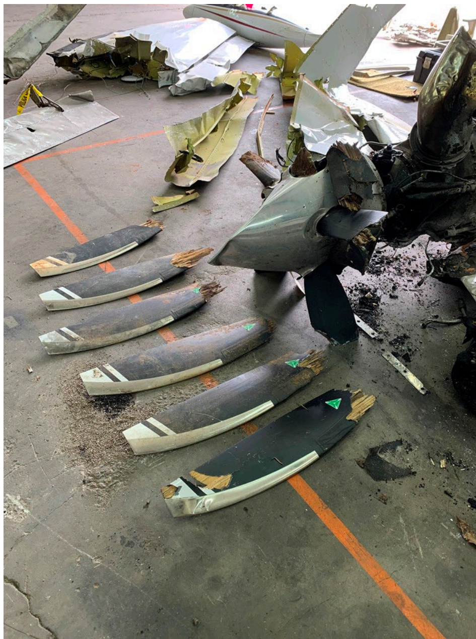
Photo 14 – Right Engine and Six Fractured Propeller Blades (NTSB)
