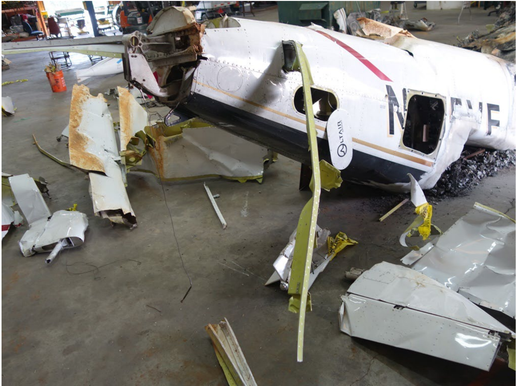
Photo 11 – Right Forward Horizontal Stabilizer Spar (PIPER)
