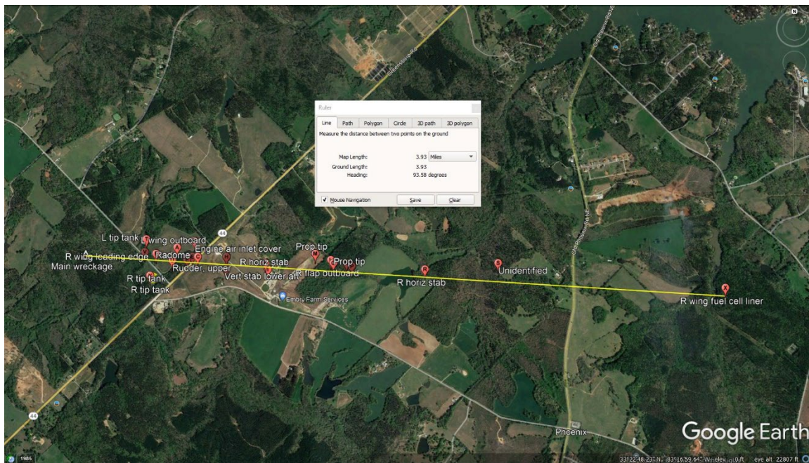
Figure 3. Google Earth image showing distribution of wreckage pieces. Furthest piece was about 3.9 miles east (about 094° true) from main wreckage.
