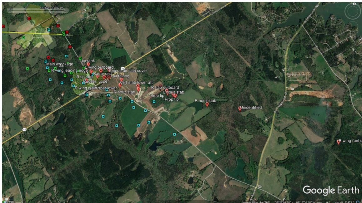
Figure 4. Orthomosaic in Google Earth showing the distribution of the wreckage pieces with regard to locations of radar returns.
