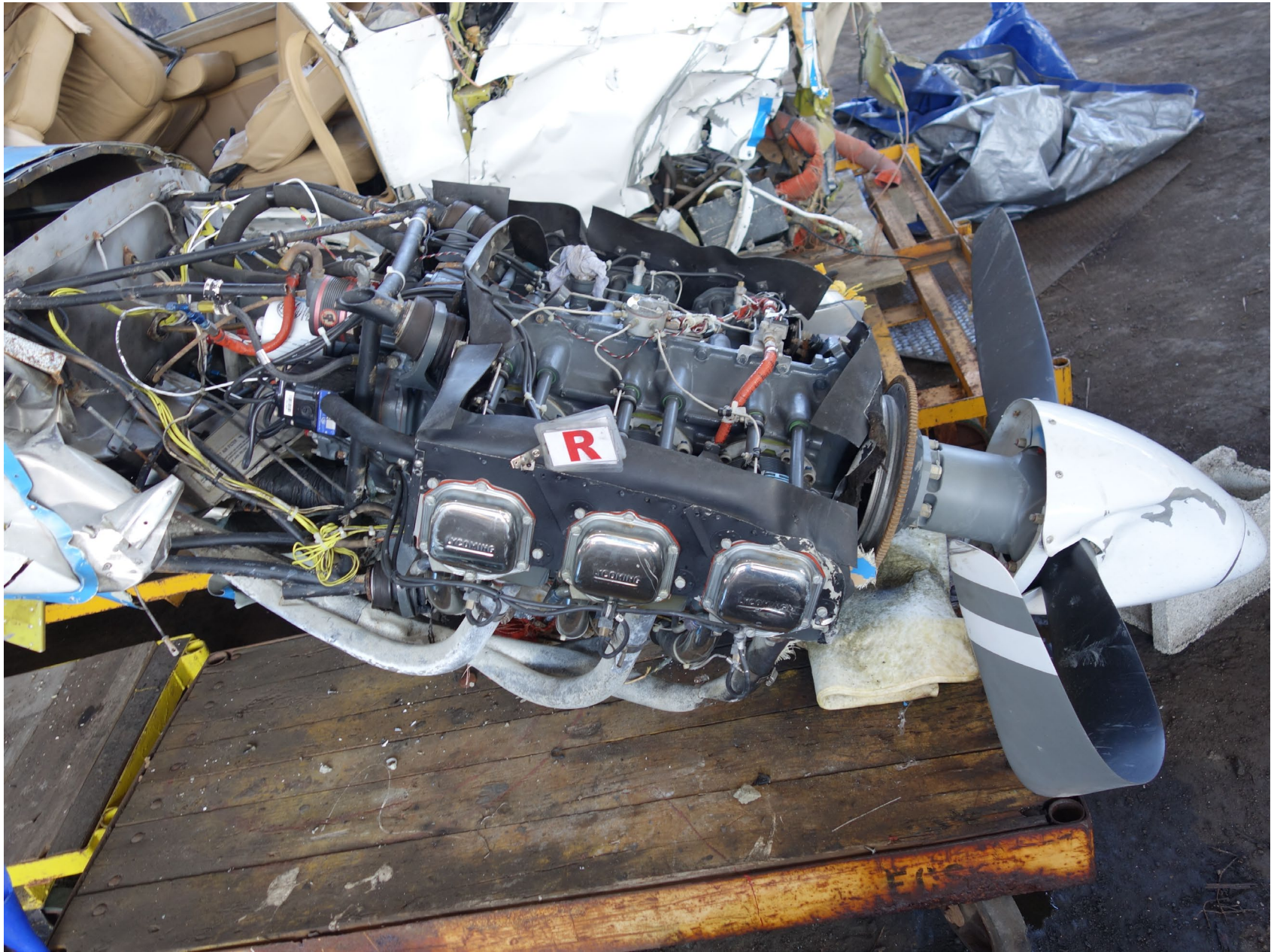
Photo 5 - Piper Digital Photograph. View of the Right Side of the Right Engine Assembly with Attached Propeller
