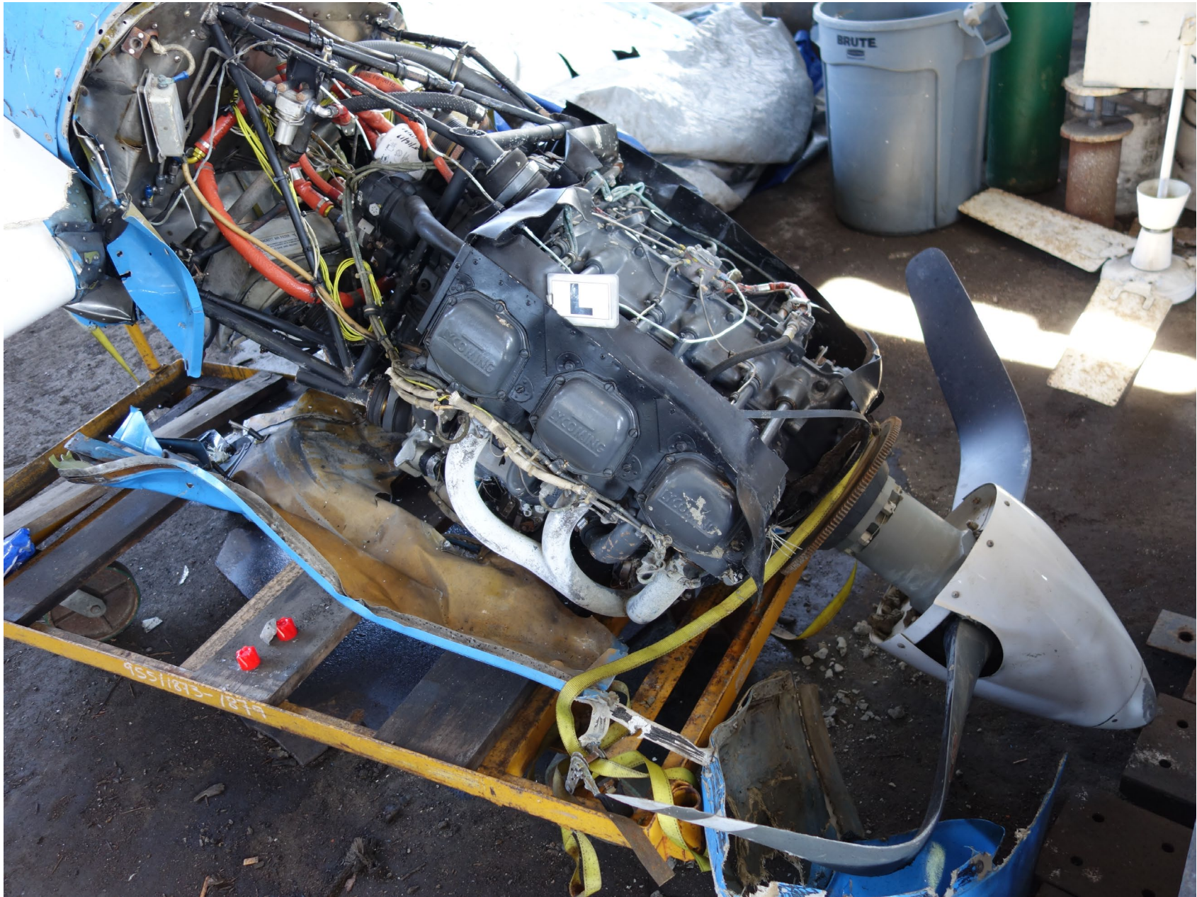
Photo 4 - Piper Digital Photograph. View of the Right Side of the Left Engine Assembly with Attached Propeller.
