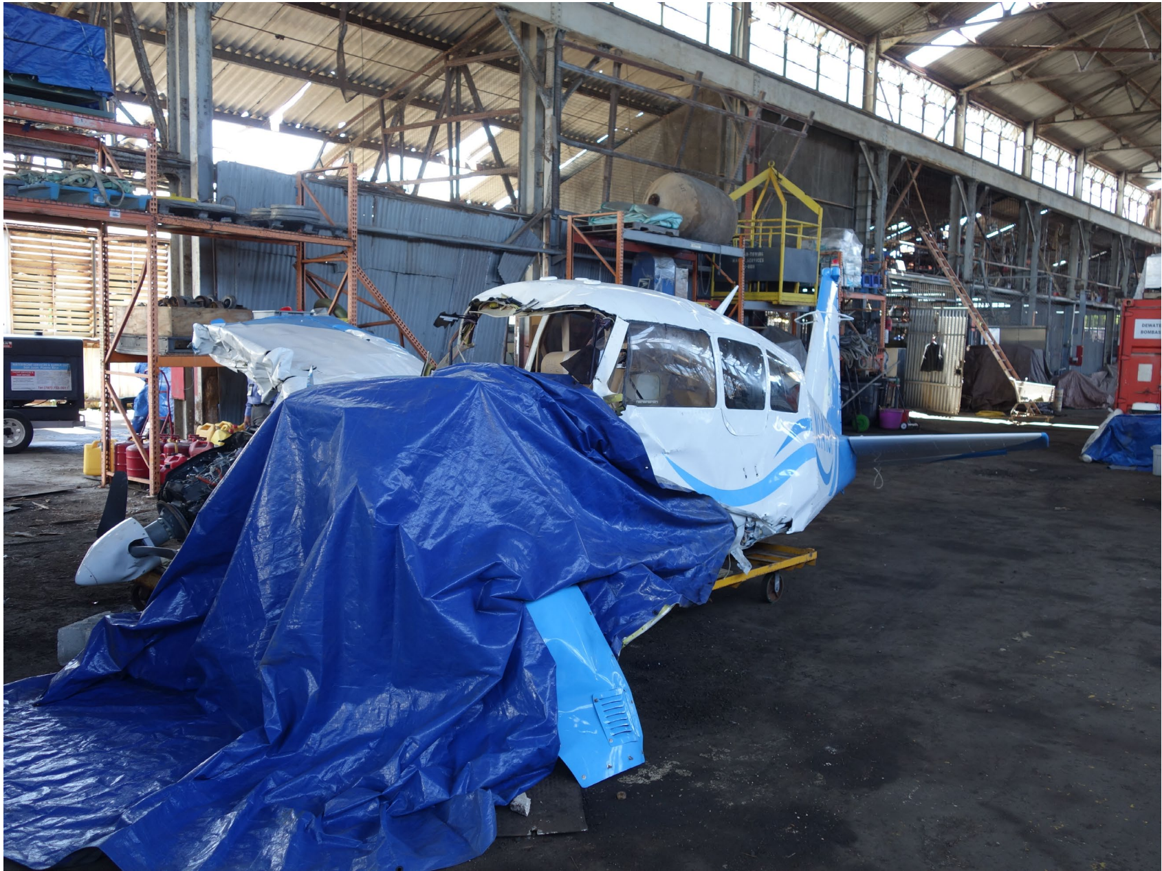
Photo 1 – Piper Digital Photograph. Left Side View of the Airplane Following Recovery. Note the Separated Left Wing.
