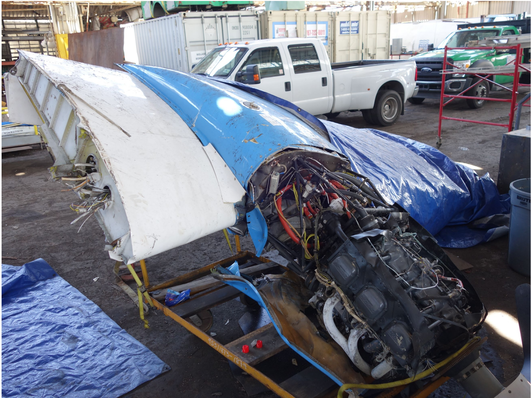
Photo 2 - Piper Digital Photograph. View of the Separated Left Wing with Attached Engine and Propeller Assembly.
