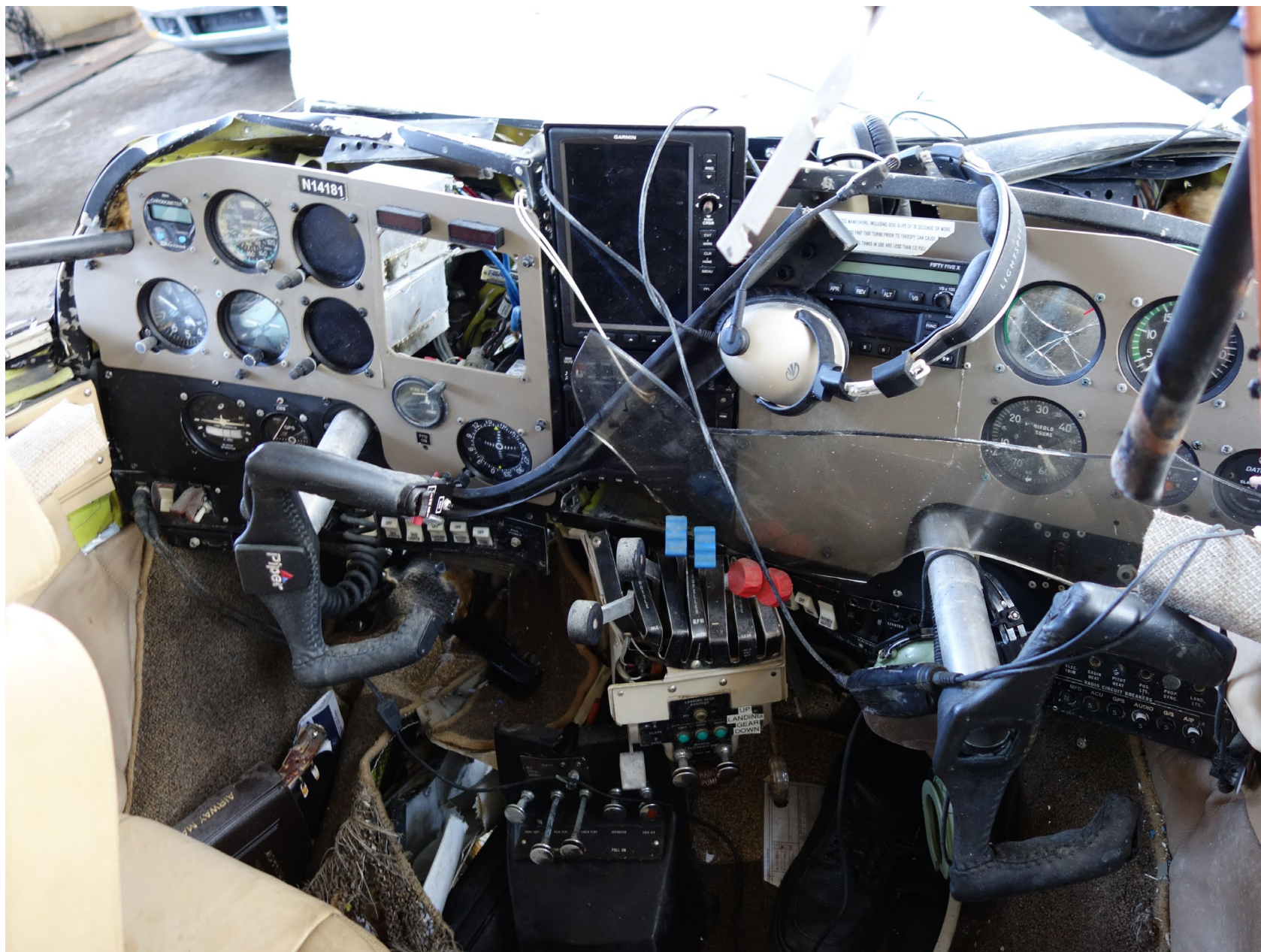
Photo 6 - Piper Digital Photograph. View of the Instrument Panel. Note the Positions of the Throttle, Propeller, and Mixture Controls.
