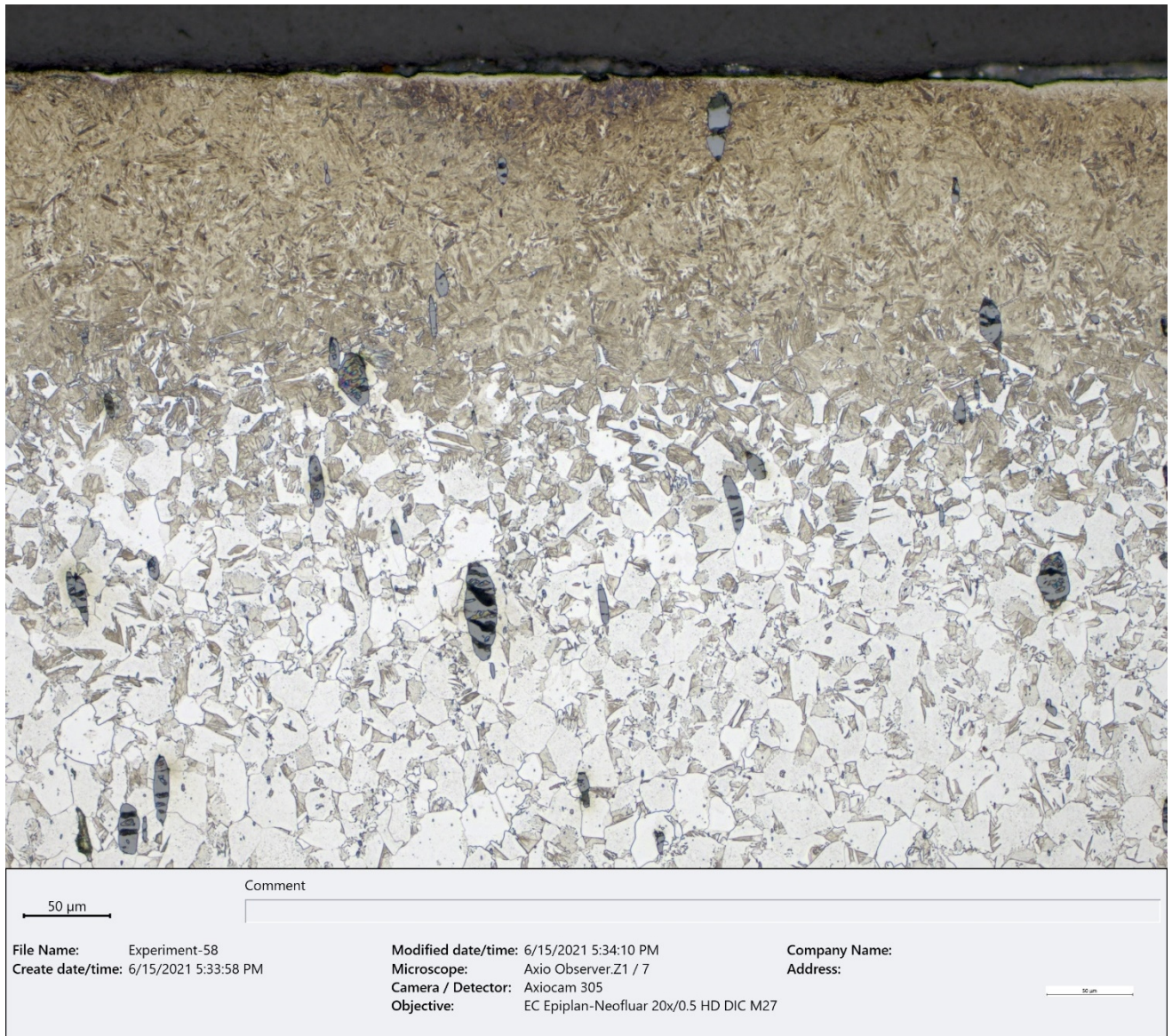
Figure 25 – Bright-field (BF) optical micrograph of a cross-section through the surface of the fractured ball screw remnant. The darker areas were the carburized surface, with the core microstructure below (~200X, etched 2% Nital).
