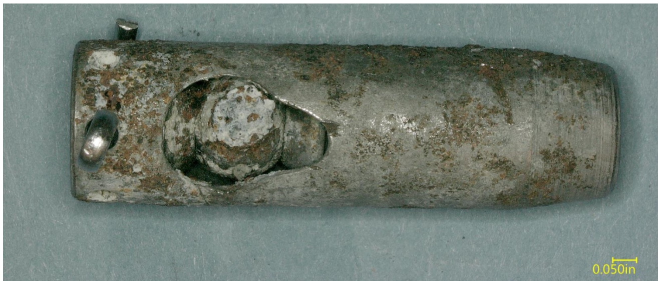
Figure 16 – View of the ball joint assembly remnant and the ball screw neck fracture surface, as received.
