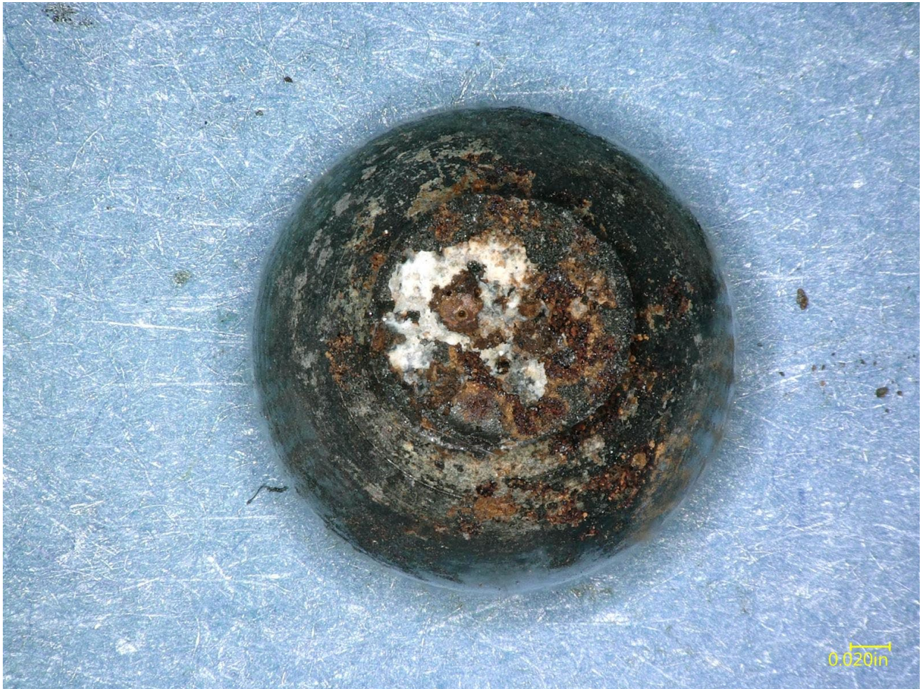
Figure 20 – View of the ball screw neck fracture surface from the head side, after cleaning.
