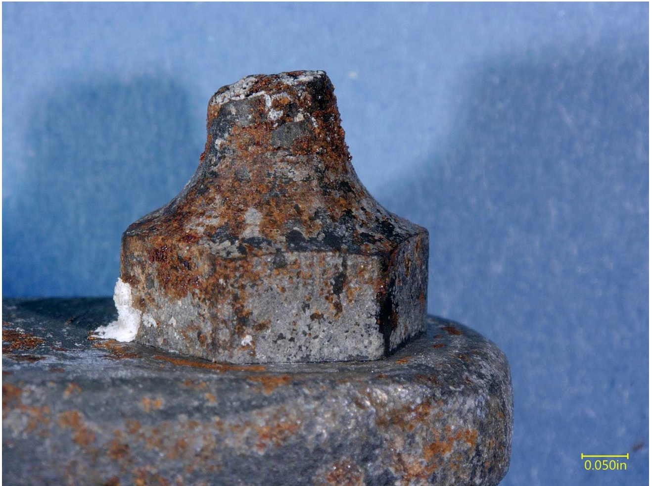
Figure 4 – Side view of the fracture surface of the ball screw remnant, still connected to the throttle lever, as received.
