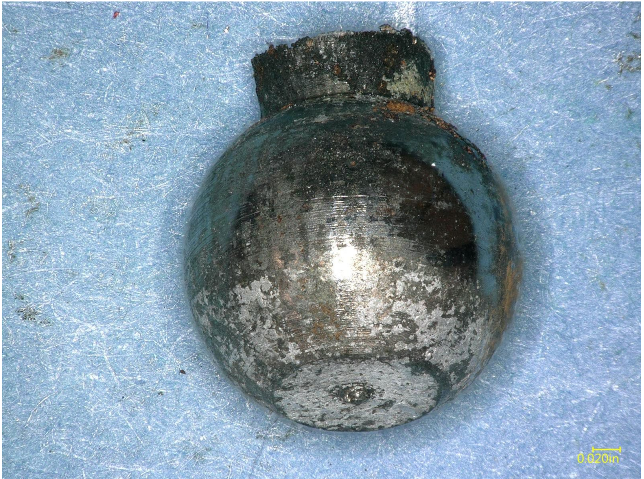
Figure 19 – Closer view of the head and fractured neck of the ball screw remnant from Figure 18, viewed from the side.
