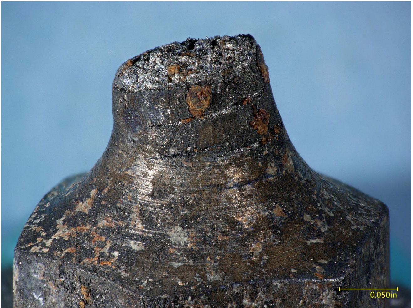
Figure 5 – The ball screw neck fracture from Figure 4, after cleaning, showing parallel secondary cracks and a general deformation of the neck.
