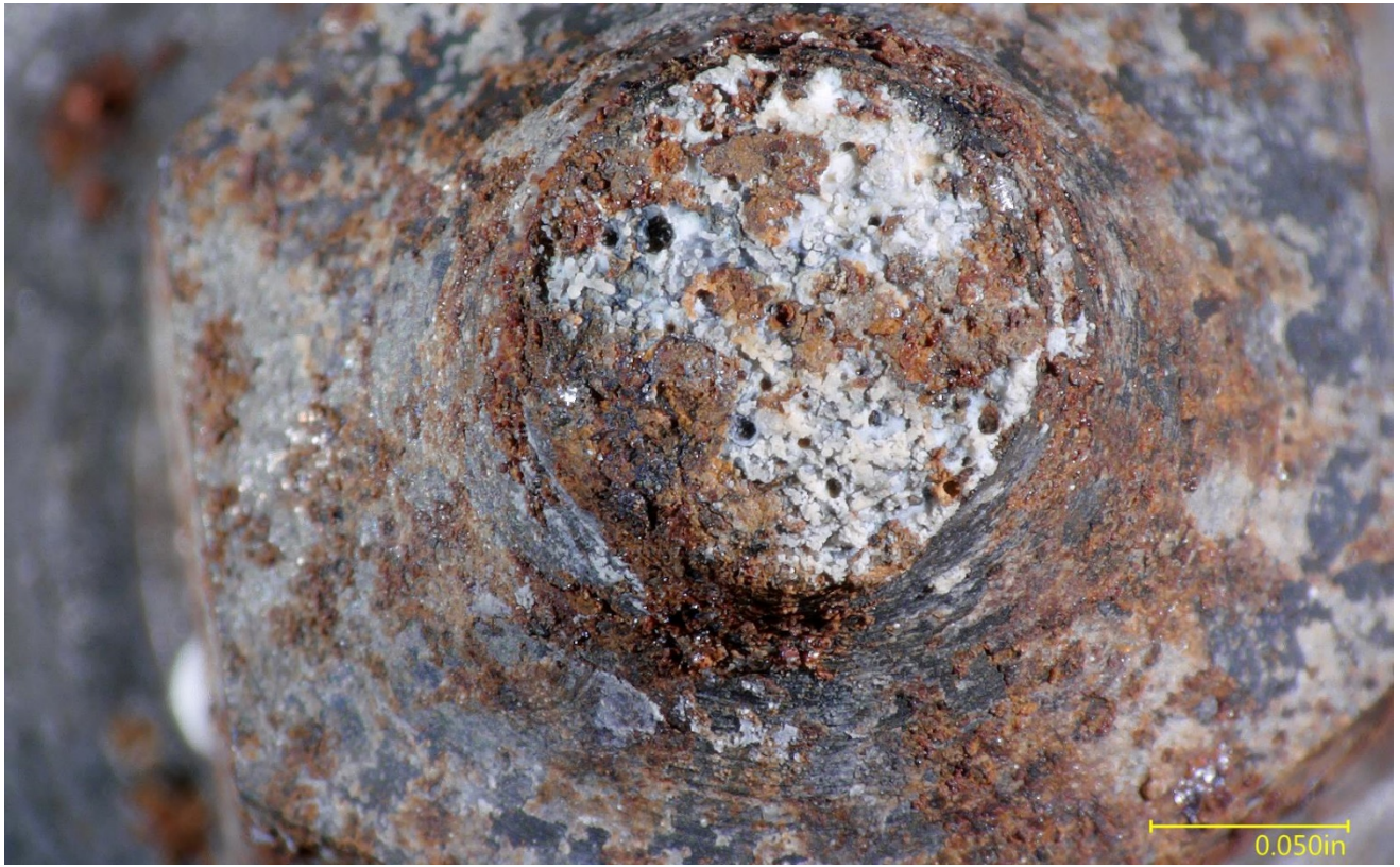
Figure 6 – View of the fracture surface of the ball screw neck from the throttle lever side, as received.
