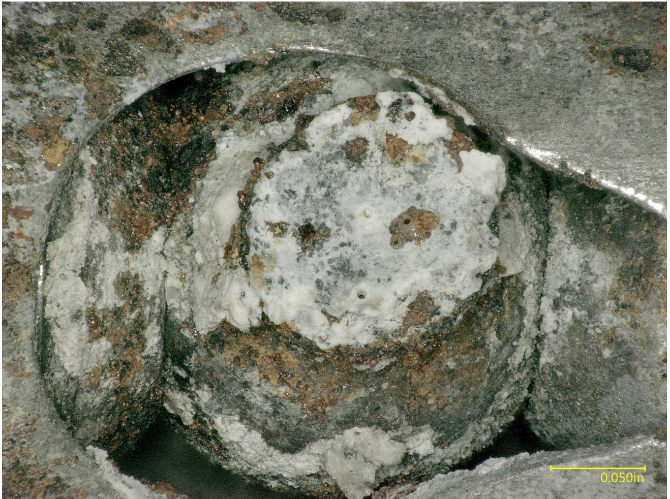
Figure 17 – Closer view of the ball screw neck remnant fracture surface, as received.
