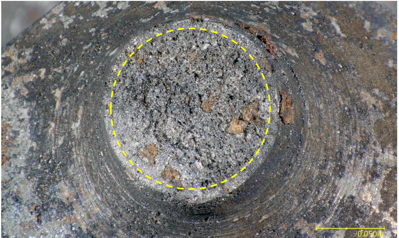
Figure 7 – View of the throttle lever side ball screw neck fracture surface, after cleaning. The dashed oval represents the different fracture regions on the surface.
