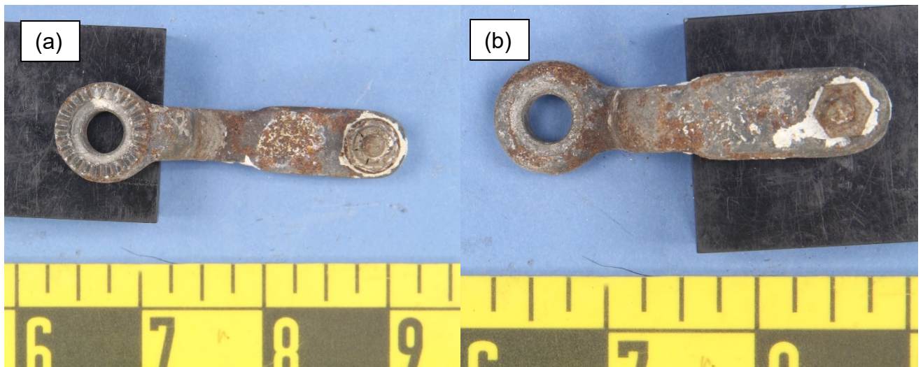
Figure 2 – The throttle lever, viewed from (a) the face with the threaded portion of the ball screw with the nut, and (b) the face with the fractured ball screw neck.
