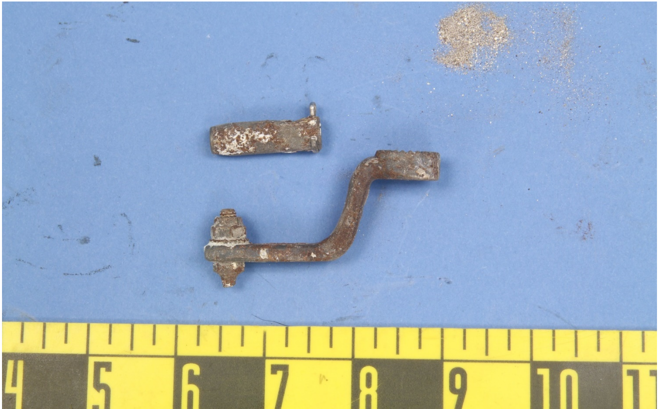
Figure 1 – The pieces from the throttle connection, as received. Also included was an amount of dust and sand debris.
