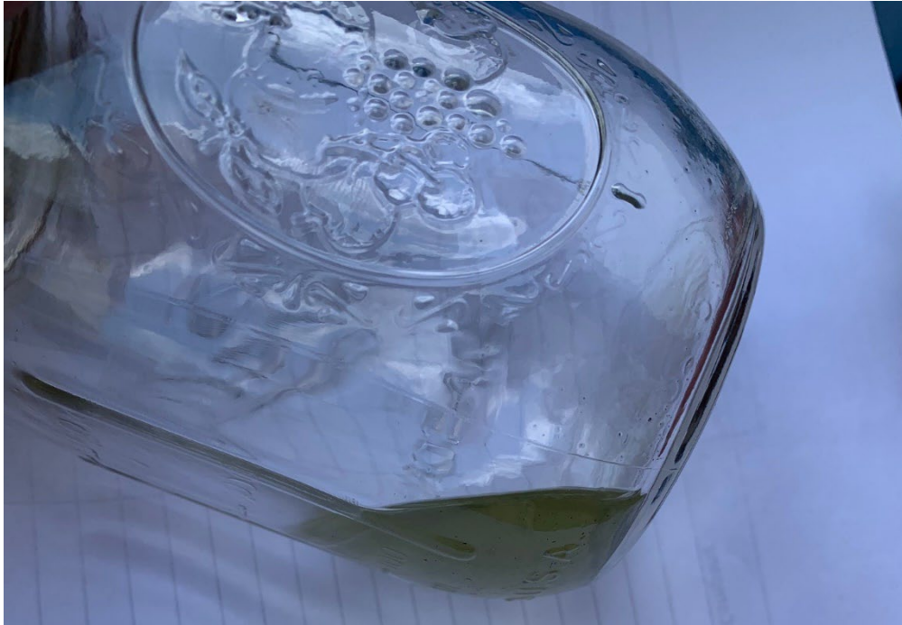
Photograph 1 – Fuel sample #1 – obtained from carburetor bowl.
