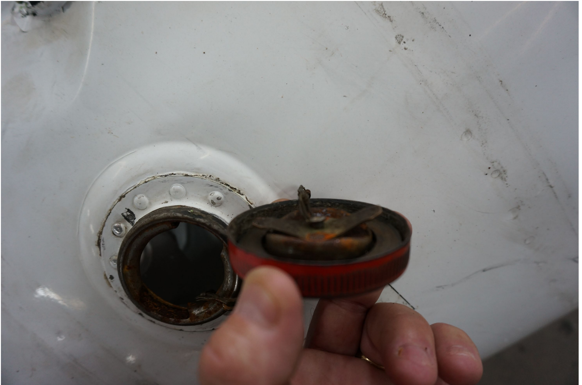
Photo 14 - Inside of Fuel Cap (Side View of Locking Mechanism)
