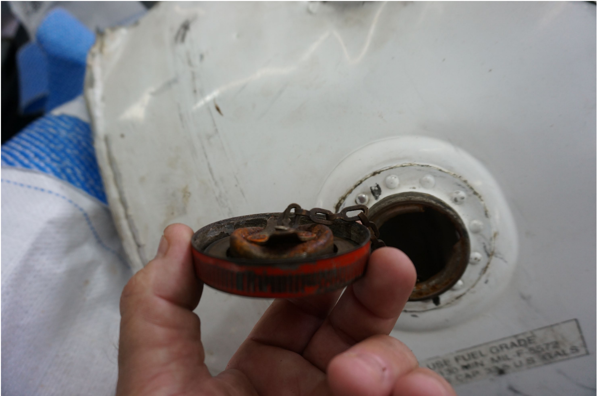
Photo 15 – Inside of Fuel Cap (End View of Locking Mechanism)
