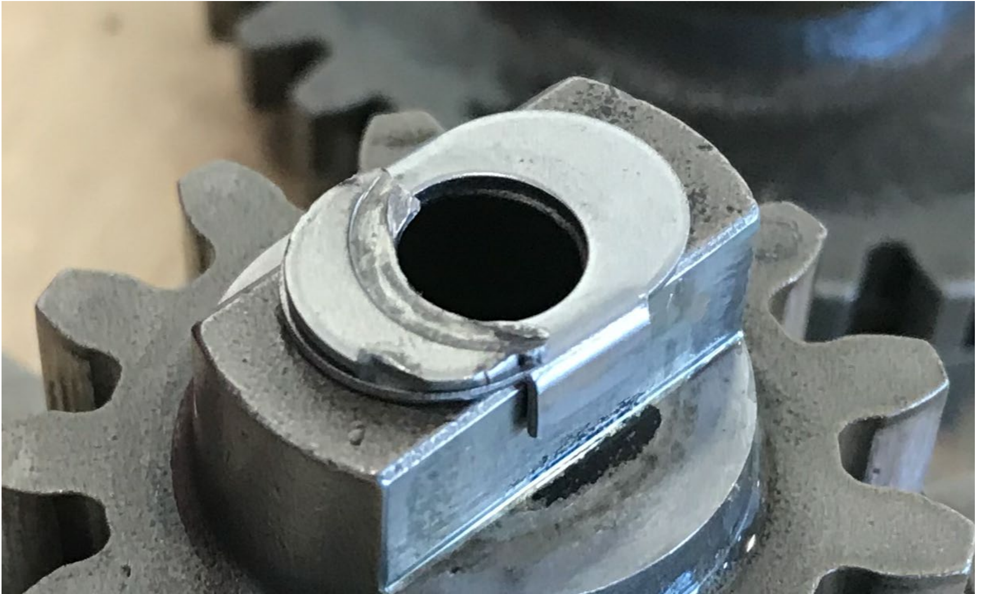
Photo 7 - FAA Digital Photograph. View of the Crankshaft Gear, Exemplar Lockplate on the Bottom and Accident Lockplate on top. The FAA inspector Reported the Profile of the Accident Lockplate Matched the Un-Bent Profile of the Exemplar Lockplate.
