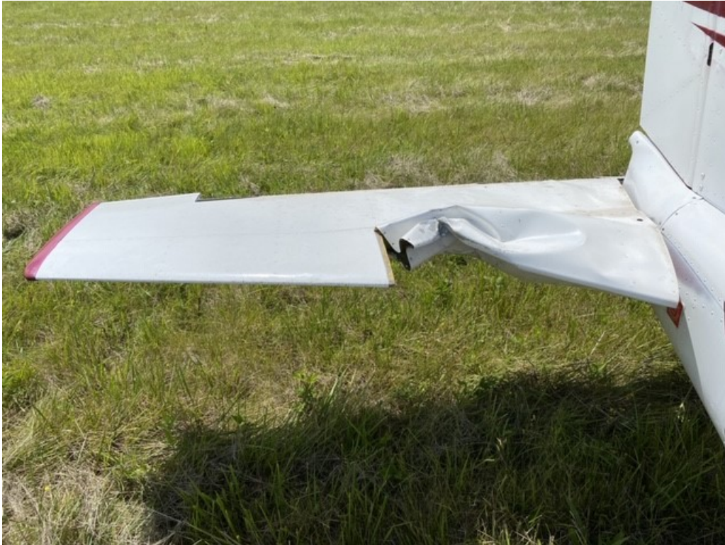
Figure 1: Photograph Provided by Victor Yore. View Depicting the Damage to The Right Horizontal Stabilator.
