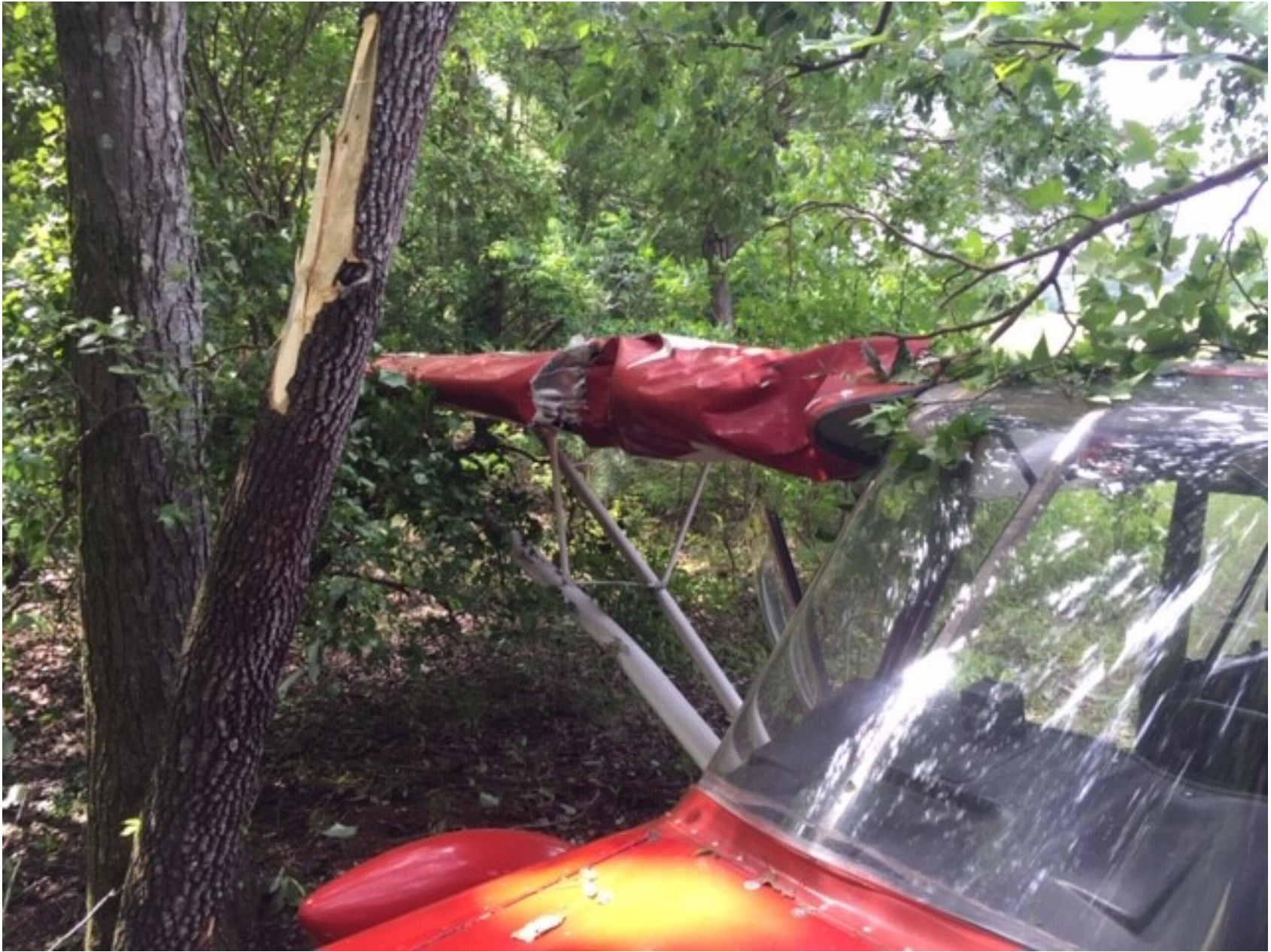
Photo 2 – View of right wing showing buckling damage
