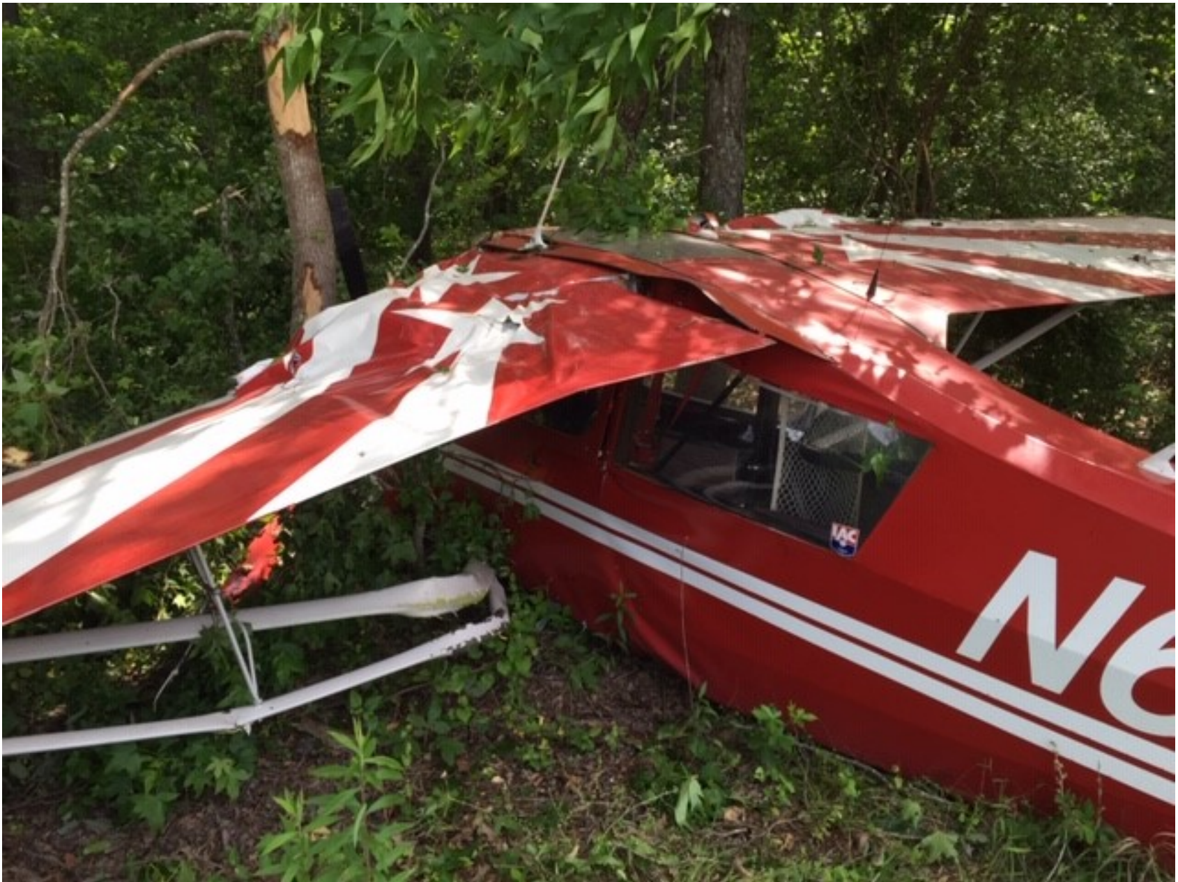
Photo 1 – View of airplane from left side showing left wing damage
