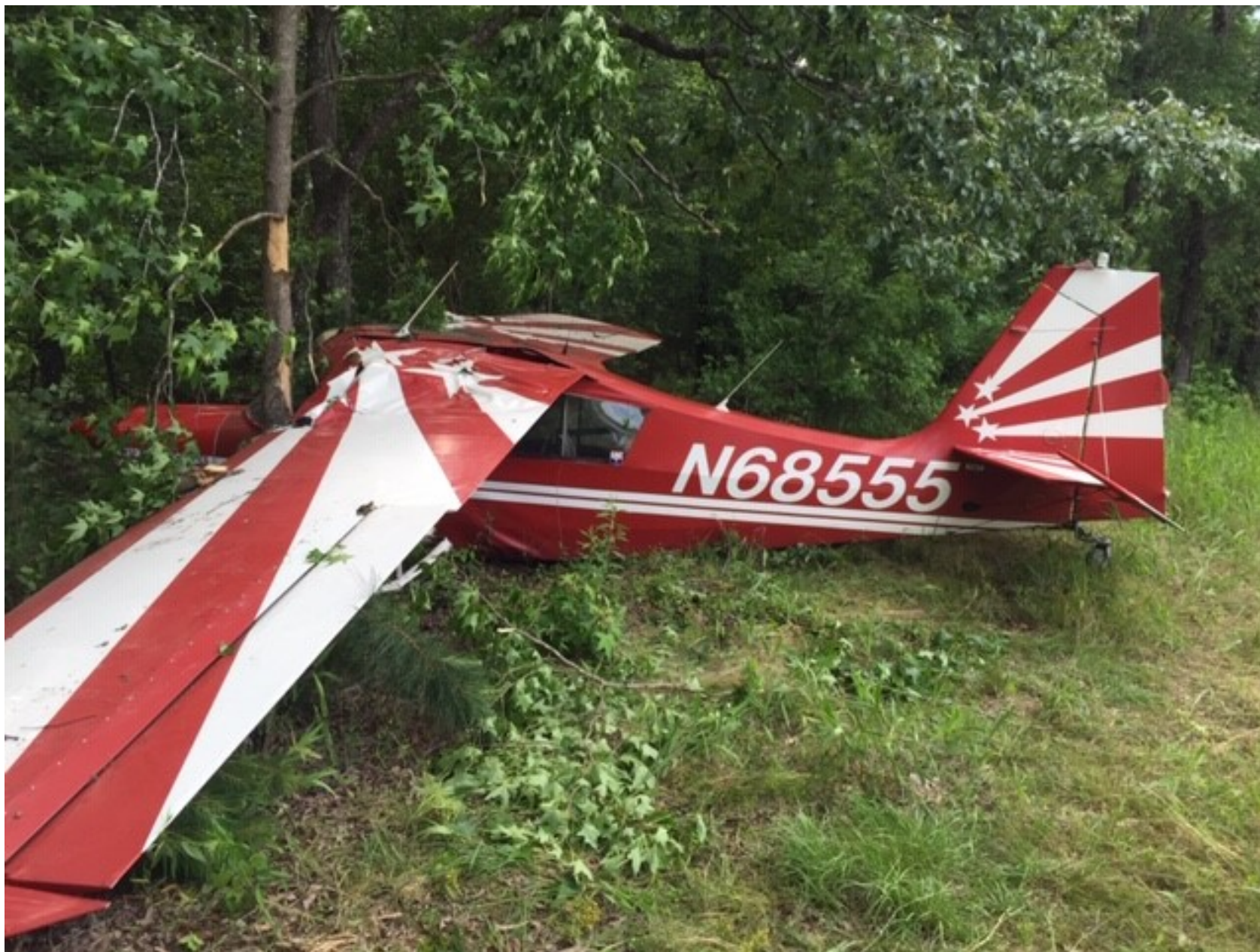
Photo 3 – View of left side of fuselage showing buckling damage
