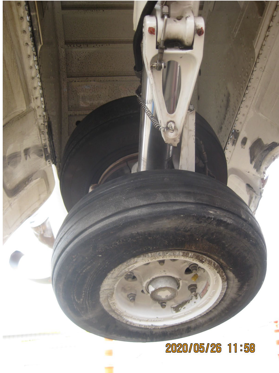
Photo 5 – Left landing gear fractured scissors. (Courtesy of FAA)
