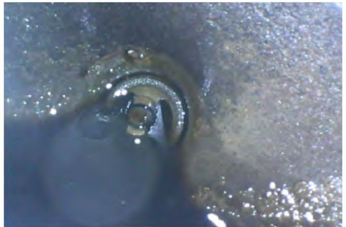
#5 Bottom Spark Plug (submerged in oil)
