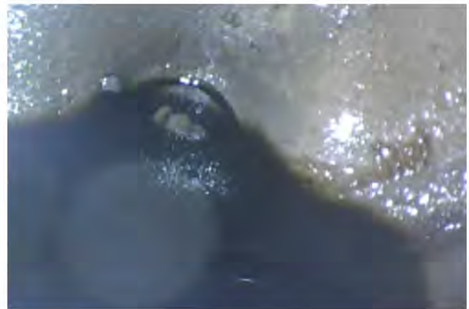
#1 Bottom Spark Plug (submerged in oil)
