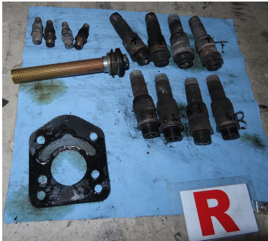
Photograph #5 – Right engine spark plugs, injectors, and oil screen.
