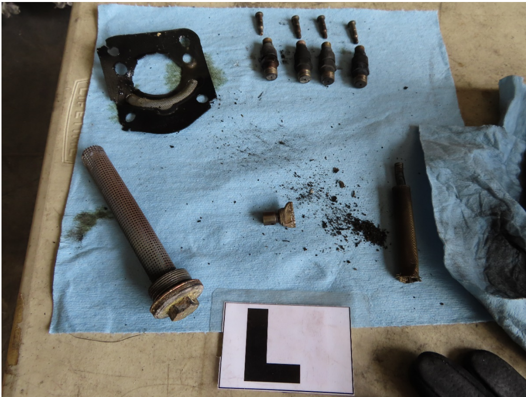
Photograph #3 – Left engine injectors and oil screen.
