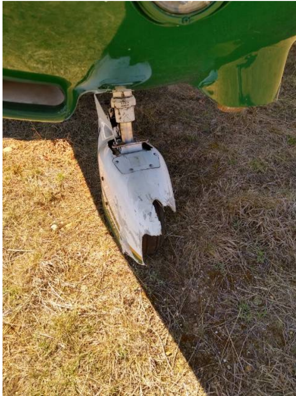
Photo 1 – Nose Landing Gear – Courtesy of Town of East Hampton
