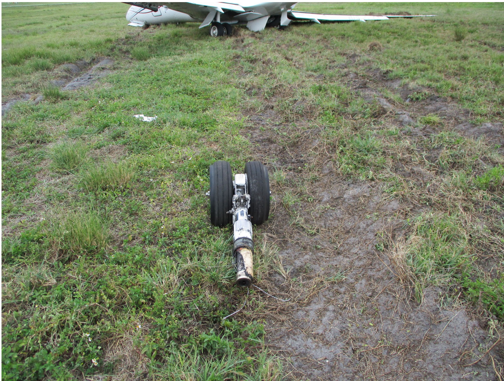
Photo 7 – Nose Landing Gear (FAA Photo)
