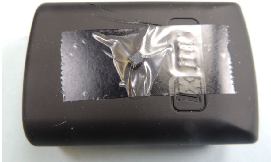
Figure 1. The LXNav Nano with impact damage.
