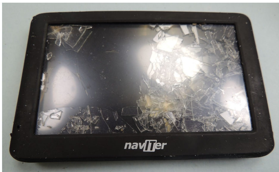
Figure 2. The Naviter Oudie shown with impact damage.
