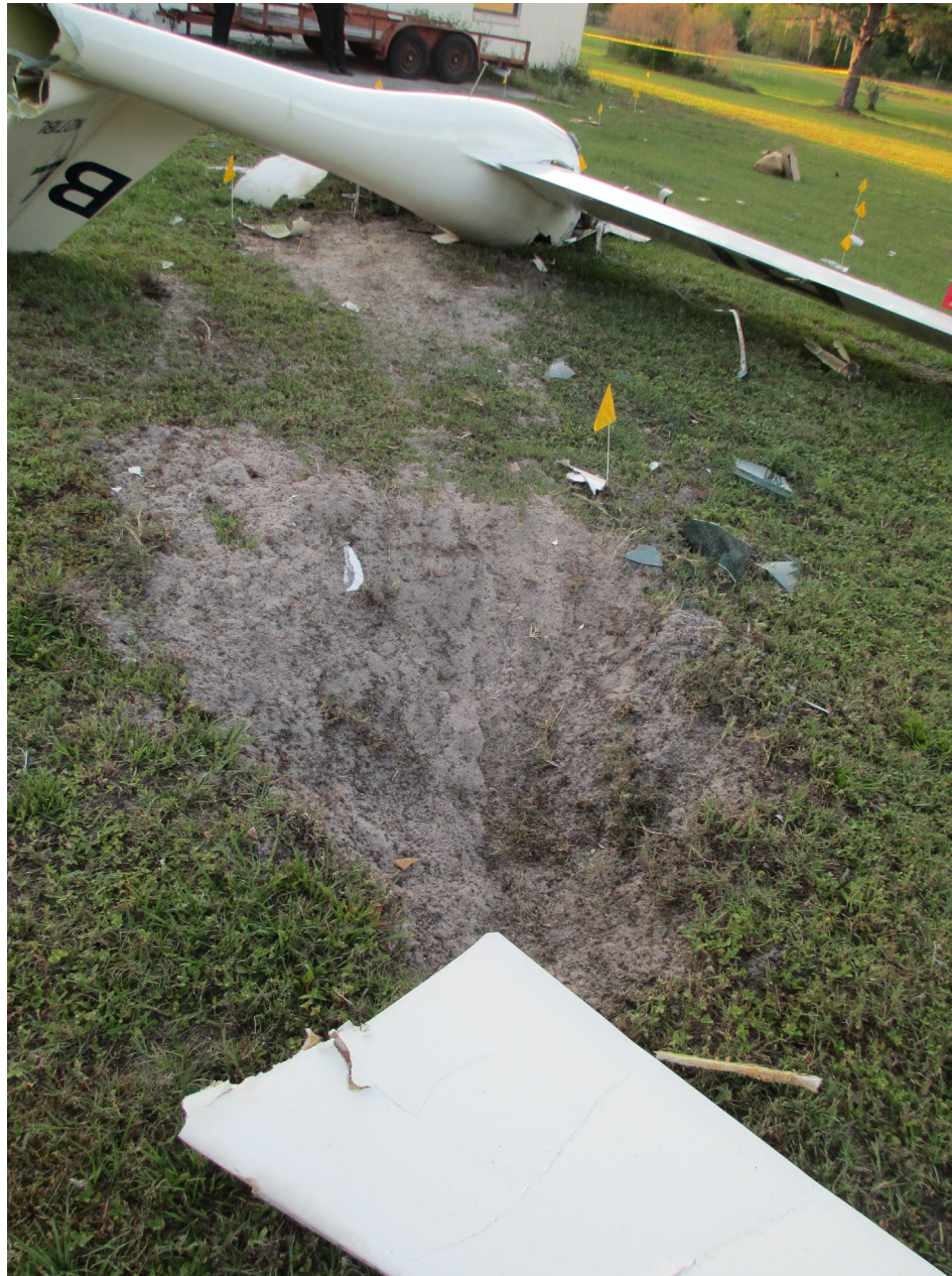
Photo 1 – View of Initial Ground Scar and Main Wreckage (FAA)
