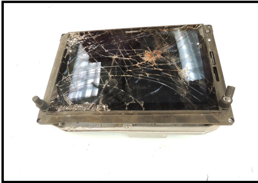
Figure 1. Damaged exterior of damaged EFIS.
