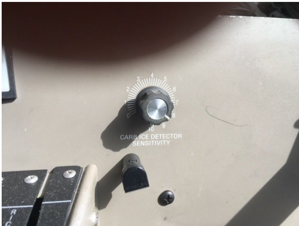
Photograph 6 – Accident airplane – Cockpit instrument panel (Carb Ice sensitivity control). (Photo provided Beverly Flight Center).
