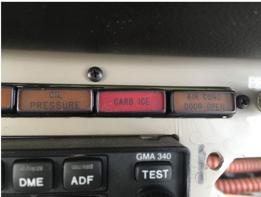
Photograph 5 – Accident airplane – Cockpit instrument panel (Carb Ice light). (Photo provided Beverly Flight Center).
