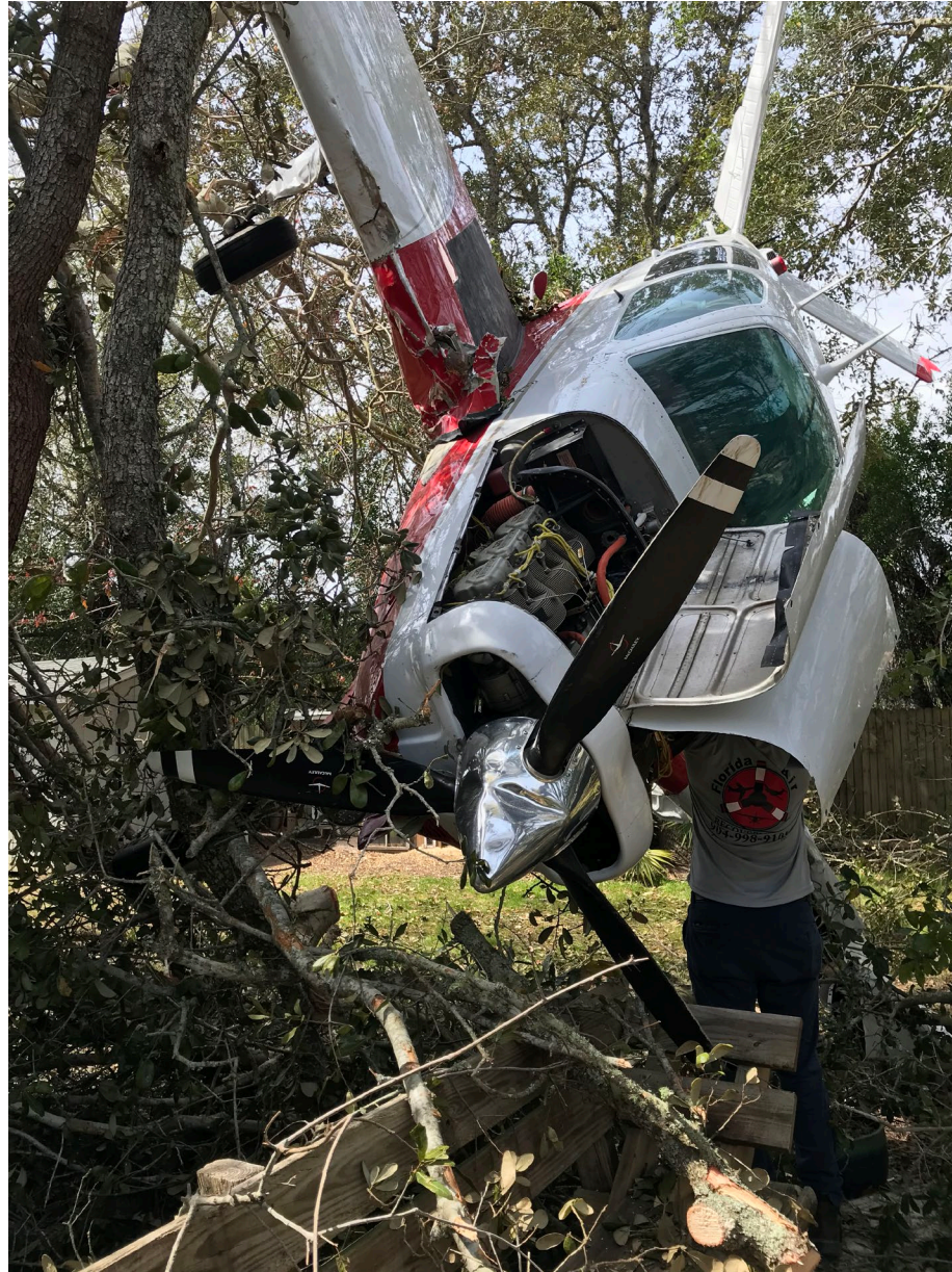
Photo 1 – View of airplane wreckage resting in tree. Note right wing damage. (Courtesy of FAA)
