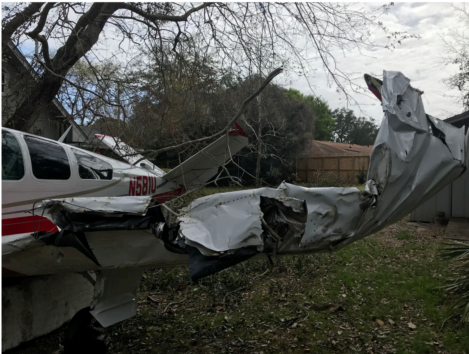
Photo 2 –Closeup view of severely deformed left wing. (Courtesy of FAA)
