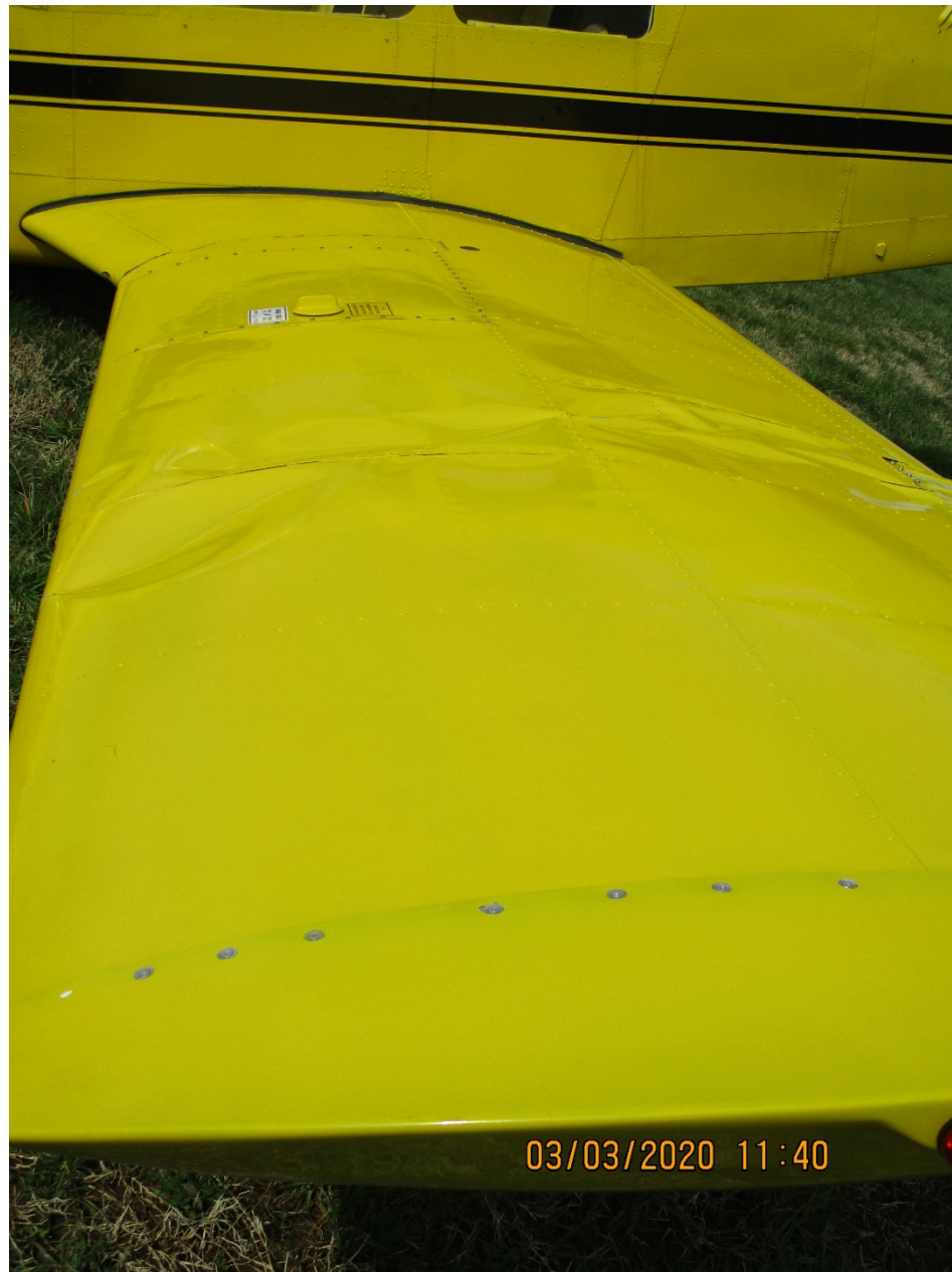
Photo 5 – View of Left Wing Damage (Photo Courtesy of FAA)
