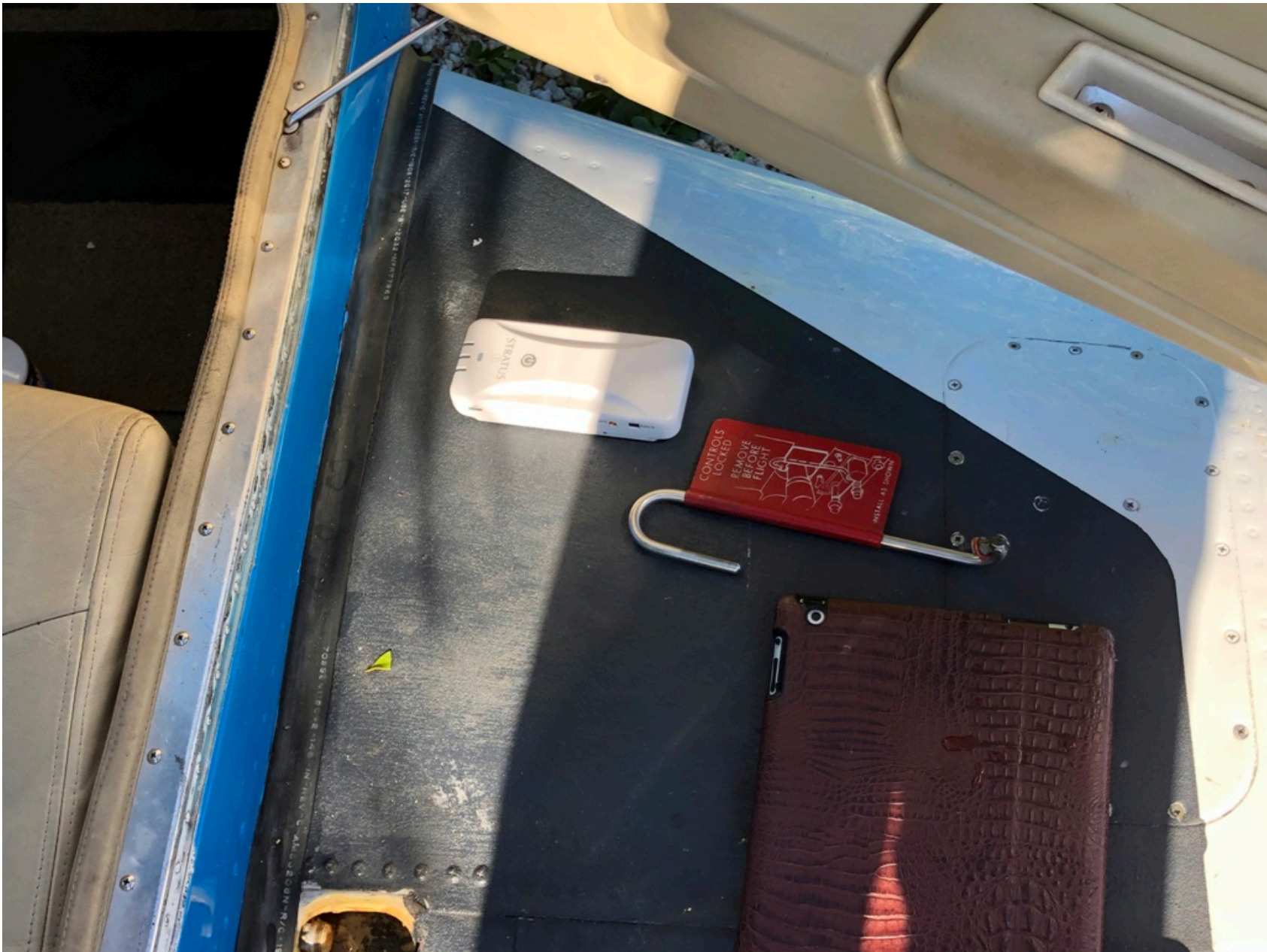
Photo 5 - Digital Photograph From Airport Manager. Photograph taken at 1547 EST. View Depicts the As-Observed Position of the Gust Control Lock About 12 Minutes after the Accident.
