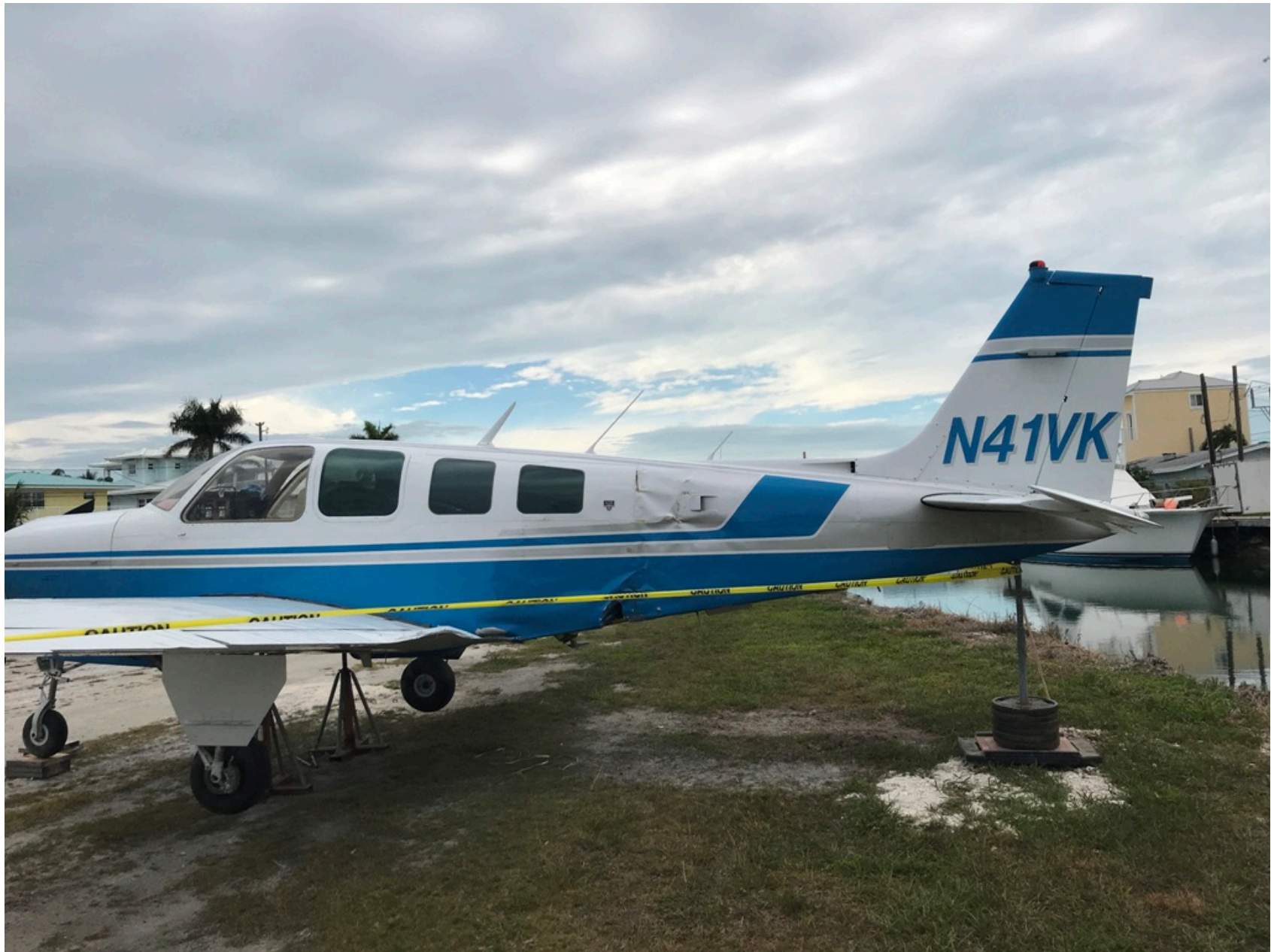
Photo 6 – FAA Digital Photograph. Left Side View Taken After Recovery Depicting the Position of the Elevator Primary Flight Control Surface with the Gust Control Lock Installed.
