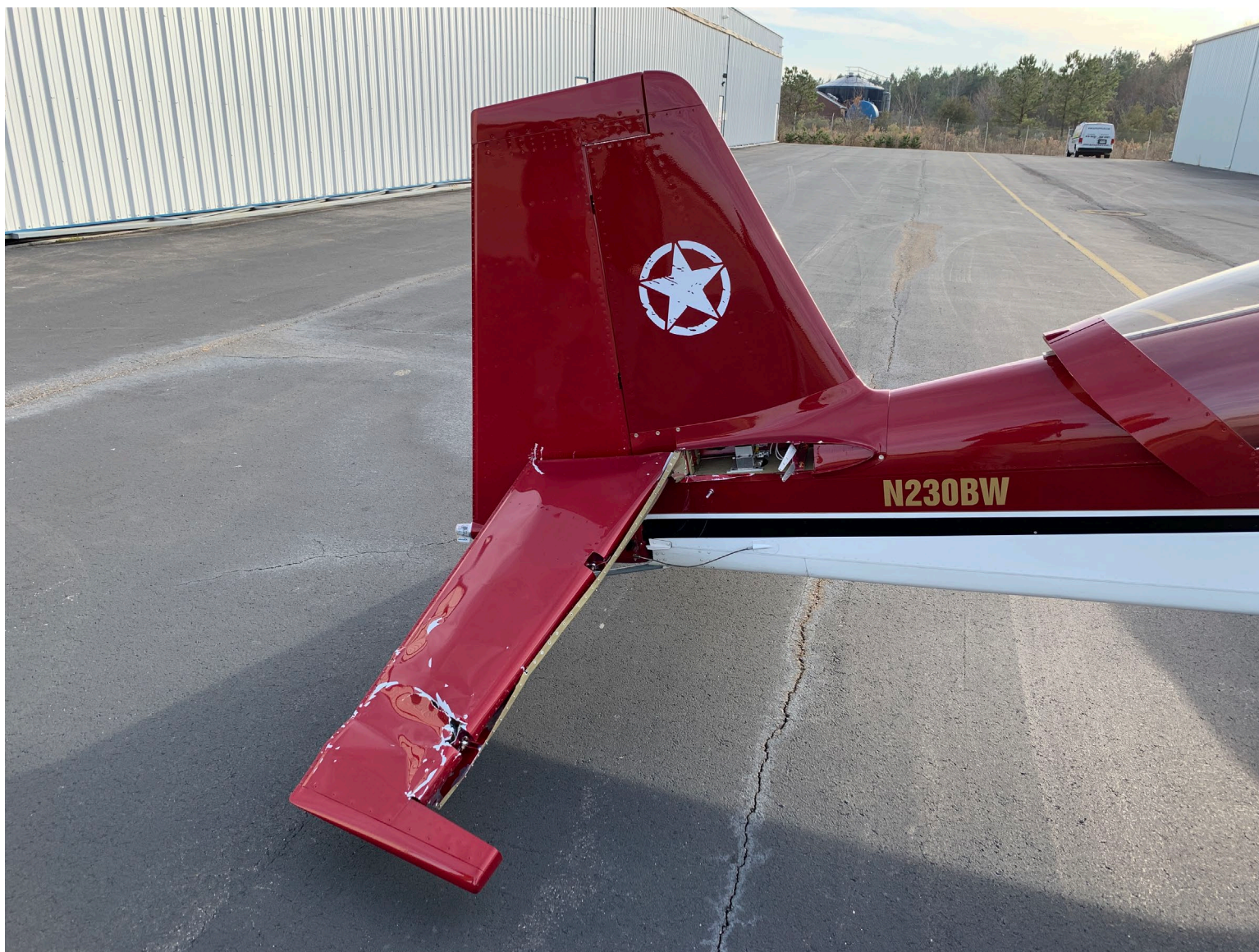
Photo 1 – View of right side tail damage. Right stabilizer missing. Right elevator bent down and damaged. (Courtesy of Owner)
