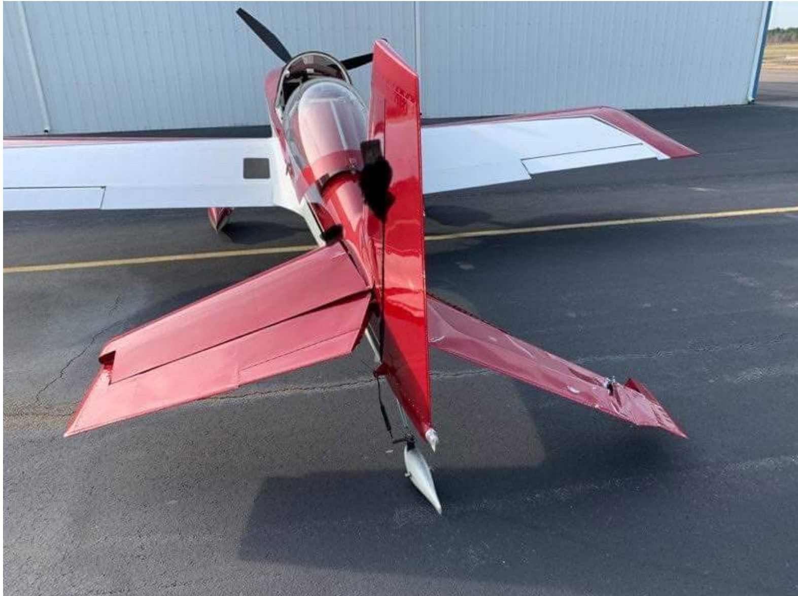
Photo 3 – View of empennage looking forward. Both left and right sides bent down. Right side missing stabilizer. (Courtesy of Owner)
