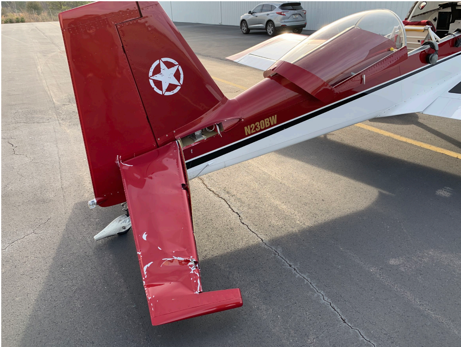
Photo 2 – Close up view of right elevator damage. Note the stabilizer is missing and entire structure is bent down. (Courtesy of Owner)
