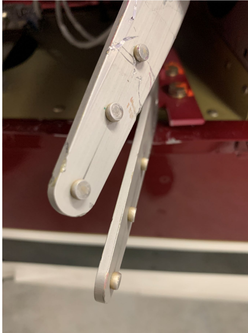
Photo 5 – Photo of forward spar inboard attachment straps/rivets. Note they are bent down and aft. (Courtesy of Owner)
