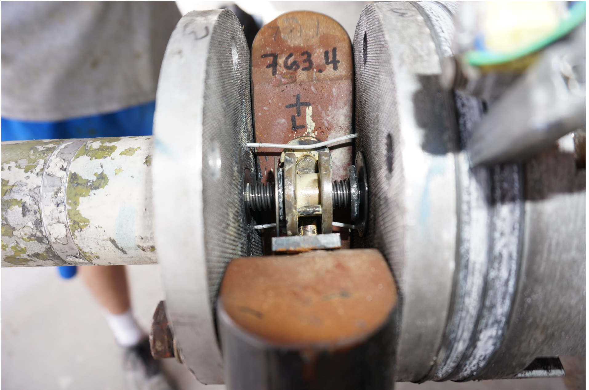
Photo 14 - Propeller Pitch Spool in Approximately Mid-Range Pitch Position
