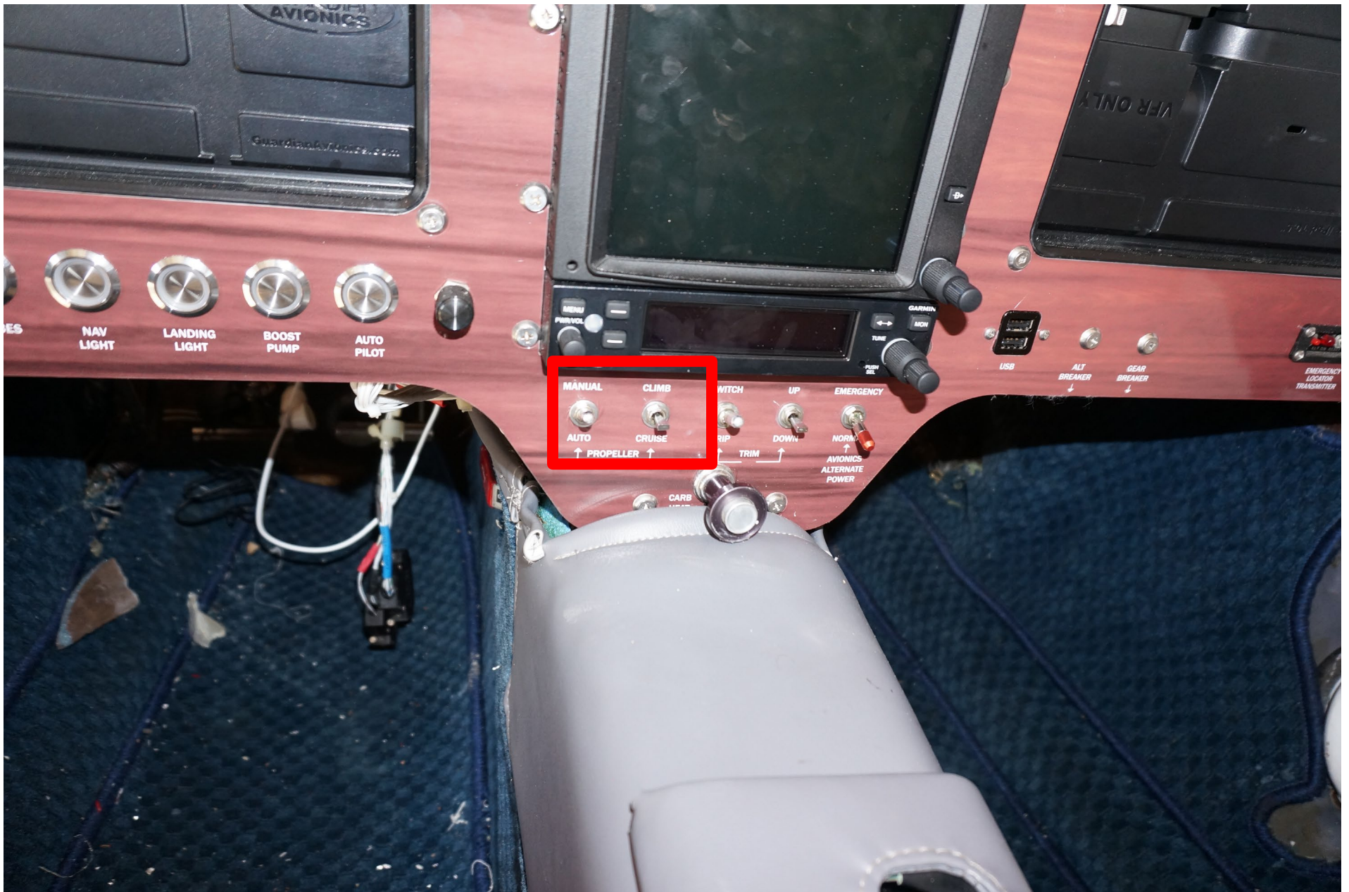
Photo 11 – Propeller Control Switches
