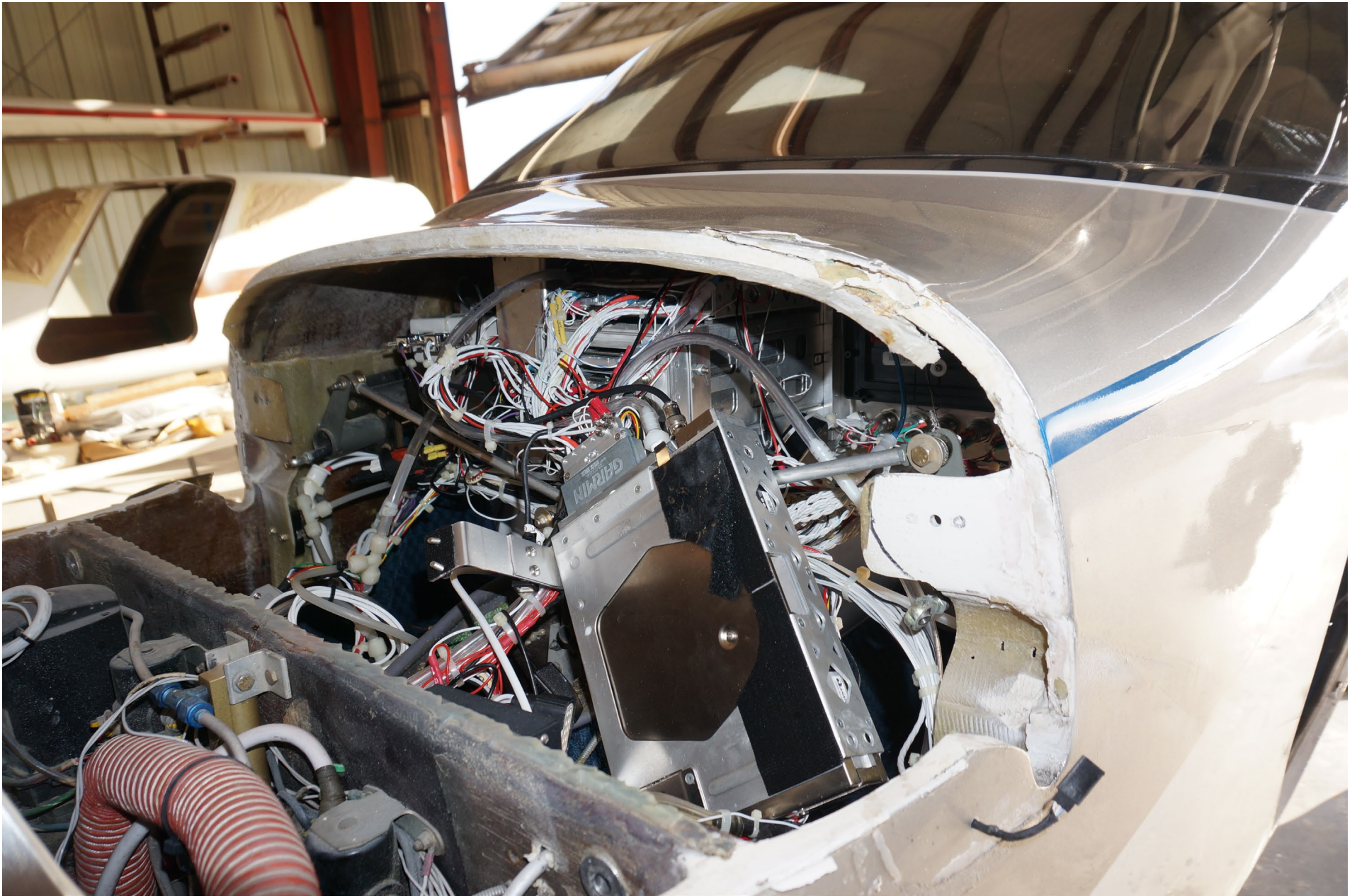
Photo 10 – Upper Fuselage Damage Forward of Windshield
