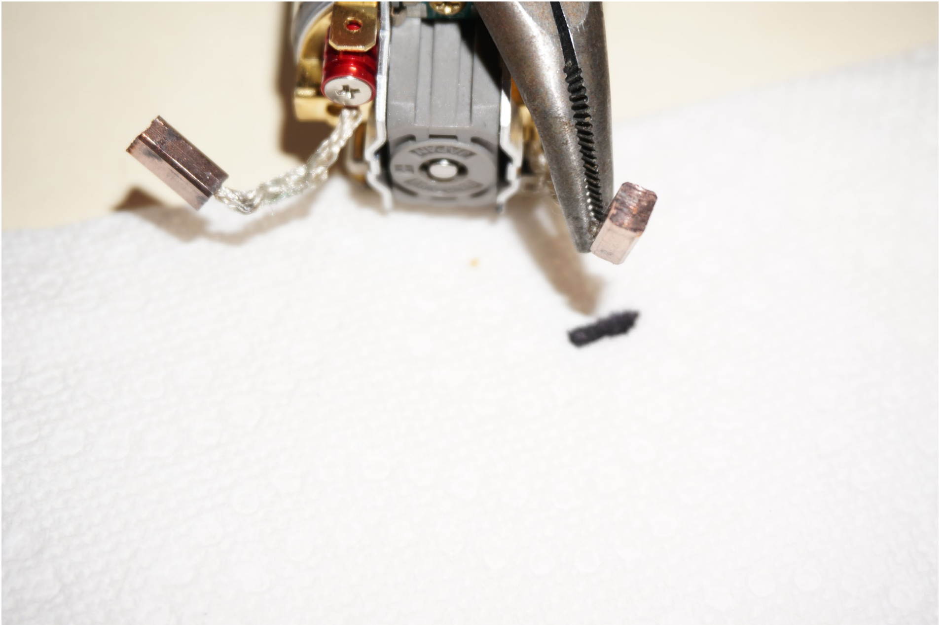
Photo 1 – Electric Motor Carbon Brush (-)
