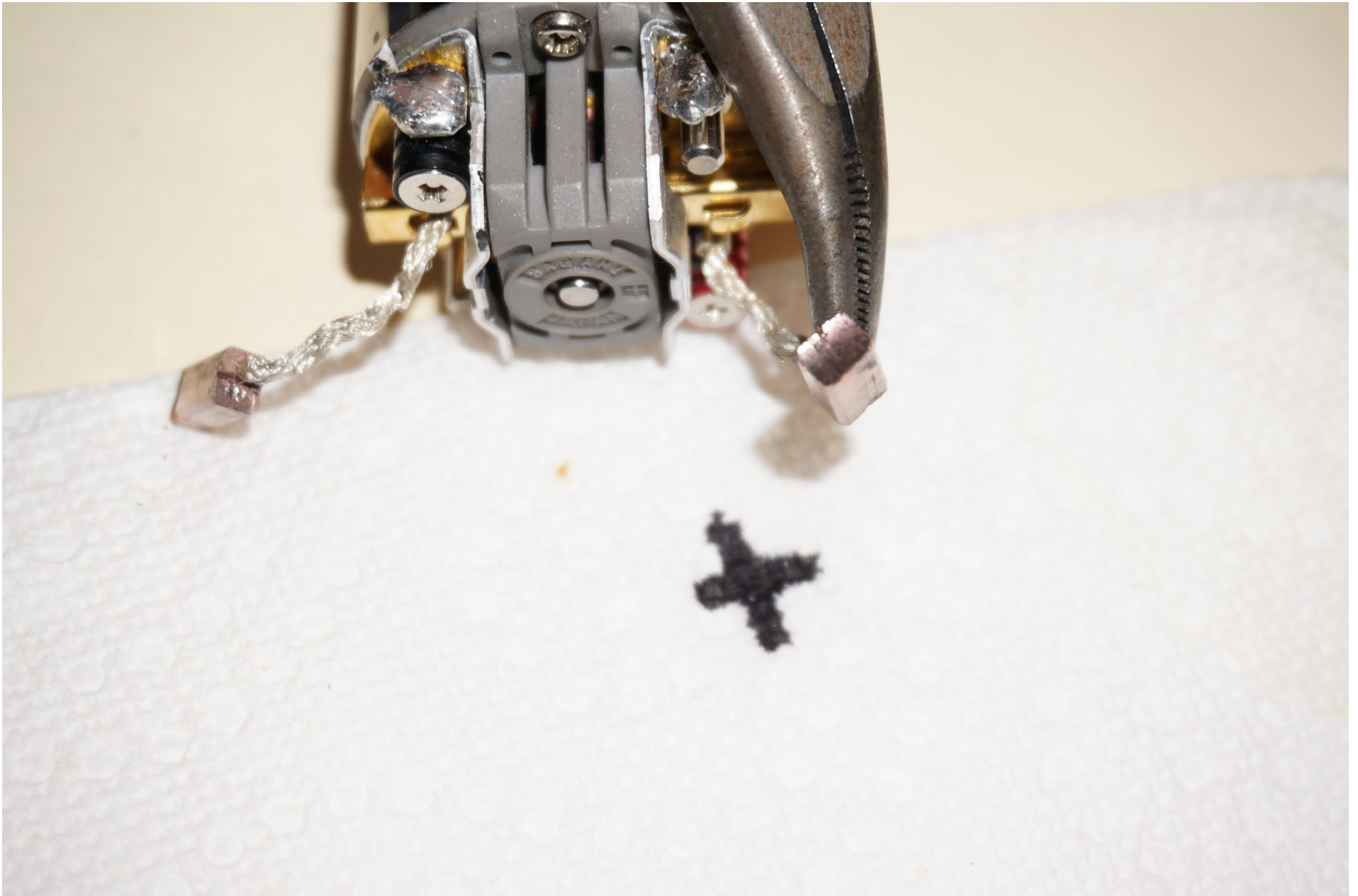
Photo 2 – Electric Motor Carbon Brush (+)
