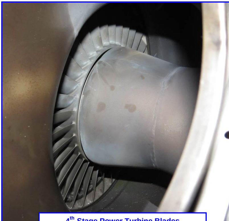
4 th -Stage Power Turbine Blades
