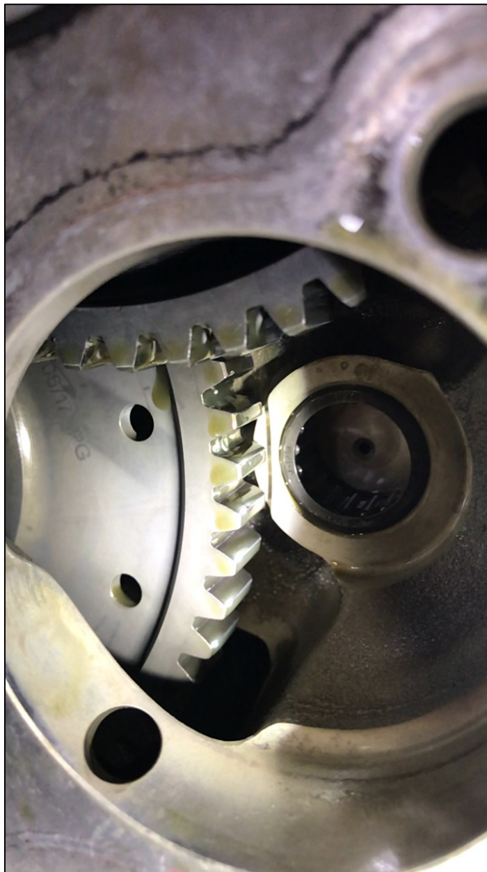
Photo 2: Closer view of the camshaft gear (item #4). The condition of the gear was unremarkable.
