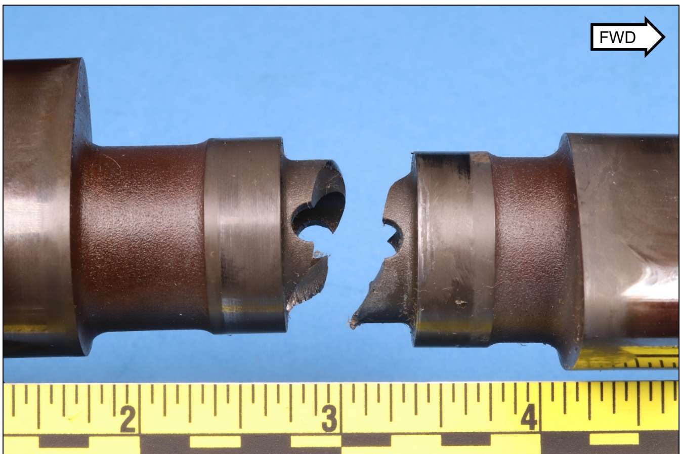
Figure 2. Side view of the camshaft fracture.
