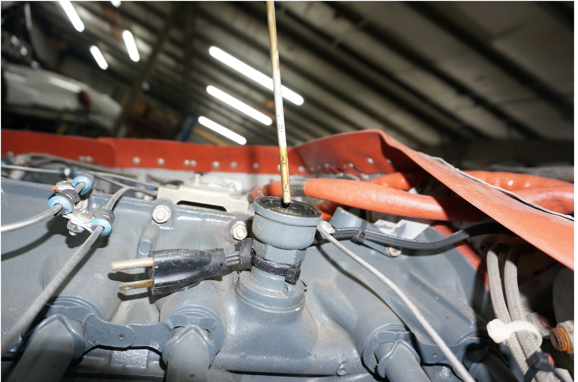
Photo 12 – Oil Level Gauge (Dipstick)
