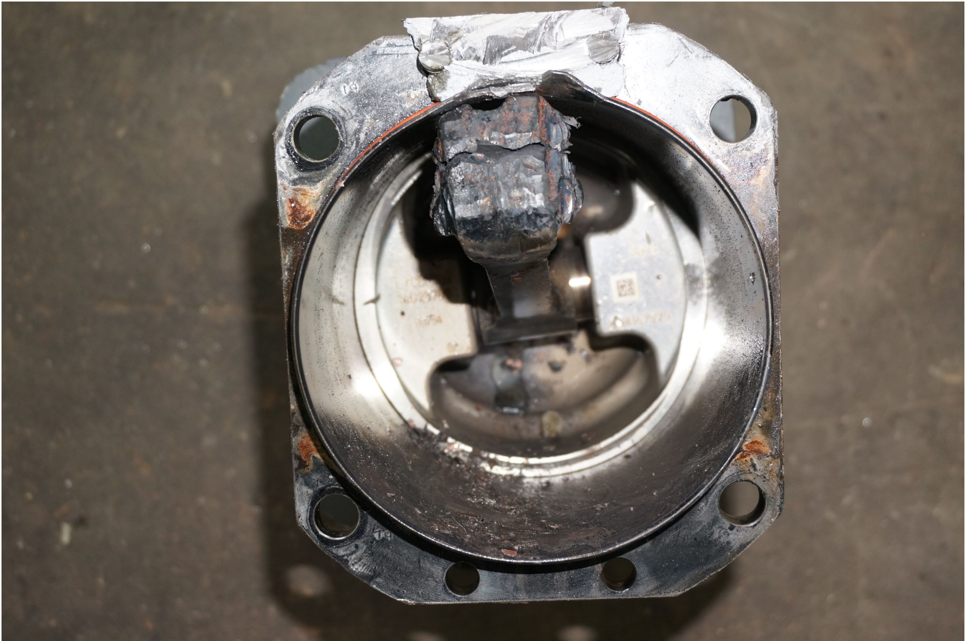
Photo 16 – Remains of No.4 Connecting Rod
