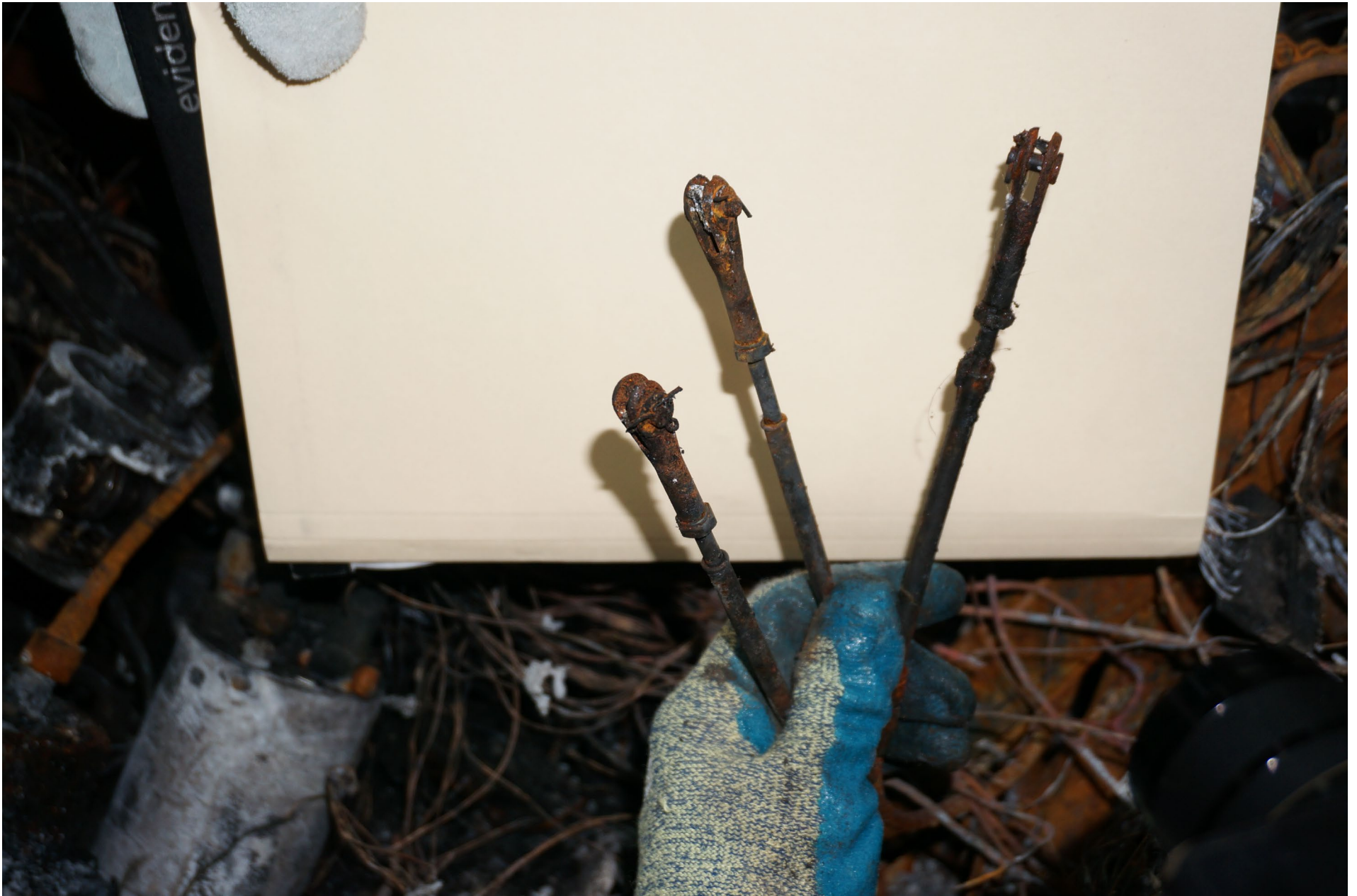
Photo 10 – Throttle, Propeller, and Mixture Control Cables
