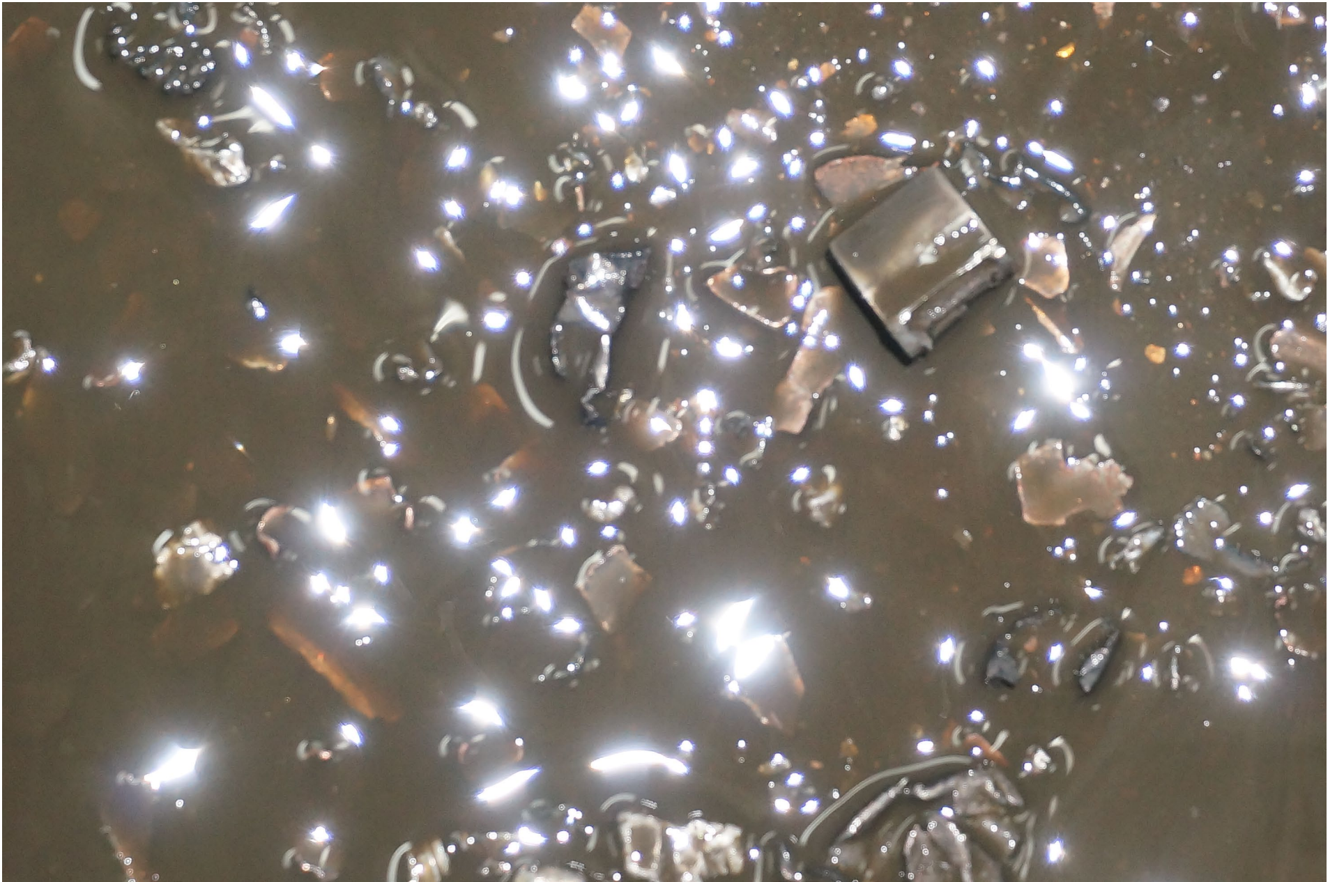
Photo 20 – Contents of Engine Oil Sump
