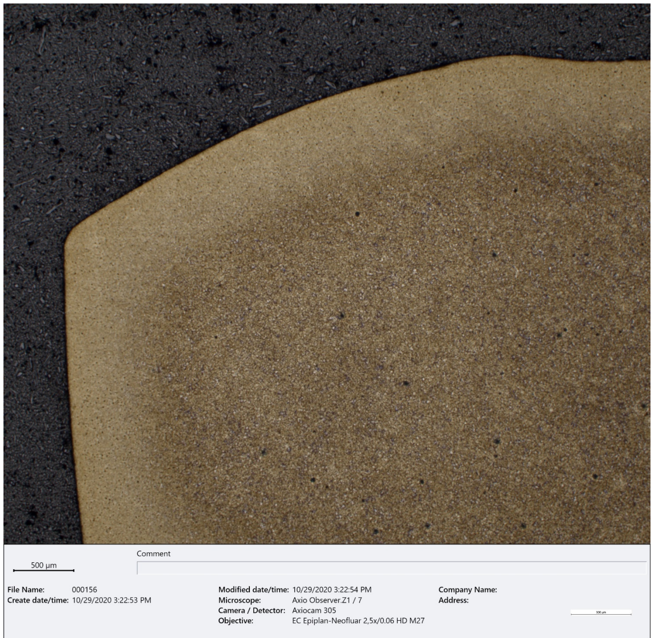
Figure 34 – BF optical micrograph of the surface corner of the cross sectioned fractured gear tooth, showing a different etching response from the surface and core regions (~25X, etched 2% Nital).
