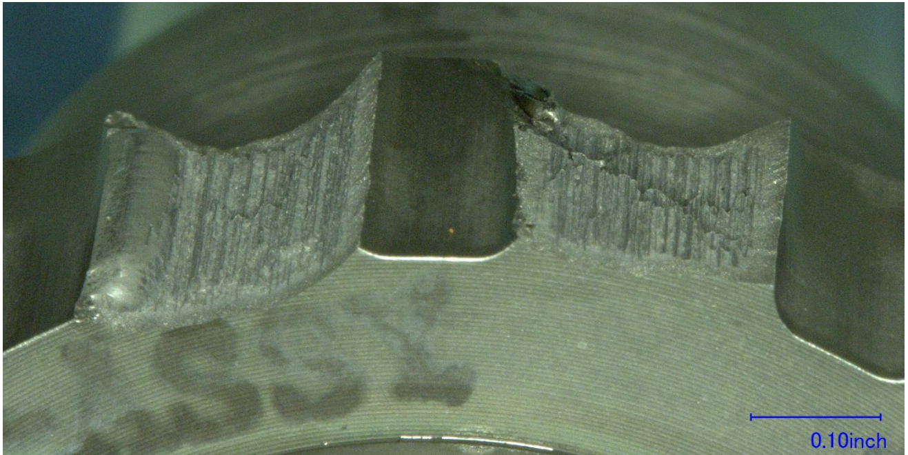
Figure 18 – Angled view of the fractured gear teeth from the drive gear.
