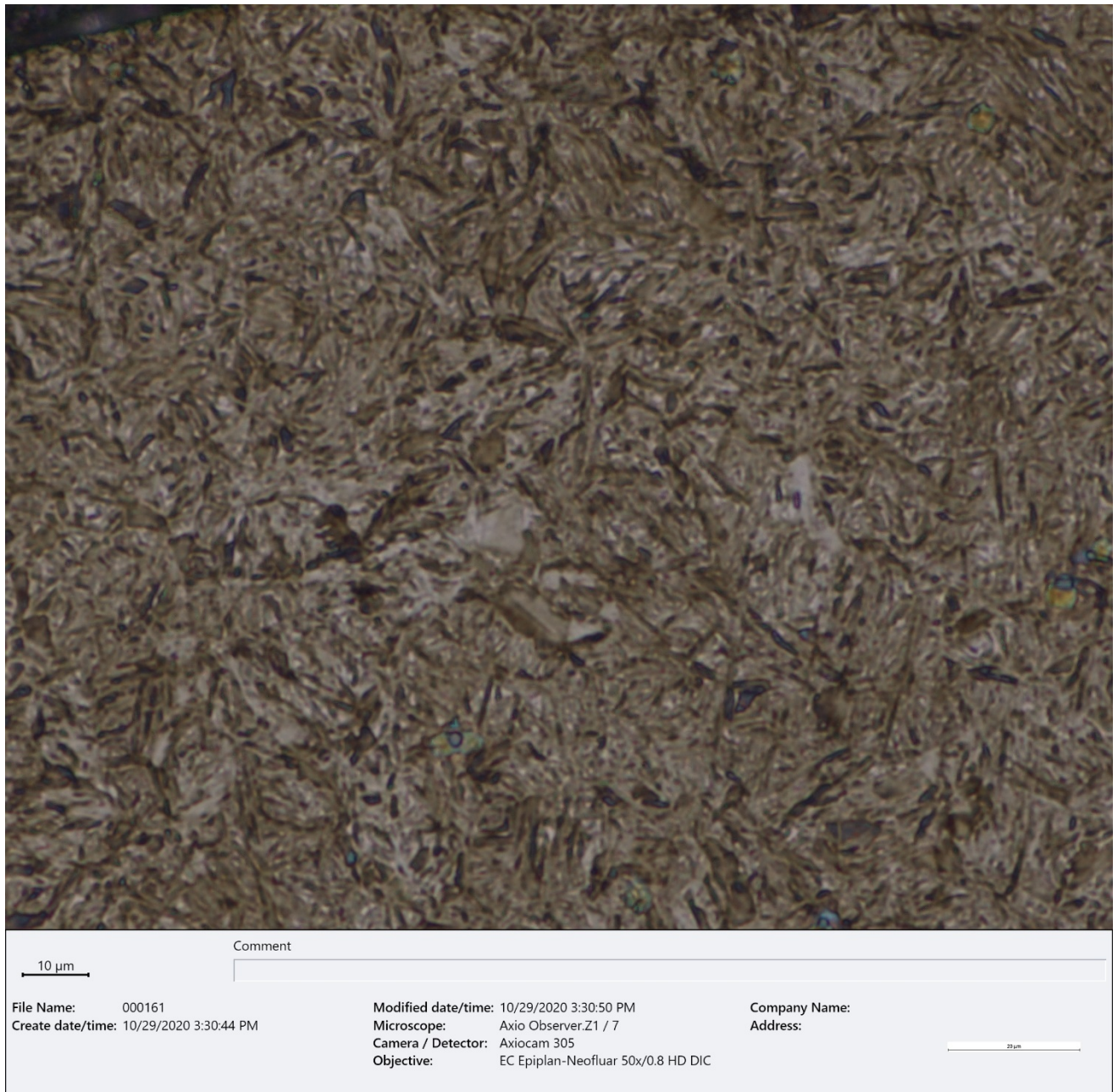
Figure 36 – BF optical micrograph of the surface microstructure of cross sectioned fractured gear tooth (~1000X, etched 2% Nital).
