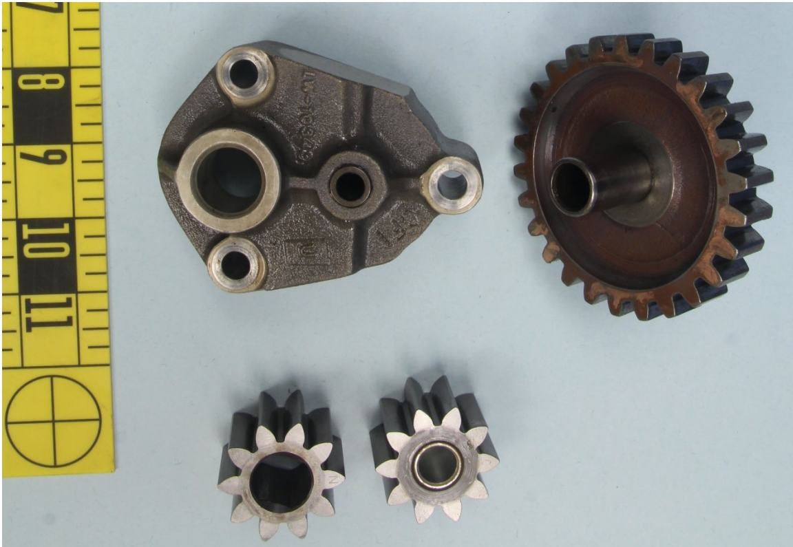
Figure 1 – The oil pump case half, impellers, and large gear, as received.
