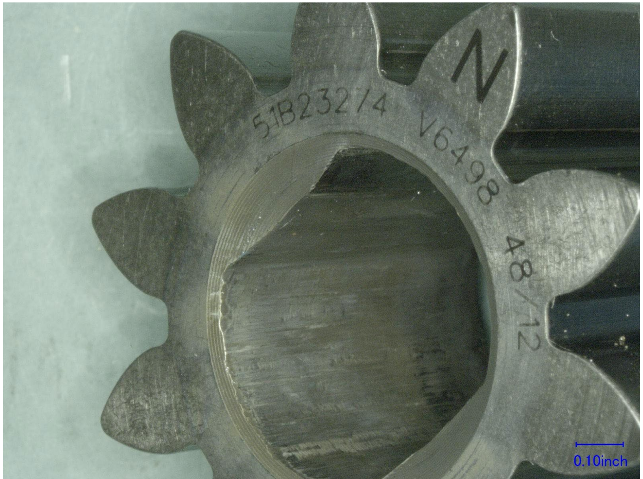
Figure 11 – Angled view of the marked face, teeth, and internal cavity of the slotted impeller gear.
