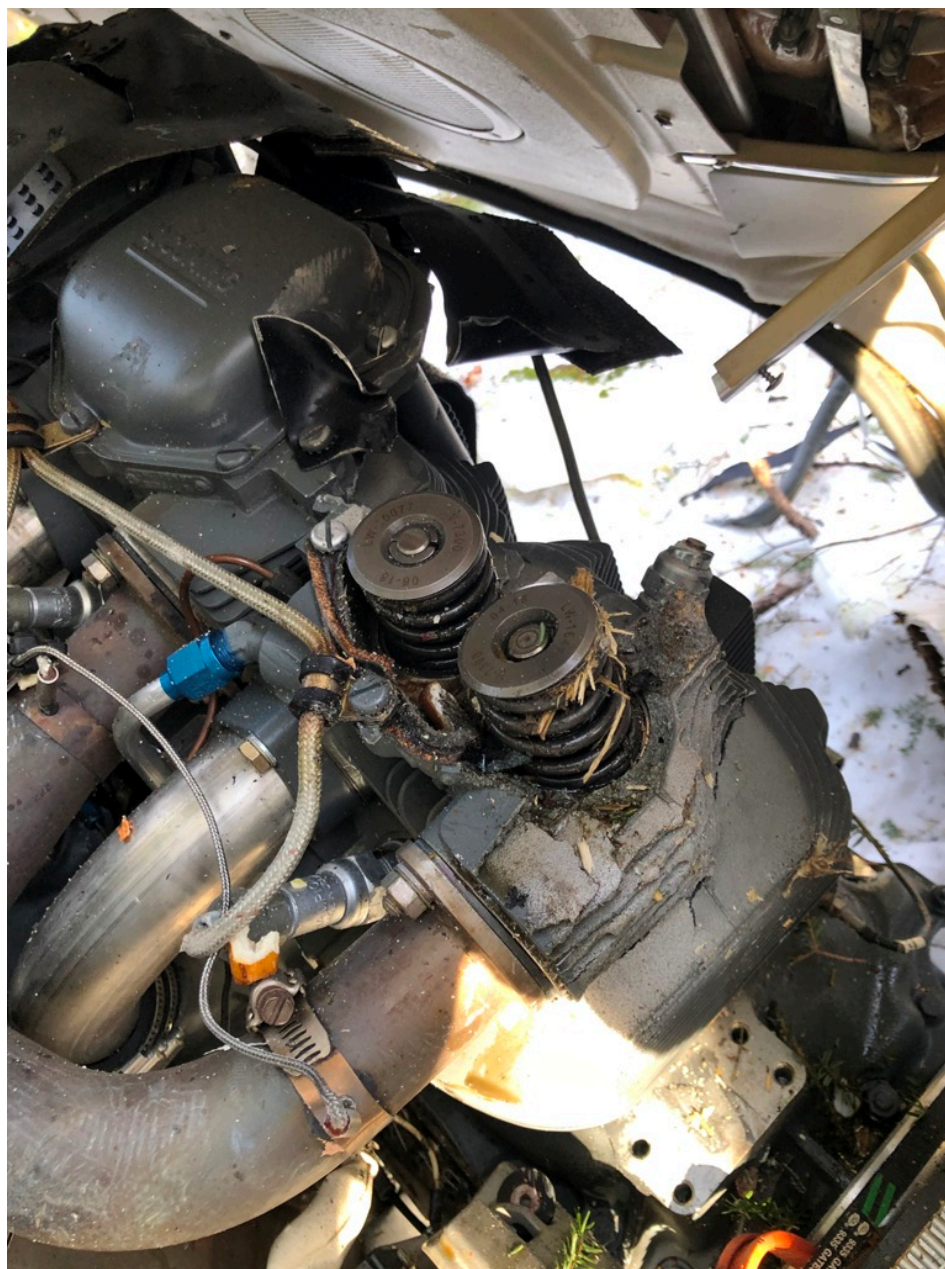
Photo 6 – Engine Impact Damage (FAA Photo)
