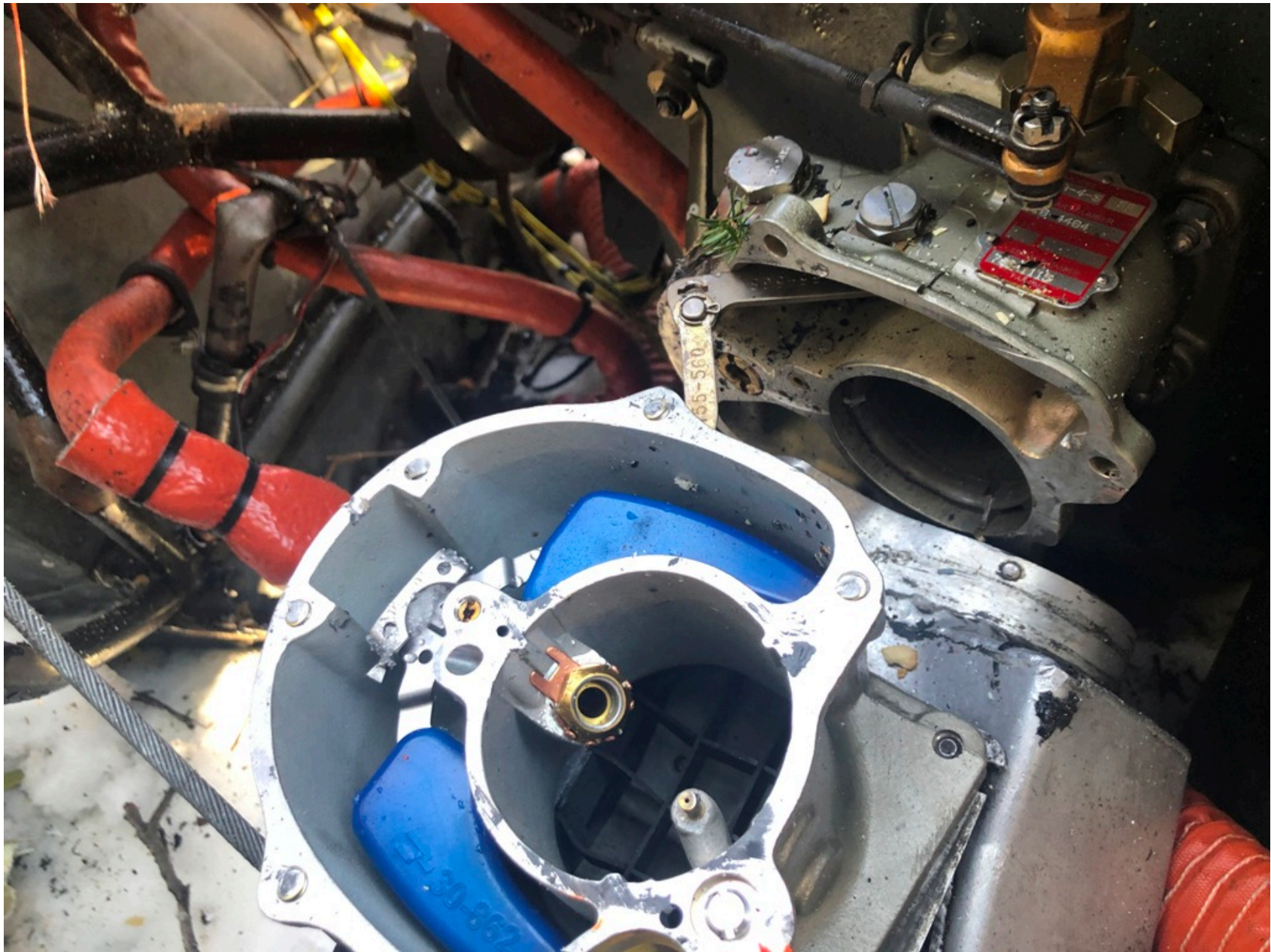
Photo 7 – Carburetor Impact Damage (FAA Photo)
