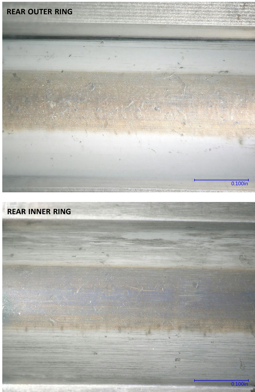
Figure 9: Digital microscope images of the races on the outer (top) and inner (bottom) rings of the rear support bearing.
