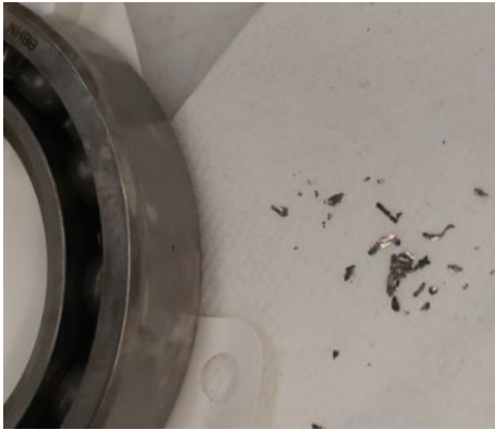
Photo 6- Particles collected from the forward support bearing.
