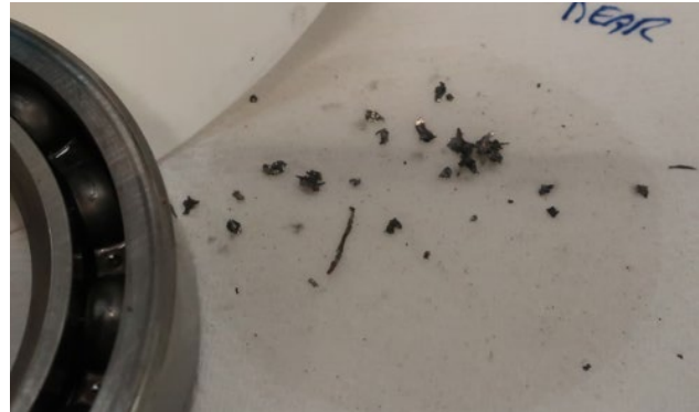
Photo 7 - Particles collected from the rear support bearing.
